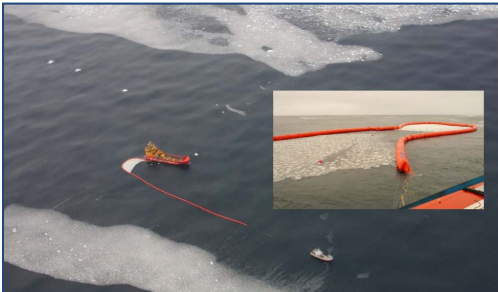
Figure 4-1 Testing Norlense 1200 containment boom in combination with weir- and heavy oil skimmer from Framo.
