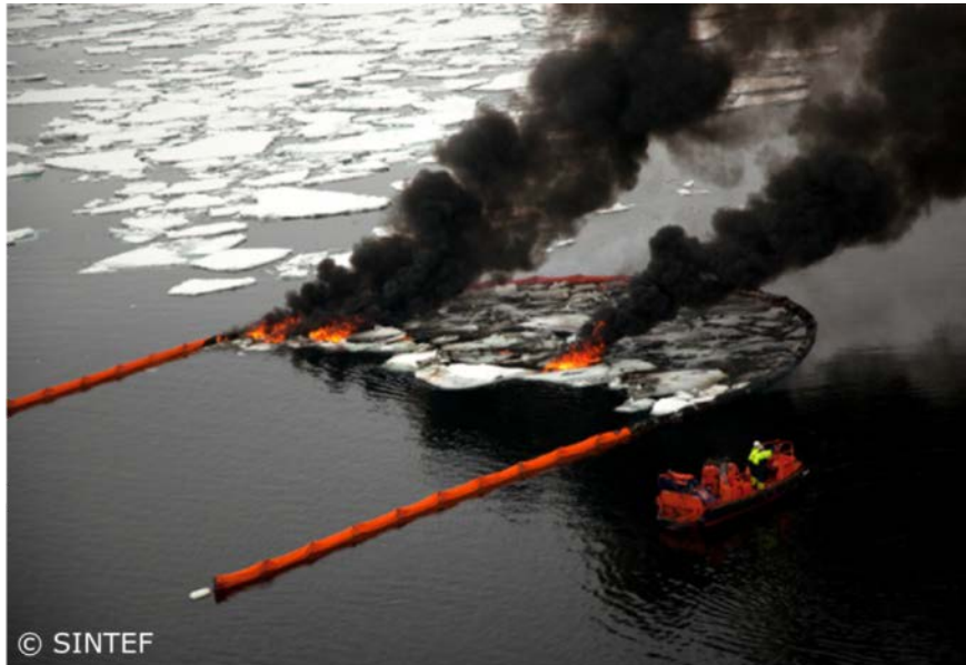
Figure 3-6 In-situ burning test conducted within the JIP Oil in Ice (Copyright: SINTEF).
