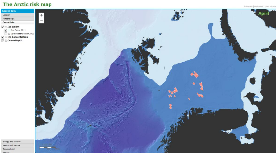
Figure 6-3 Example – average extension of sea ice (> 10% ice concentration) in April 2011, from DNV GL’s Arctic Risk Map.
