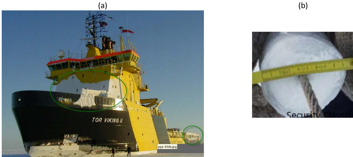
Figure 8-4 Examples - a) snow accumulated on vertical surfaces, b) snow accreted on wire
