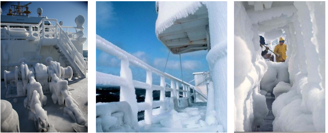
Figure 8-6 Examples – effects of marine icing
