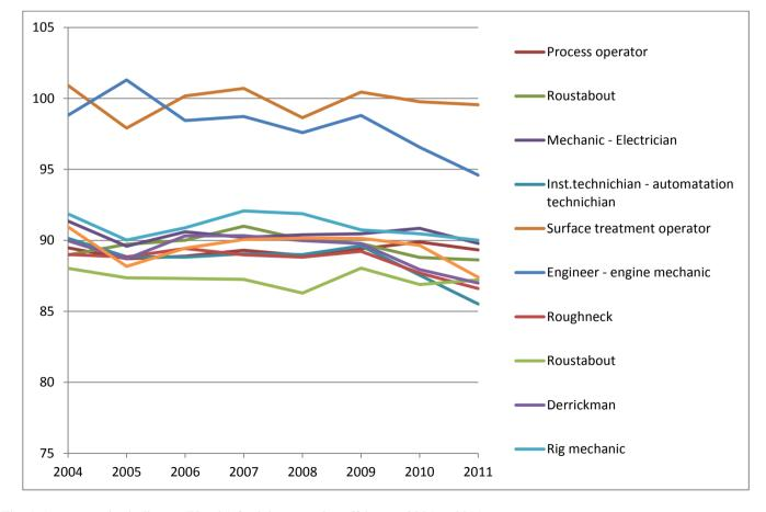
Fig. 1-Average noise indicator (Y-axis) for job categories offshore - 2004 to 2011
