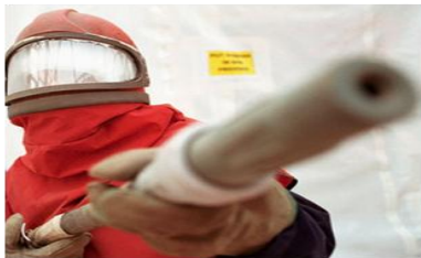
Sand blasting: L_{pA} = 105-115 dB
