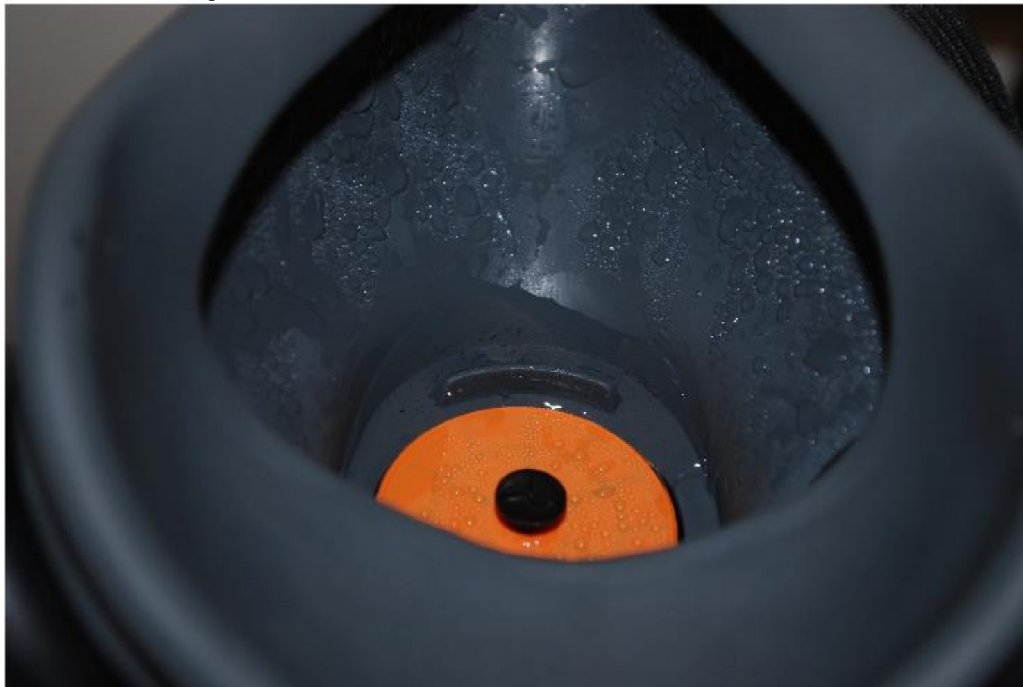
Figure 6.21 The picture is showing condensed water in a SR 90-3 TPE after a test performed in -25\text{ }^{\circ}\text{C} .
