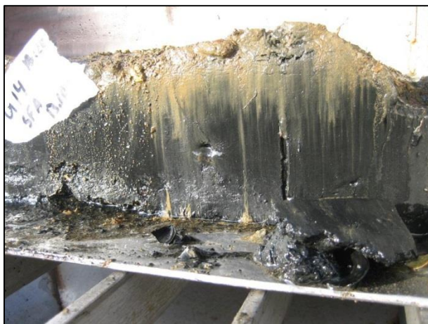
Figure A-3. A cross section of a grab sample with “healthy” oxygenated sediment at the top and black cuttings material below.
