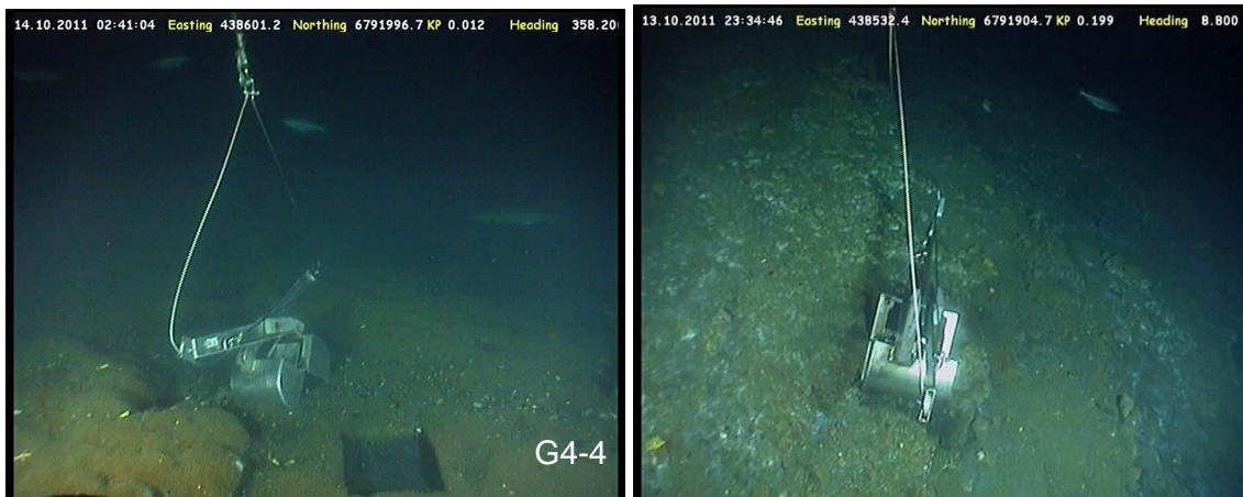
Figure A-2. Grab sampling of drill cuttings surfaces at G4 (left) and G5 (right). The positioning accuracy and ROV visual inspection permit grab replicates to be positioned adjacent to each other. Note the slope of the pile at G5.
