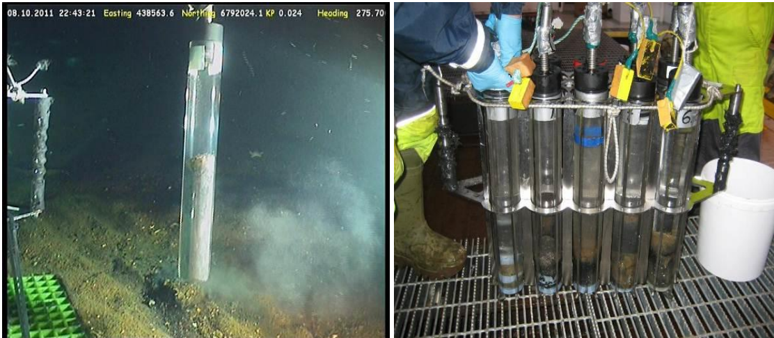
Figure 4-3. A sample corer and corer rack for storing several tubes (DNV 2012).
