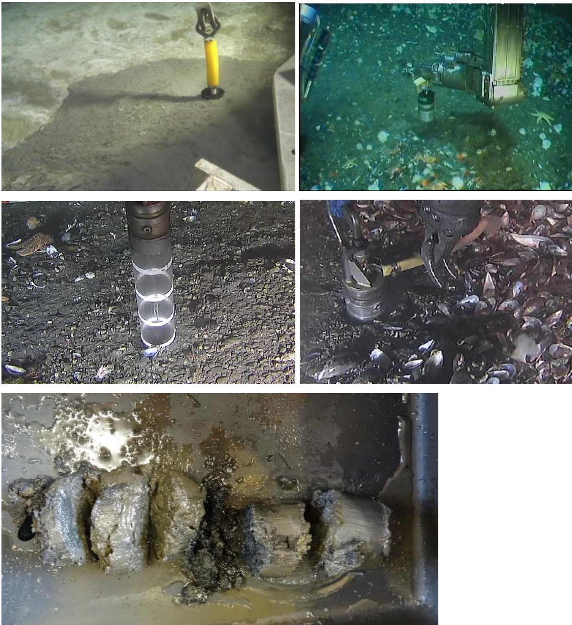
Figure 5-1. Various still photos of ROV operated corer sampling at drill cuttings pile surfaces. Note the variable quality at different locations. A sectioned corer sample is shown in the lowest image.
