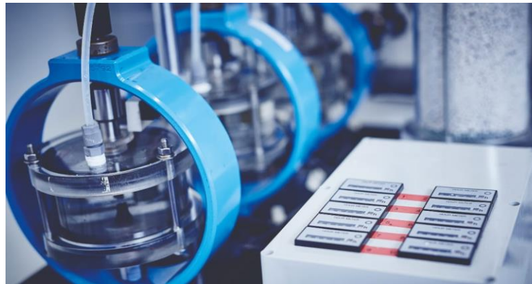
SSC testing using NACE TM0177 Method A specification
