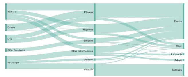
Figure 50 Production flows in the chemical/petrochemicals industry (calculated, based on data from IEA 2017a and other sources)
