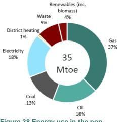
Figure 38 Energy use in the nonmetallic minerals industry, 2016 (based on Eurostat, 2018a)
