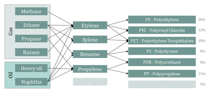
Figure 52 Production flows in the chemical/petrochemicals industry, with the main plastics products on the right (Endrava, based on a wide range of sources). Note: there are too many products for all to be presented in this figure, hence the use of "..." in the light-green boxes at the bottom
