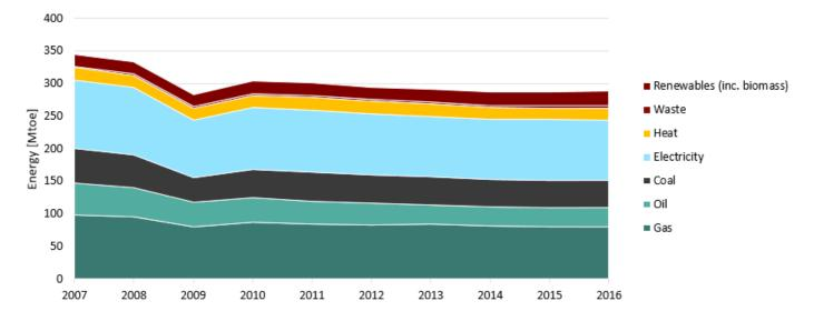
Figure 29 Use of energy in industry in Europe (based on Eurostat, 2018a, non-energy use is not included)
