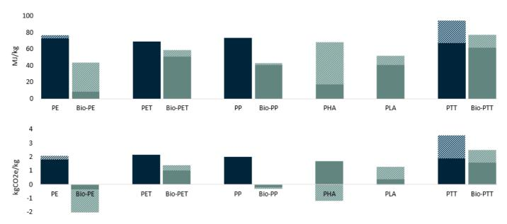
Figure 93 Use of fossil energy (up), and carbon footprint (down) for the production of various types of plastics (based on Shen et al. 2012, Chen et al. 2012)
