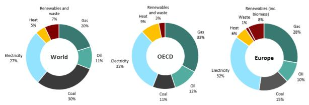
Figure 11 Energy sources to the industry in the world, OECD and Europe (based on IEA 2017 and Eurostat 2018a), for heating, lighting, electrical processes and cooling
