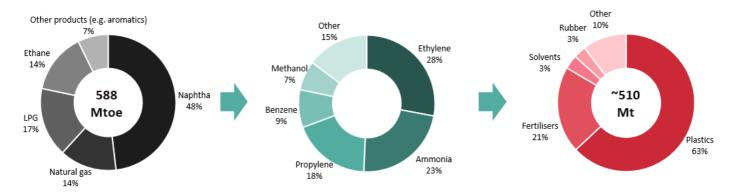
Figure 15 Production flows in the chemical/petrochemicals industry in the world (calculated, based on data from IEA 2017 and other sources)
