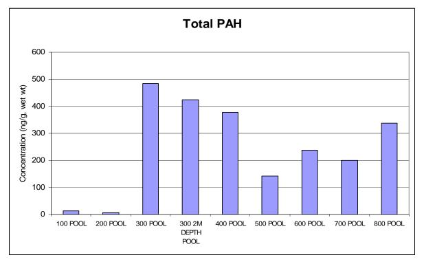
Figure 1. Total PAH Concentrations (ng/g,wet wt) in the Replicate Mussel Samples
