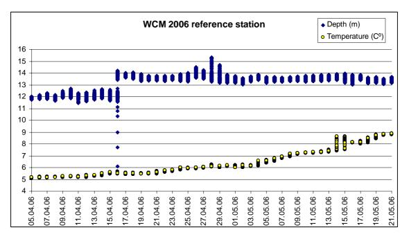
Figure X. Water temperature and measuring depth at WCM 2006 reference station. Note change in depth at the 16<sup>th</sup> of April. Measurements at 10 minute interval.
