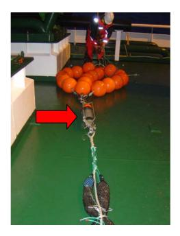
Figure 6. Current instrumentation was fitted by "in line" mounting between the mussels and the submerged flotation.
