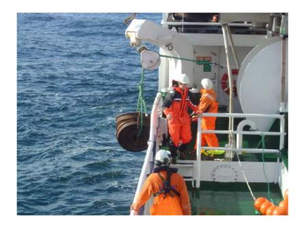
Figure 4. Launching of bottom mooring weight
