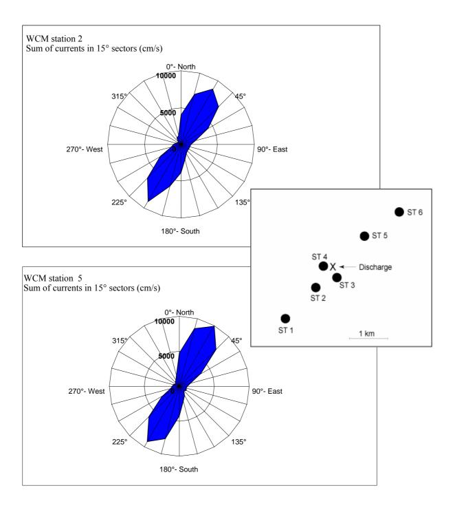
Figure 4. Sum of current measurements (in 15° sectors) at the two stations off Ekofisk. Positions of cages shown for comparison.
