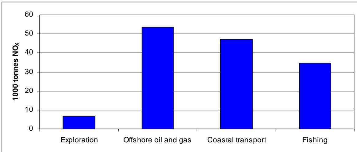
**Figure 6** Emission of NOx. Exploration, total offshore oil and gas industry, marine coastal transportation and fishing [13]. Numbers for exploration are from Table 7. Total offshore oil and gas are from Table 8. All emissions are 1997 numbers.
