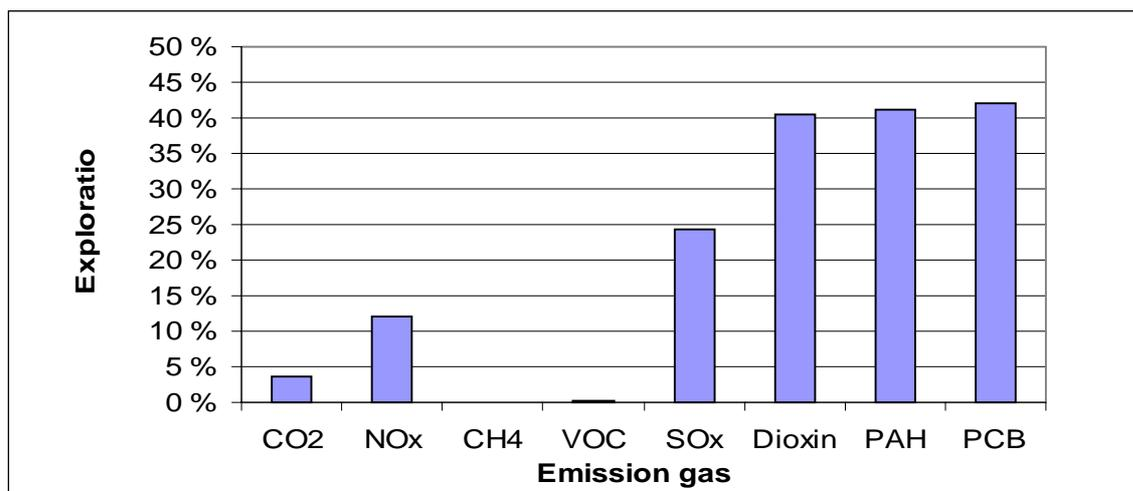
**Figure 4** Exploration activity's contribution to emissions to air from the offshore oil and gas industry. All numbers are from 1998. The differences in the percentages between dioxin, PAH and PCB are due to rounding.
