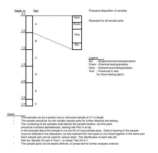
Figure A2.1. Proposed plan for sectioning and disposition of sample parts from deep core samples.
