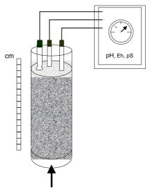
Figure A2.3. Diagram showing the measurements of pH, Eh and sulfide in upper parts of the shallow core.
