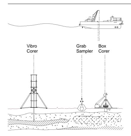
Figure 5. Sampling tools for use in cuttings piles
