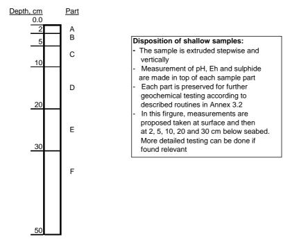
Figure A2.2. Proposed plan for sectioning and disposition of sample parts from shallow core samples.
