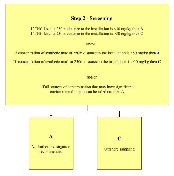
Figure 3. Cuttings piles characterisation process. Step 2: Further evaluation.
