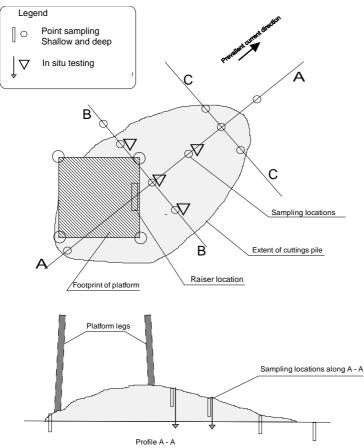
Figure 4. Illustration of a possible sampling scheme for a medium to large cuttings pile.
