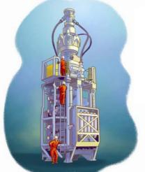
The blow out preventer consists of 3-5 large valves that can be closed so that oil and gas cannot flow to the surface.
