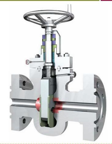
When the stem is operated to the upper end position, it is good practice to turn the hand-wheel back slightly to avoid any damage to the backseat. The manufacturer's instructions should always be followed in this respect.
