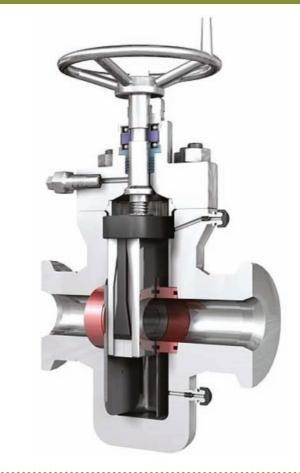
This valve must be tightly screwed in the closed position so that the gate will expand against the seats.
