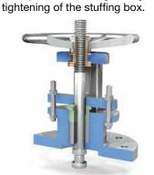
2) Remove the gland nuts. Lift up the pressure gland and the pressure sleeve and bind them securely.
