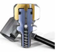
For connections with parallel threads, sealing must be achieved with a separate metal seat or sealing ring. These connections must be locked with a locking pin, or by using the lock-tight fluid specified for the installation.
