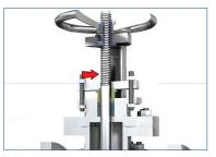
3) Skewed pressure gland Skewed tightening of the pressure gland.
