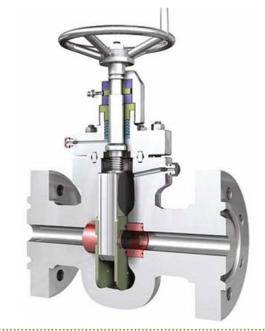
This valve must not be tightly screwed to a closed position. This is because the gate parts should be able to 'float'.
