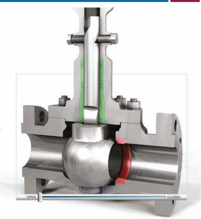
This valve must be tightly screwed to the closed position. This is because the ball must be pressed tightly against the seat and provide a good seal, especially when the seat is mounted in the upstream direction.
