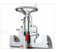
The first thing to do is to loosen the stem cup under the wheel. The stem is now pushed into the backseat position by the system pressure in the valve housing.
