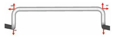
Quick opening and closing of valves can cause pressure pulses caused by positive or negative acceleration of the fluid. The pressure pulses may reflect, for example, when they encounter shut-off ends, T-pieces, phase changes in the fluid or large expansions in a cross-section. If several of these reflections meet each other, they could reinforce each other and produce a pressure which is several times greater than the original system pressure. Such a pulse can move with sonic velocity.
