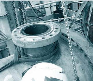
When pressure is not acting on both sides of the piston, there is a danger that the force of gravity will operate the valve in a depressurized system.
