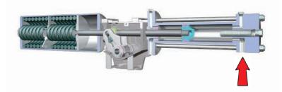
On certain valves that are critical for safety, there is a backup system to ensure that the valve can be opened and closed a certain number of times. For safety-critical maintenance operations, the hydraulic system, including the backup system, must be disconnected and have a drainage point against the actuator. This is done to prevent pressure buildup in the hydraulic system that could cause undesired valve operation.
