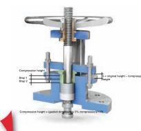
Note! Make sure the pressure gland is horizontal and does not scrape against the stem during compression.
