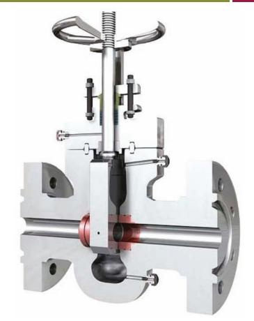
When the valve is closed, it is a good practice to turn the handwheel slightly towards the open position to prevent the gate locking at the bottom of the valve housing. The manufacturer's instructions should always be followed in this respect.
