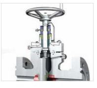
Check the seal by placing a stinger on the lubricating nipple. When the backseat seal has been checked, replacement of the stem gaskets can be carried out.
