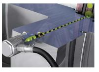
Remove deposits on the ball by rotating it 5-10 degrees back and forth 4-5 times in both the open and closed position. This applies in cases where there is both one and two lubricating nipples into each seat.
