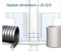
7) To ensure good contact between the stem and the gasket before compression, the gasket dimension must be adjusted within tenths of a millimeter. This is done by rolling the gasket carefully out with a gasket roller.
