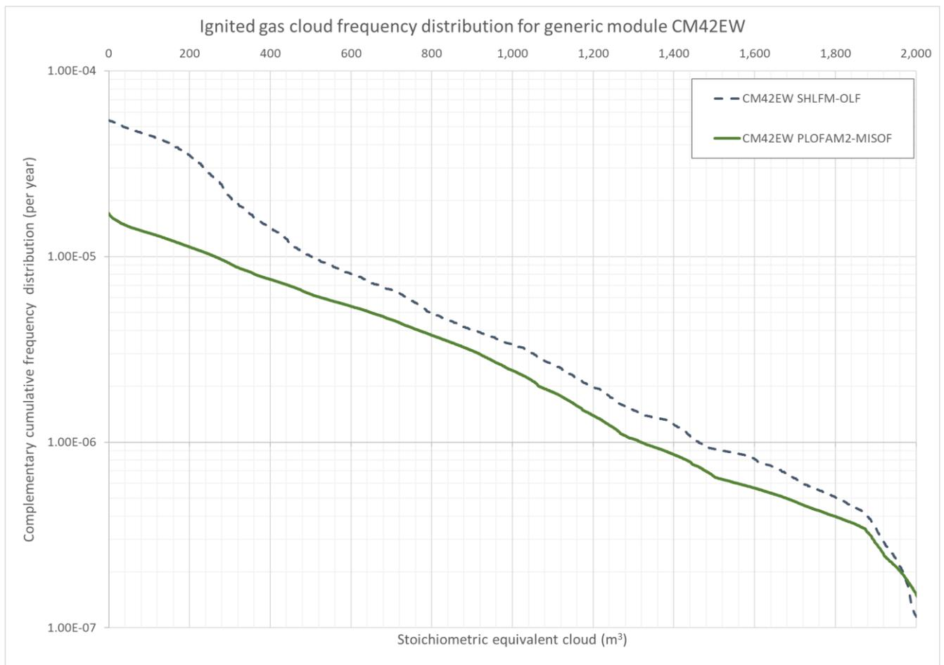
**Figure 4-1: Complementary cumulative frequency distribution for ignited stoichiometric equivalent gas cloud for the generic module CM42EW.**
