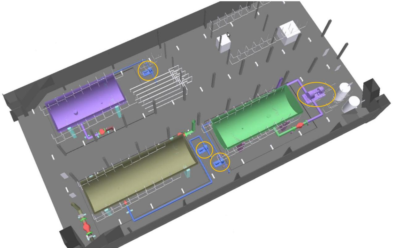
Figure 4-17: CM402EW: Bird's view displaying location of pumps
