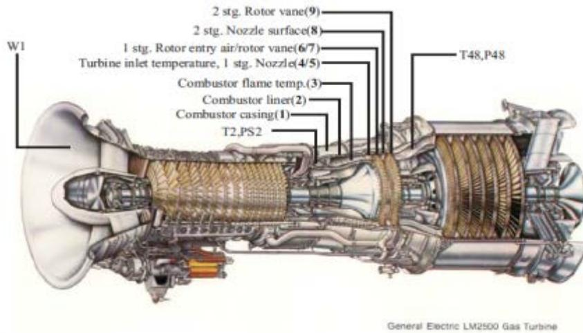
Figure 2.1 - LM 2500 gas turbine
