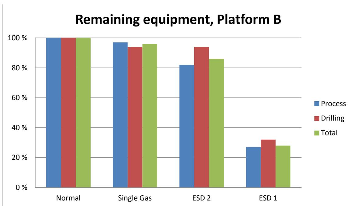
Figure 5.2: Isolation factor F for equipment on Platform B, scaled for Ex protection
