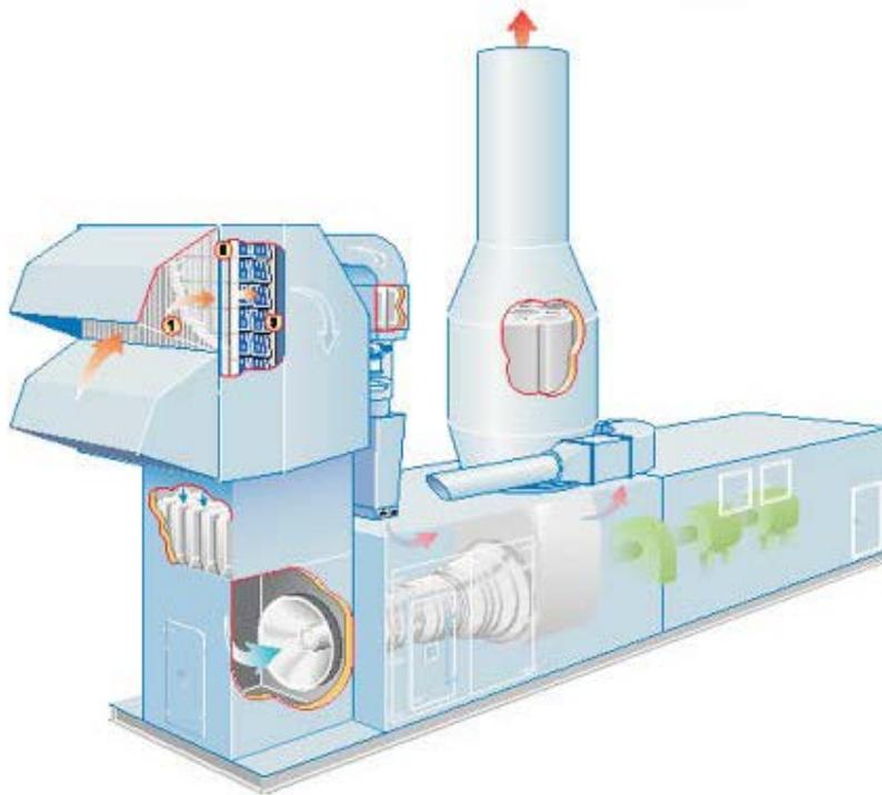
Figure 2.4 - Typical gas turbine air inlet system
