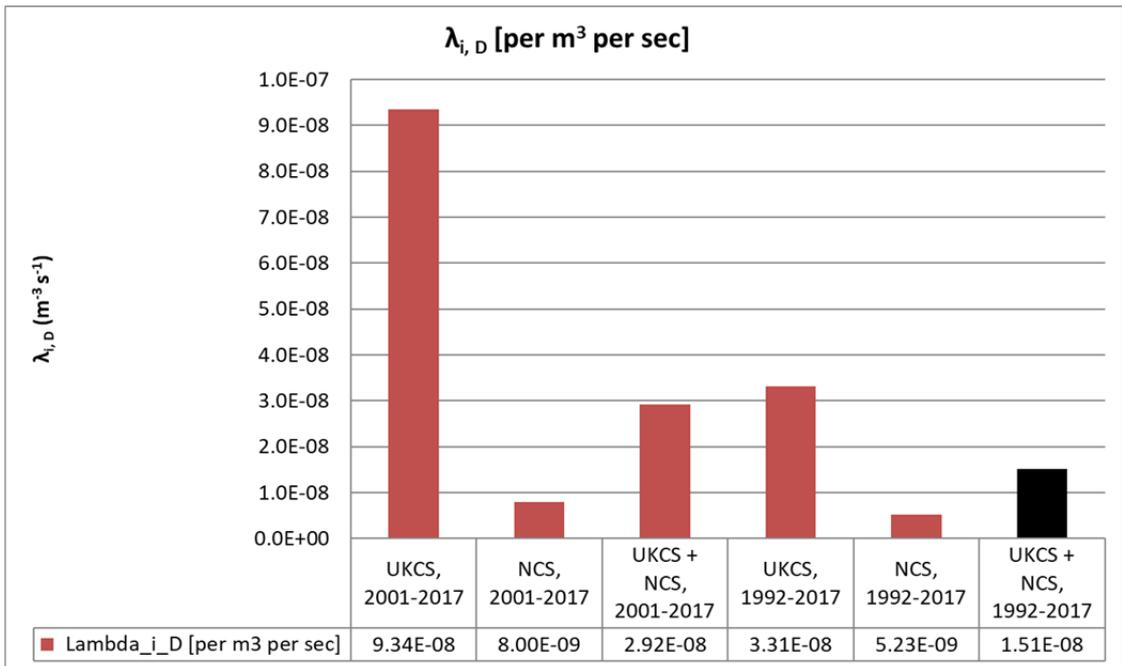
Figure 8.6 - Delayed ignition probabilities for discrete ignition sources. The concluded parameter to be used in the MISOF model is shown in black colour
