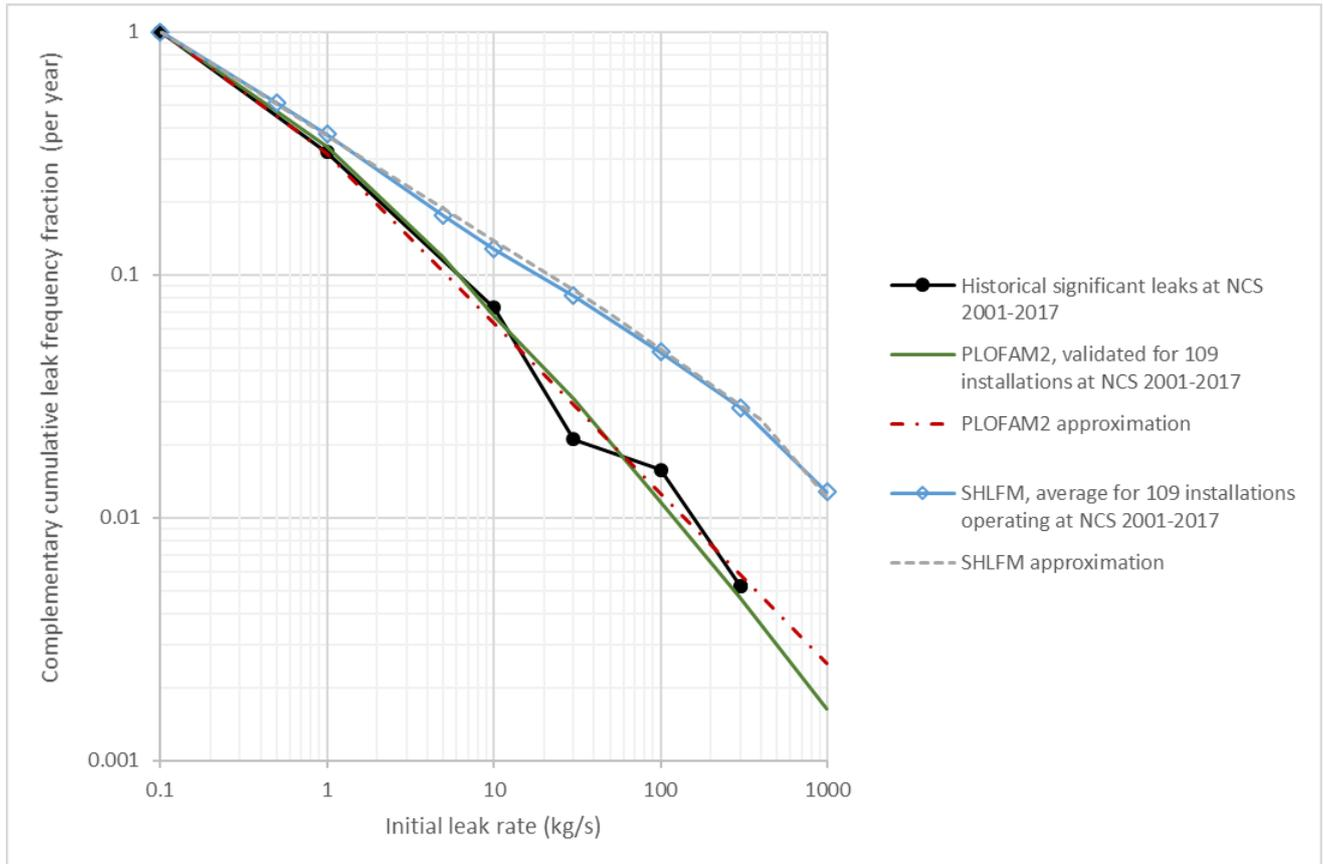
**Figure 3-5: Leak frequency fraction distribution approximations. The PLOFAM approximation applies to significant leaks. The SHLFM approximation applies to both full and limited leaks.**
