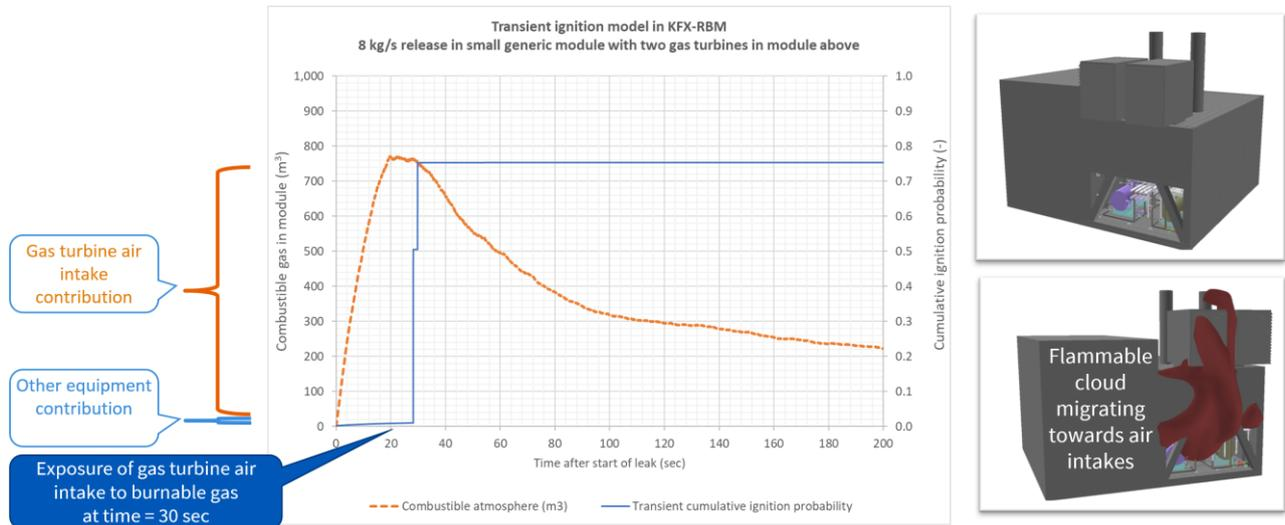
**Figure 4-21: CM42EW: example scenario (8 kg/s) by use of KFX-RBM exposing gas turbine air intake and location of gas turbine air intakes relative to the module (directly above)**
