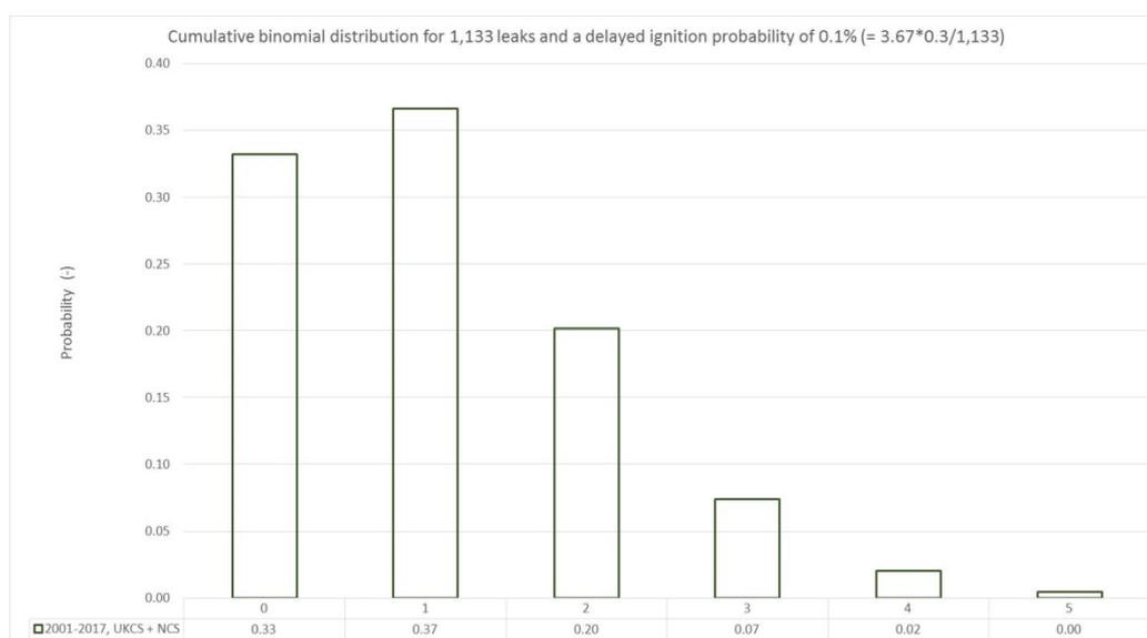
**Figure 11.8 – Binomial distribution for a delayed ignition probability of 0.1% and 1133 leaks occurring at installations located in the UKCS and NCS during the period 1992-2017**
