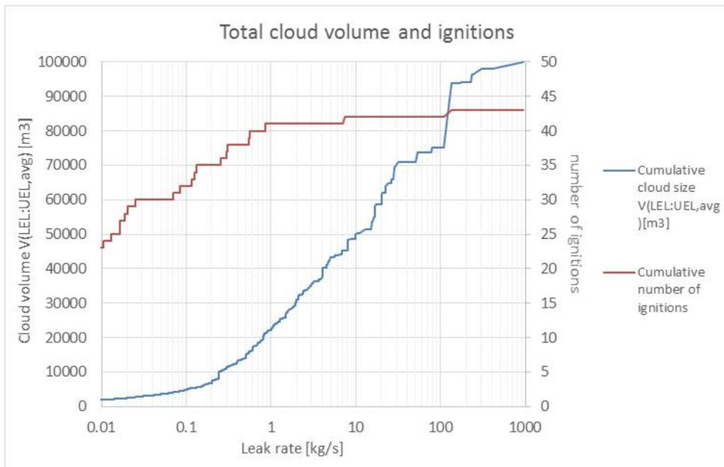
Figure 7.1 – Correlation between exposure to combustible mixtures, leak rate and ignited events extracted from the observed data (NCS and UKCS leaks in the period 1992-2017)
