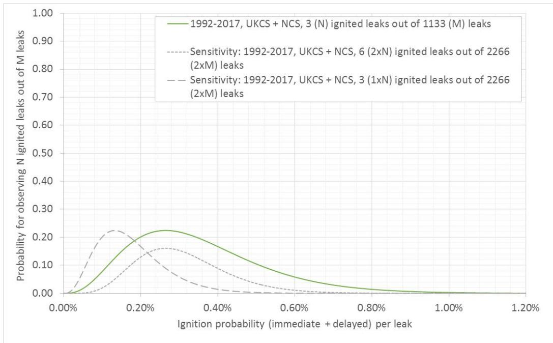
Figure 11.10 – The probability for observing N number of observed ignited leaks out of M leaks as function of  $p$  (estimate of the underlying ignition probability due to immediate and delayed ignition) based on the binomial distribution. The results are shown for the main dataset used for parameterisation and assumed outcomes in the future based on this dataset
