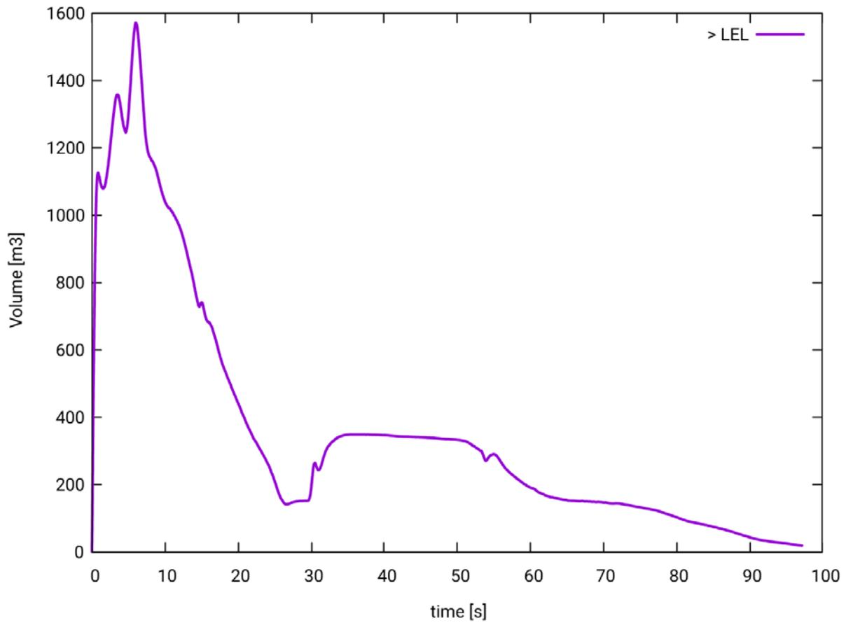
Figure 3.8 - Leak ID 146: Time history for the volume of gas with concentration higher than LFL,  $V_{>LFL,146}(t)$ , estimated by CFD simulation performed with Kamelon FireEx KFX®
