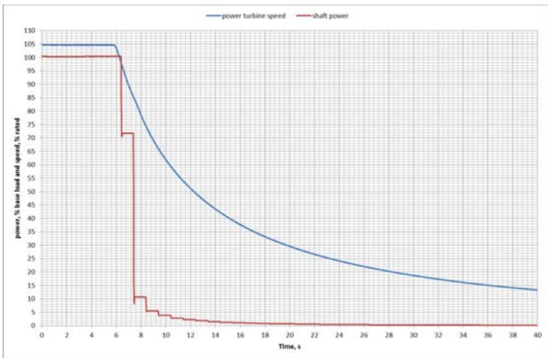
Figure 2.5 - Shaft power and turbine speed during rundown of LM2500
