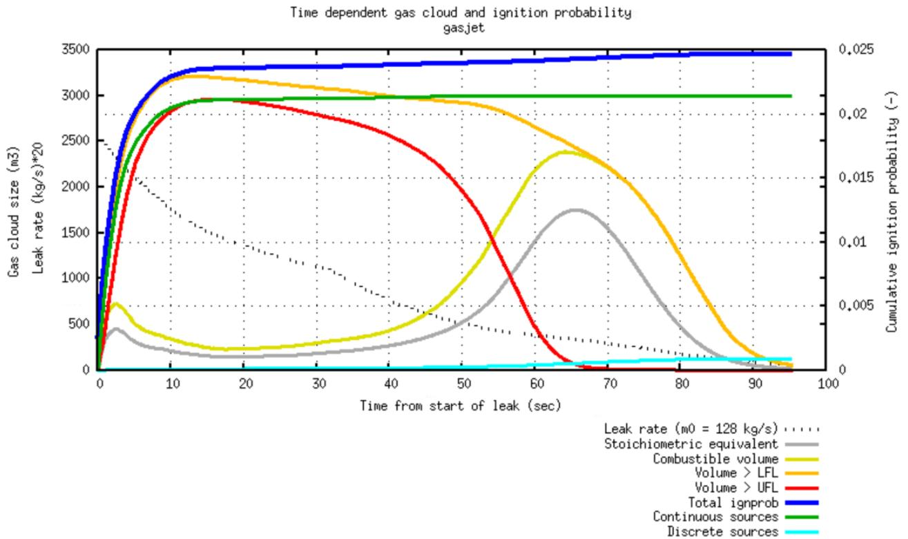
Figure 3-12: Transient result for 128 kg/s gas leak in M43OSV
