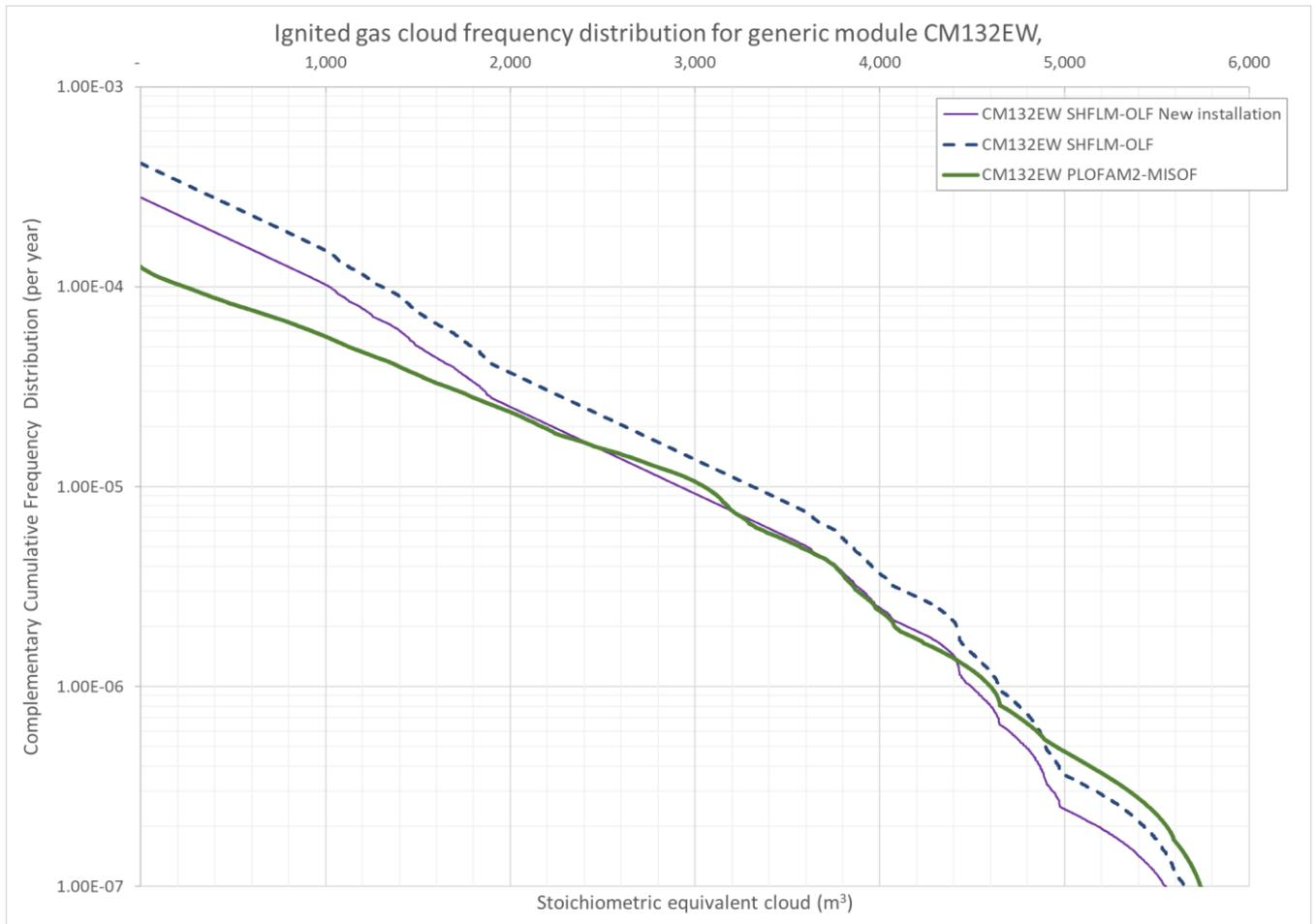
**Figure 4-8: Complementary cumulative frequency distribution for ignited stoichiometric equivalent gas cloud for the generic module CM132EW including sensitivity with OLF model assuming new installation. A correction factor of 0.675 has been used to reflect a new installation (see Table 3-6).**
