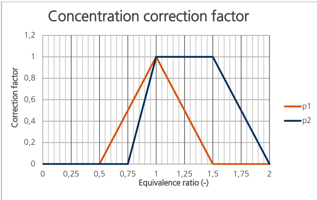
Figure 2.11 – How the correction factor  $f$  can be used to adjust the ignition probabilities  $p_i$  and  $p_j$  in the model
