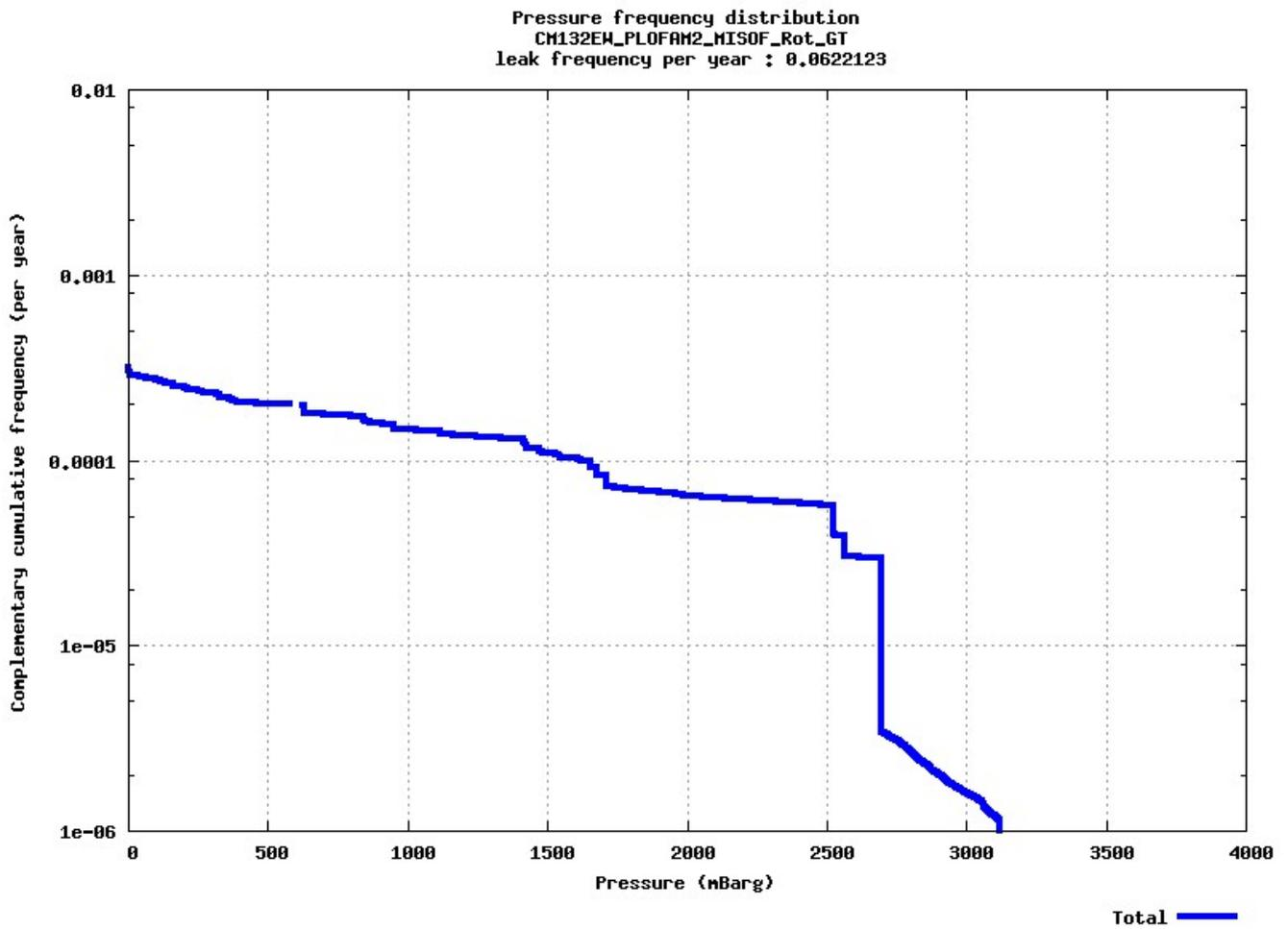
**Figure 4-25: CM132EW PLOFAM-MISOF: Complementary cumulative frequency distribution for dimensioning explosion load corresponding to the ignited gas cloud distribution in Figure 4-23. See Figure 5-2 for the result excluding the two gas turbine air intakes.**
