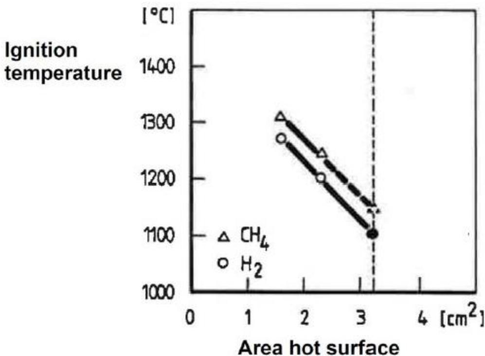
Figure 6.1: Ignition temperature as function of surface area, taken from Appendix B
