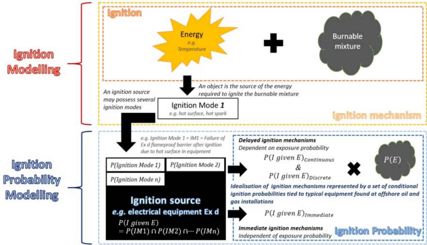
Figure 4.1 – Illustration of the fundamental difference between ignition modelling and ignition probability modelling. MISOF is covering idealised representation of ignition mechanisms by conditional ignition probabilities tied to typical equipment found on offshore oil and gas installations. See Chapter 5 and Chapter 6 for further description of terms and expressions used in this figure
