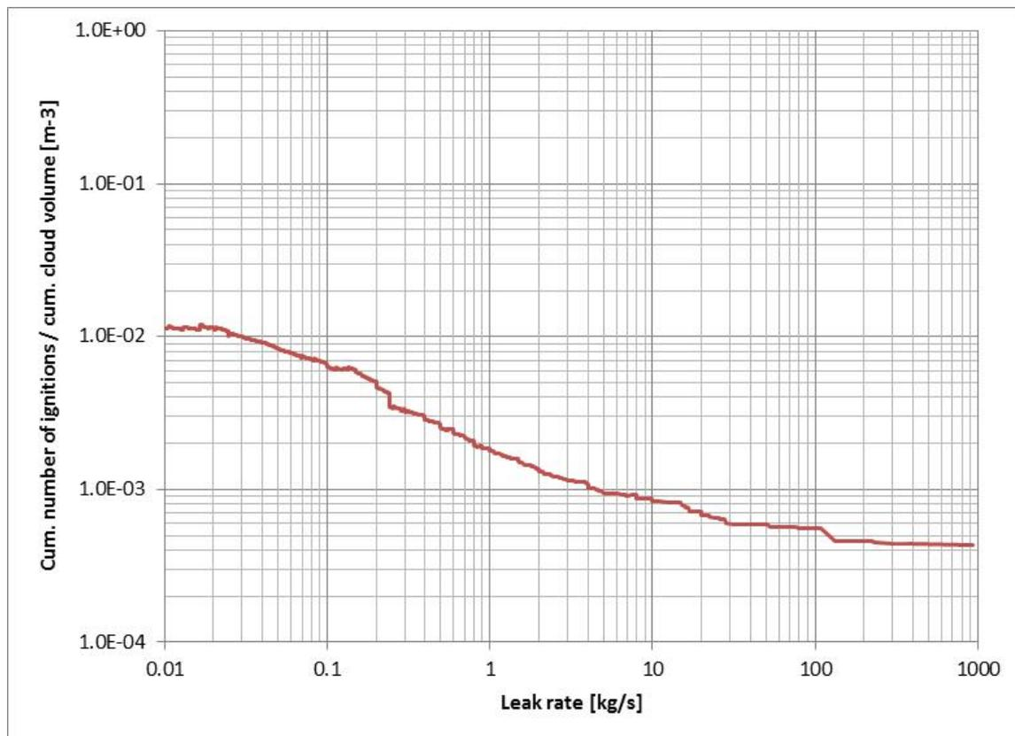
**Figure A 3.5: Ignitions, cloud sizes and leak rates**
