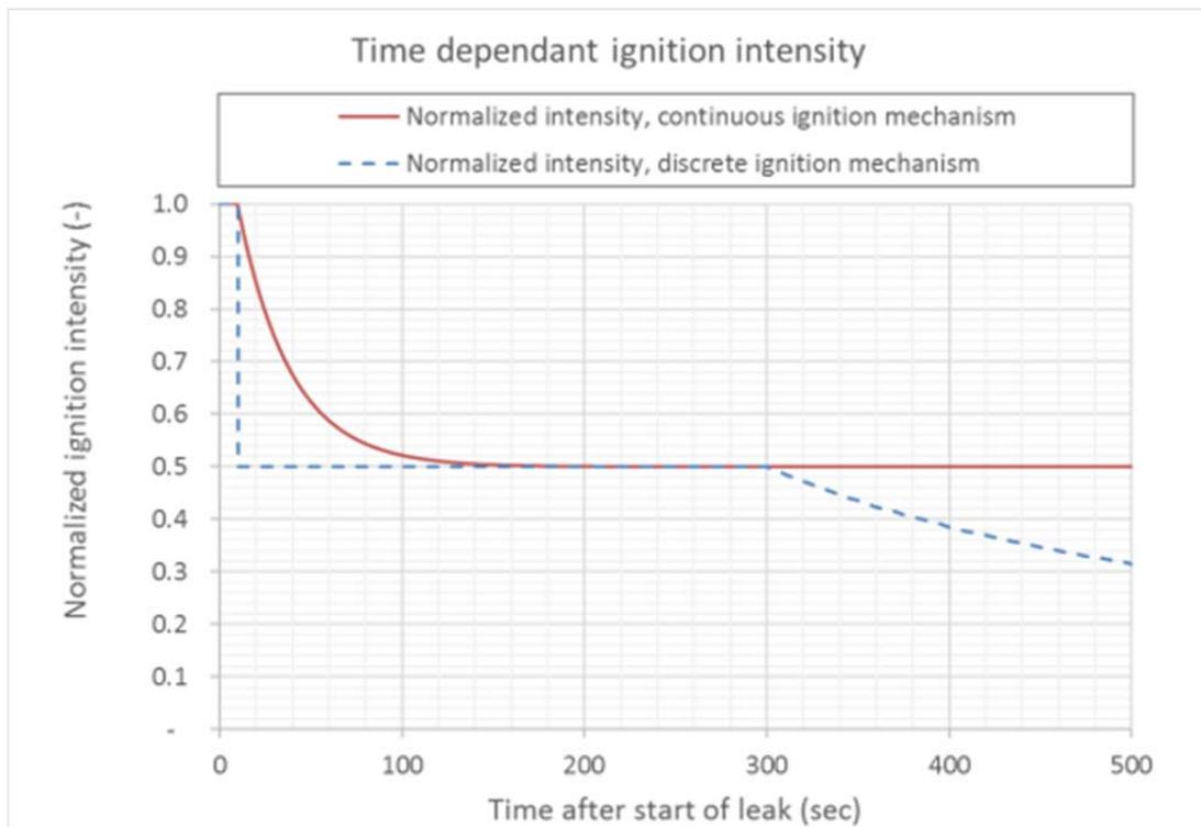
Figure 8.14 – Normalized time dependent ignition intensity for continuous and discrete ignition mechanisms for a typical scenario. This assumes detection at  $t = 5$  sec, a system response time of 5 seconds (*i.e.* delay time from first gas exposure of detectors until isolation of ignition sources has taken place),  $t_{hot} = 20$  sec and  $P_{iso} = 0.5$
