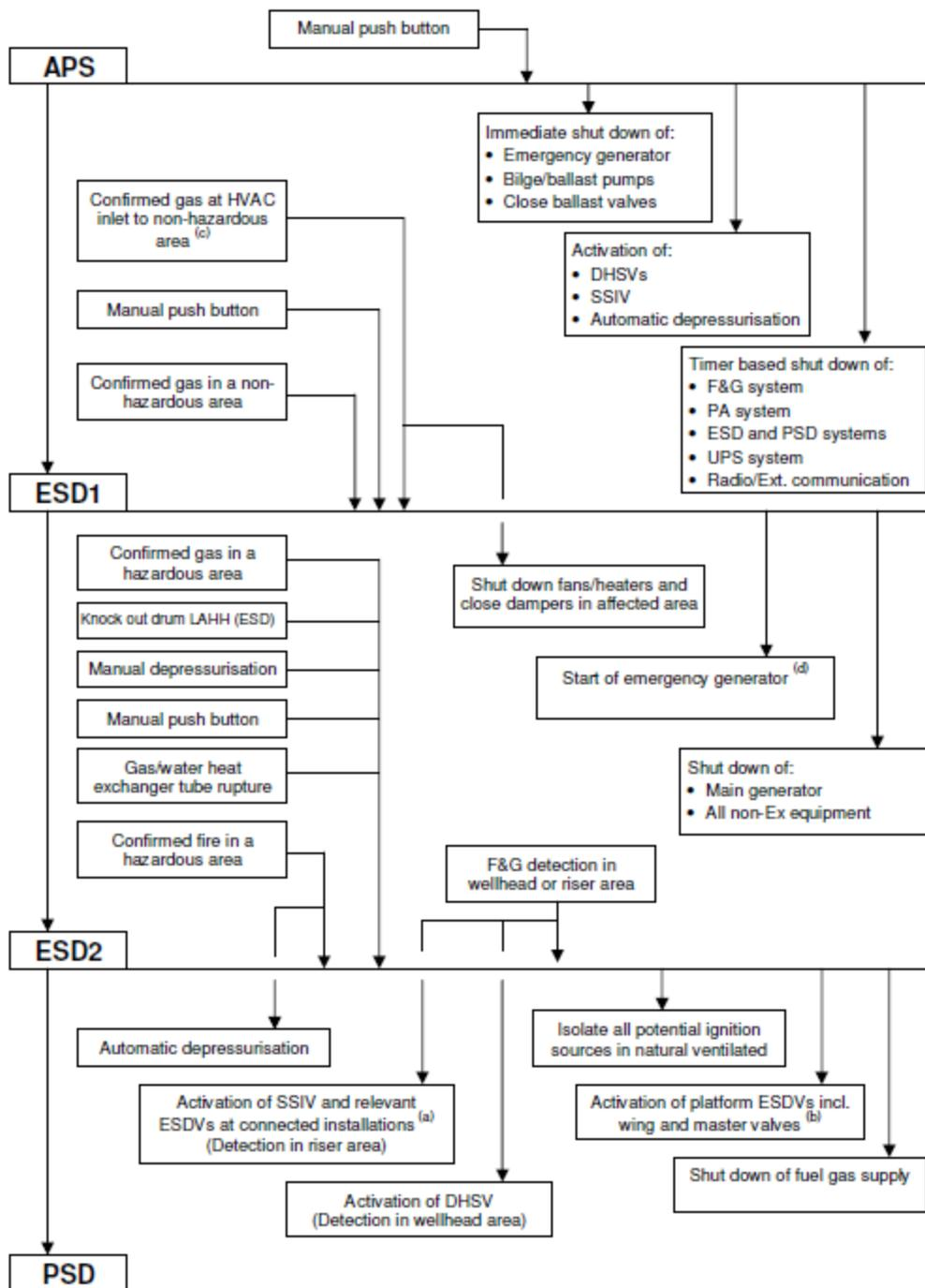
Figure 2 - Emergency shut down (ESD) principle hierarchy
