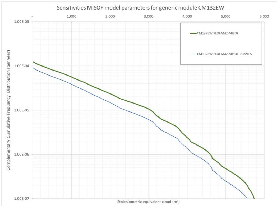
Figure 11.13 – Sensitivity  $P_{iso}$  in MISOF; default values (see Table 8.20) vs. increasing the isolated fraction with a factor of two. The figure shows the complementary cumulative frequency distribution for ignited stoichiometric equivalent gas cloud for the generic module CM132EW
