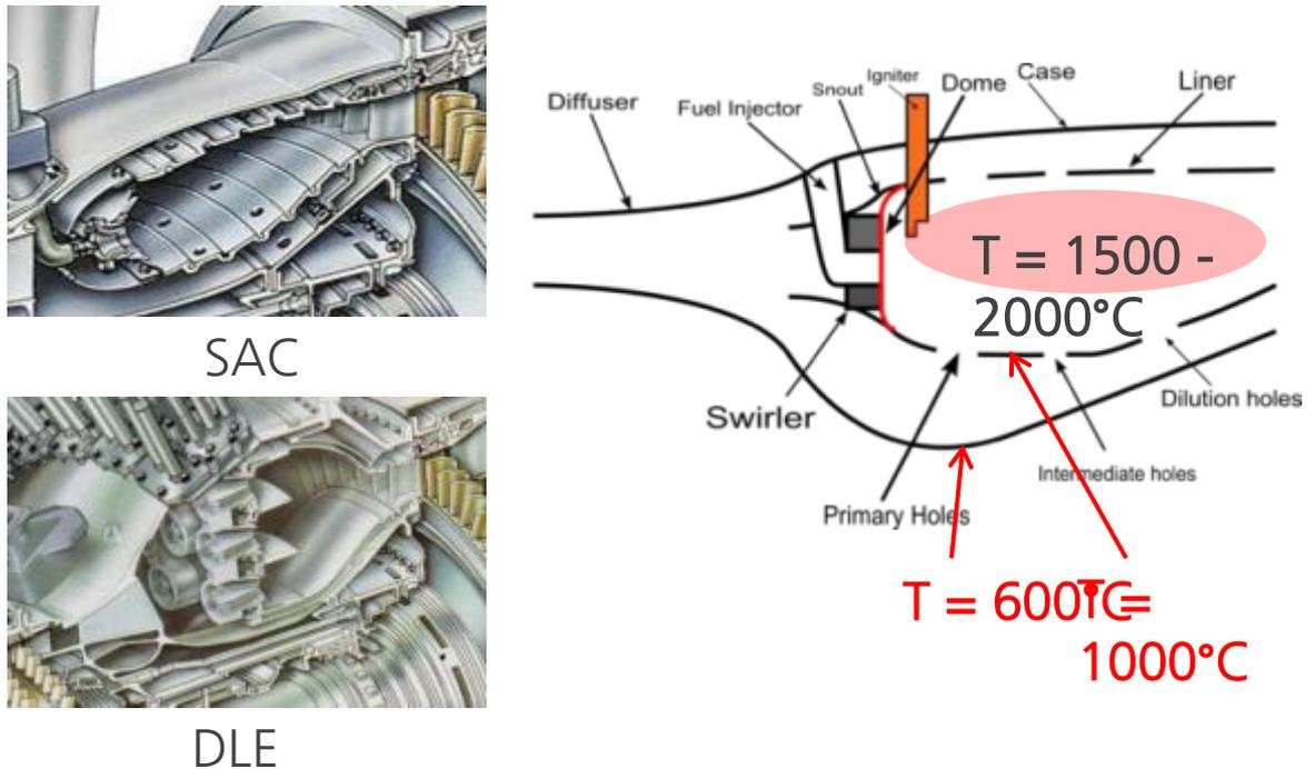
Figure 2.3 - Combustion chamber for LM2500 with inner liner and outer casing, general principles
