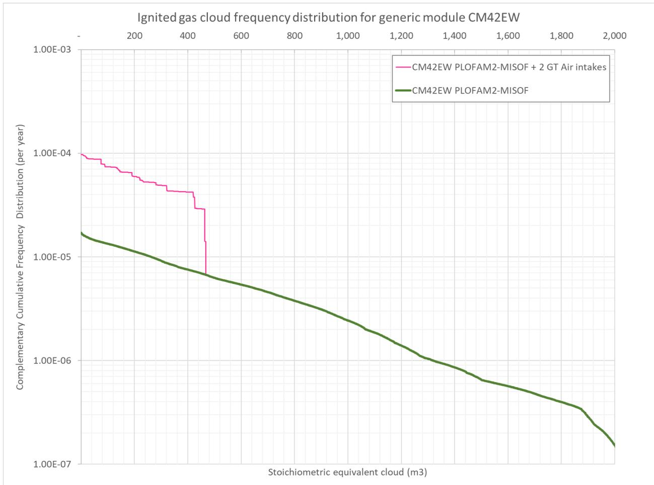
**Figure 4-22: CM42EW PLOFAM-MISOF + two gas turbine air intakes located directly above the module (see Figure 4-21); complementary cumulative frequency distribution for time of ignition of stoichiometric equivalent gas cloud.**
