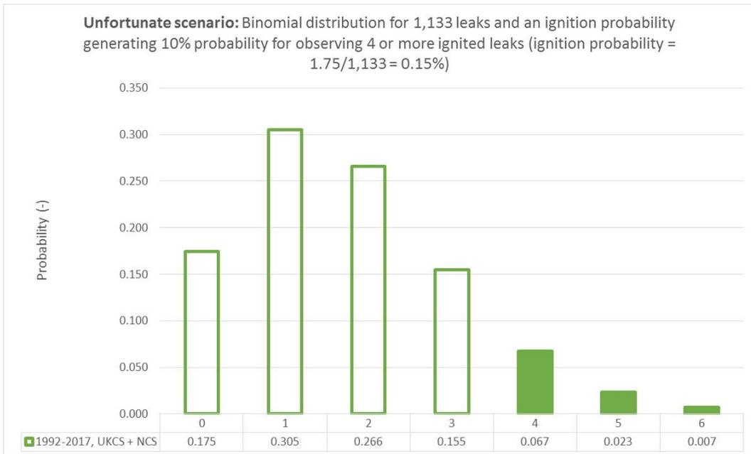
Figure 11.1 – Binomial distribution for the ignition probability (immediate plus delayed) generating 10% probability for observing more than 3 ignited leaks out of 1,133 leaks occurring at installations located on UKCS and NCS in the period 2001-2017 (ignition probability becomes 0.15%)
