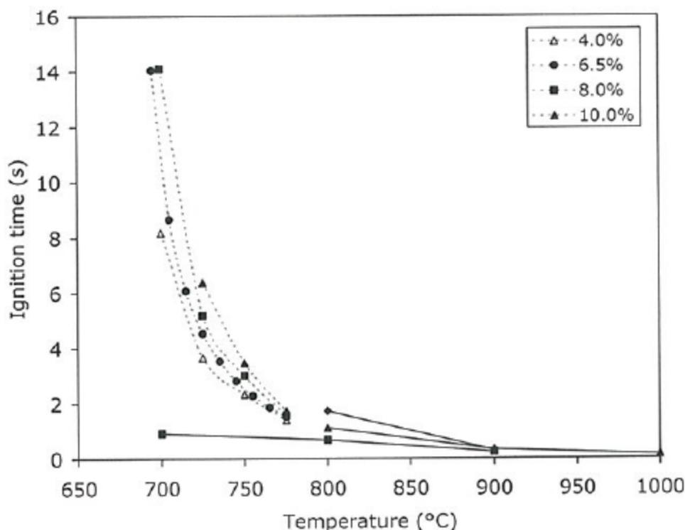
Figure 6.2: Ignition delay time for methane, taken from Ref /2/
