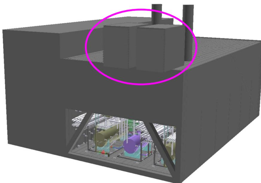
**Figure 4-24: CM132EW location of gas turbine air intakes**
