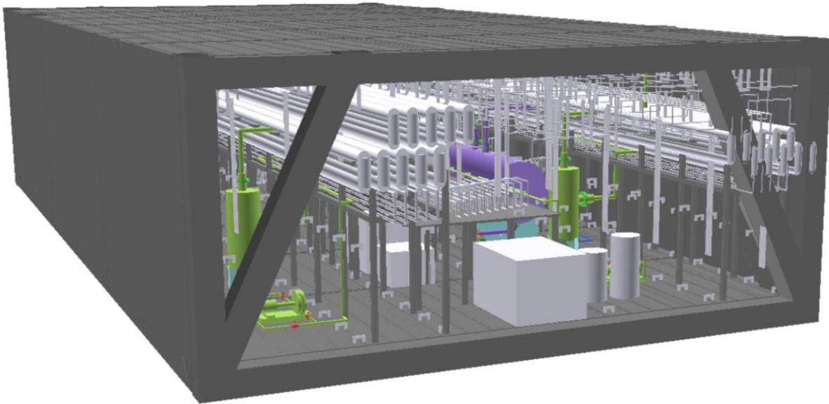
Figure 3-3: M132EW; about 13 000 gross m<sup>3</sup>, two open walls
