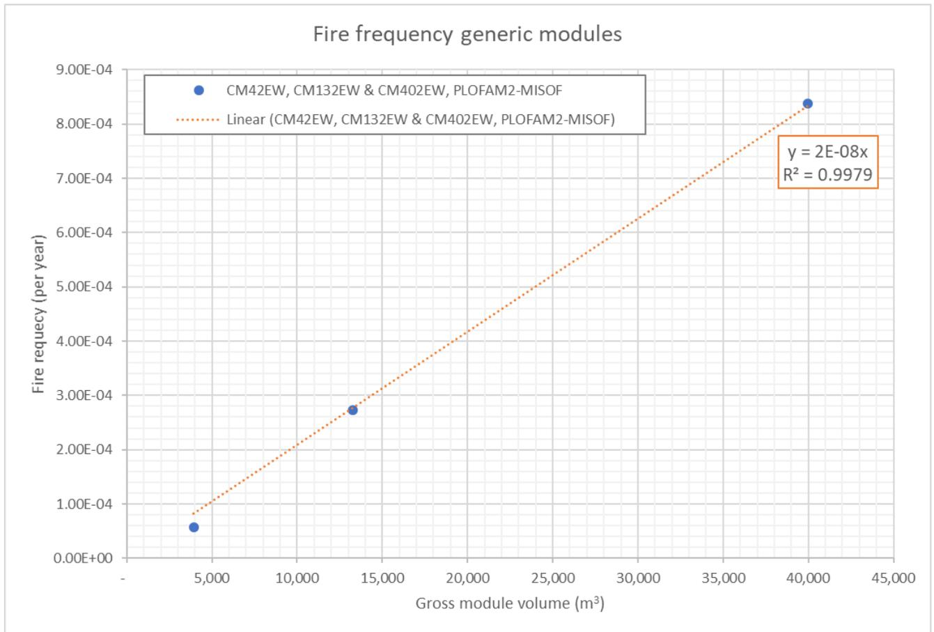
**Figure 6-2: Fire frequency vs. module volume for the various modules**
