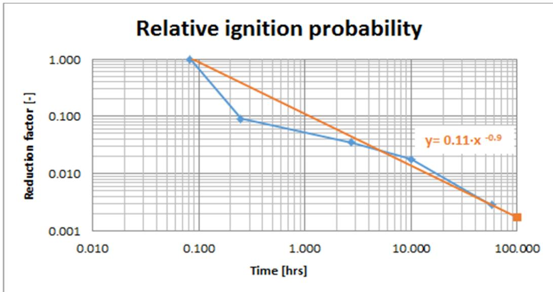
Figure 8.12 - Ignition probability reduction factor for discrete ignition sources more than 5 minutes after start of the leak
