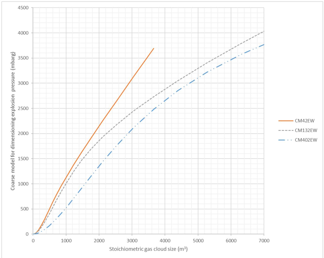
**Figure 3-9: Coarse model for dimensioning explosion pressure.**
