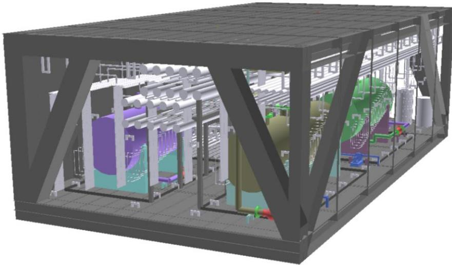
Figure 4-28: CM43ESW; 4 000 gross m<sup>3</sup>, three open walls
