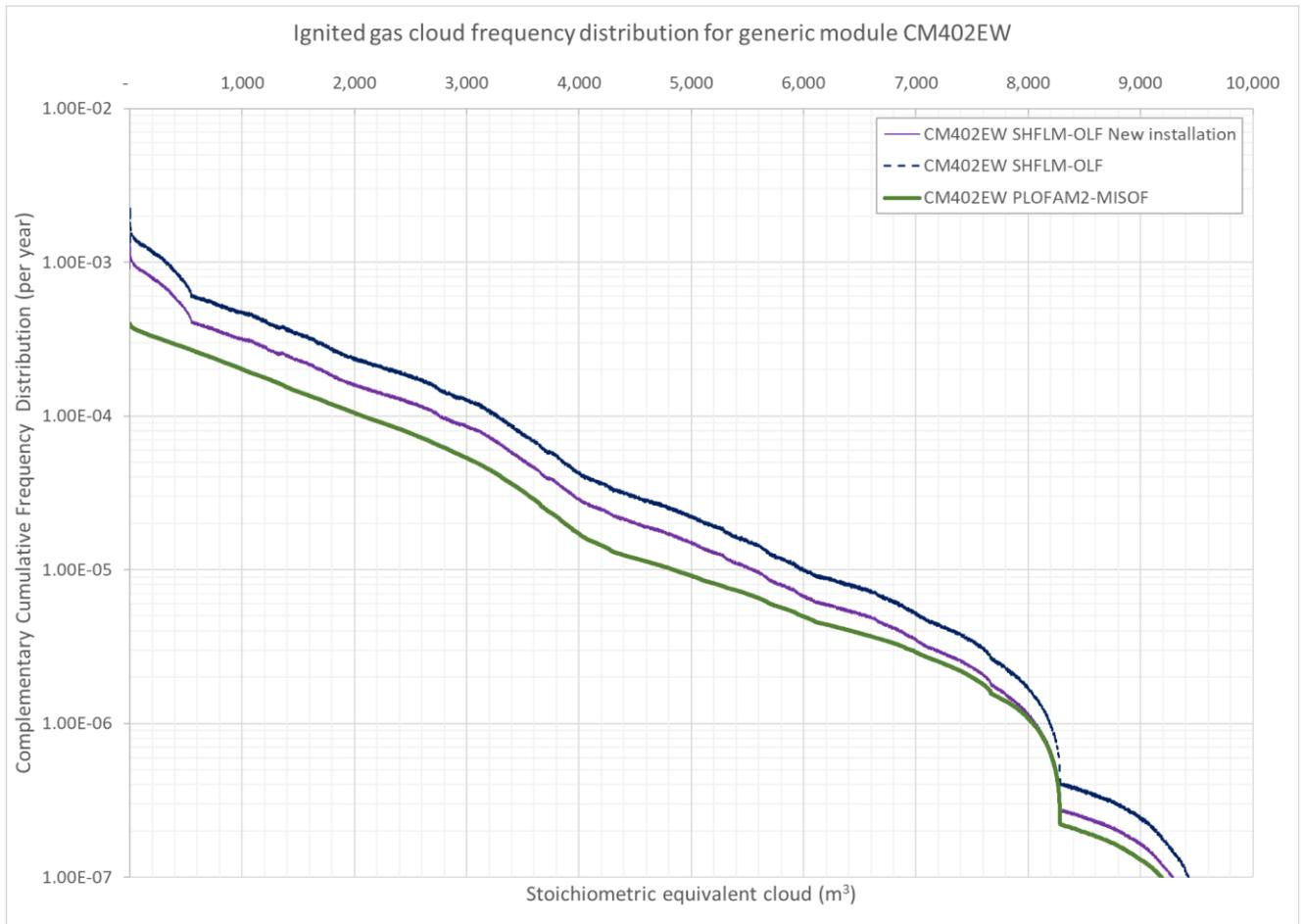
**Figure 4-9: Complementary cumulative frequency distribution for ignited stoichiometric equivalent gas cloud for the generic module CM402EW including sensitivity with OLF model assuming new installation. A correction factor of 0.675 has been used to reflect a new installation (see Table 3-6).**
