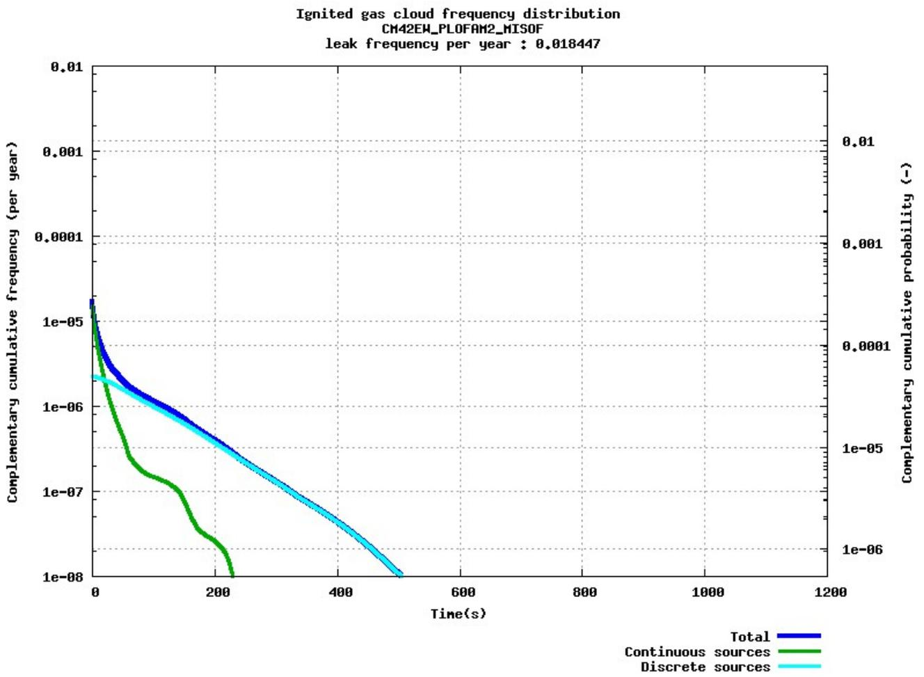
**Figure 4-13: CM42EW PLOFAM-MISOF: Complementary cumulative frequency distribution for time of ignition of stoichiometric equivalent gas cloud.**
