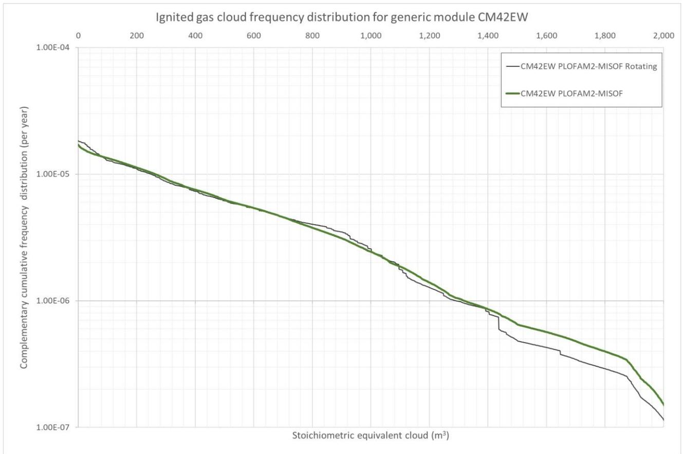
**Figure 4-19: CM42EW PLOFAM-MISOF with specific modelling of 4 pumps instead of generic volumetric modelling of rotating machinery; complementary cumulative frequency distribution for time of ignition of stoichiometric equivalent gas cloud.**
