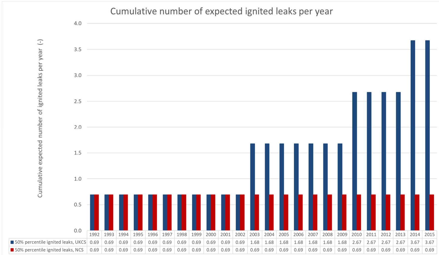
Figure 7.7 – Cumulative number of ignited PLOFAM leaks per year for the period 1992 and onwards including the effect of randomness (using 50% percentile in binomial distribution as premise for estimation of the underlying ignition probability)
