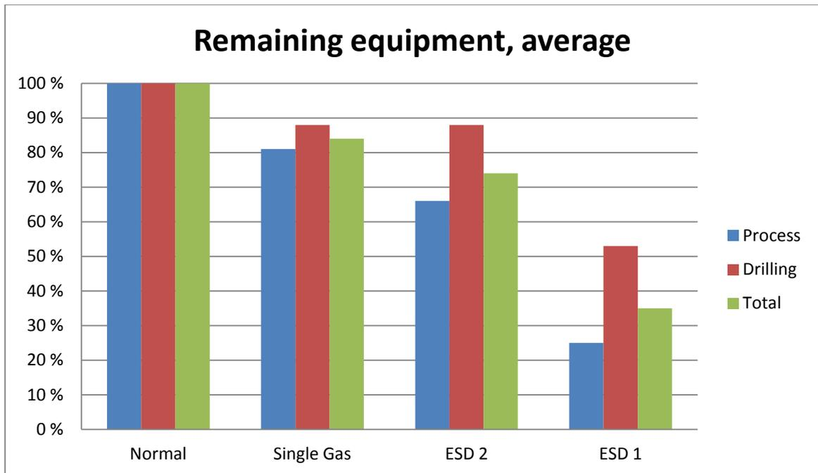
Figure 5.4: Average isolation factor F for Platform A and Platform B, scaled for Ex protection.
