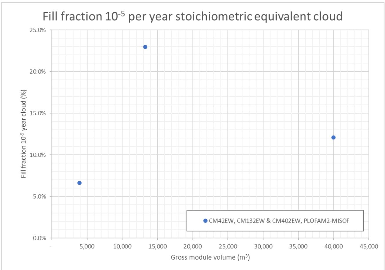
**Figure 6-8: Fill fraction 10<sup>-5</sup> per year stoichiometric equivalent volume vs. module volume for the three modules**
