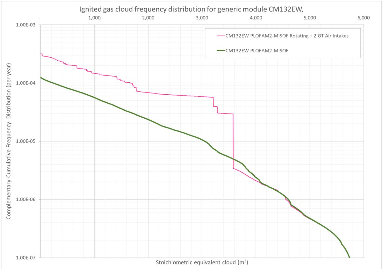
**Figure 4-23: CM132EW PLOFAM2-MISOF with specific modelling of 12 pumps instead of generic volumetric modelling of rotating machinery + two gas turbine air intakes located directly above the module (see Figure 4-24); complementary cumulative frequency distribution for time of ignition of stoichiometric equivalent gas cloud.**
