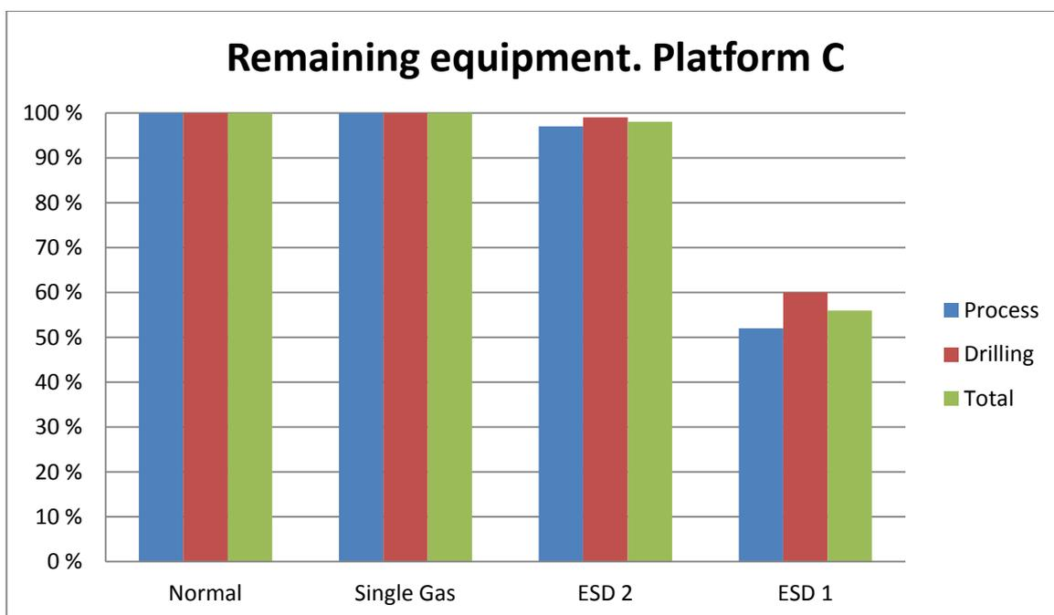
Figure 5.3: Isolation factor F for equipment on Platform C, scaled for Ex protection
