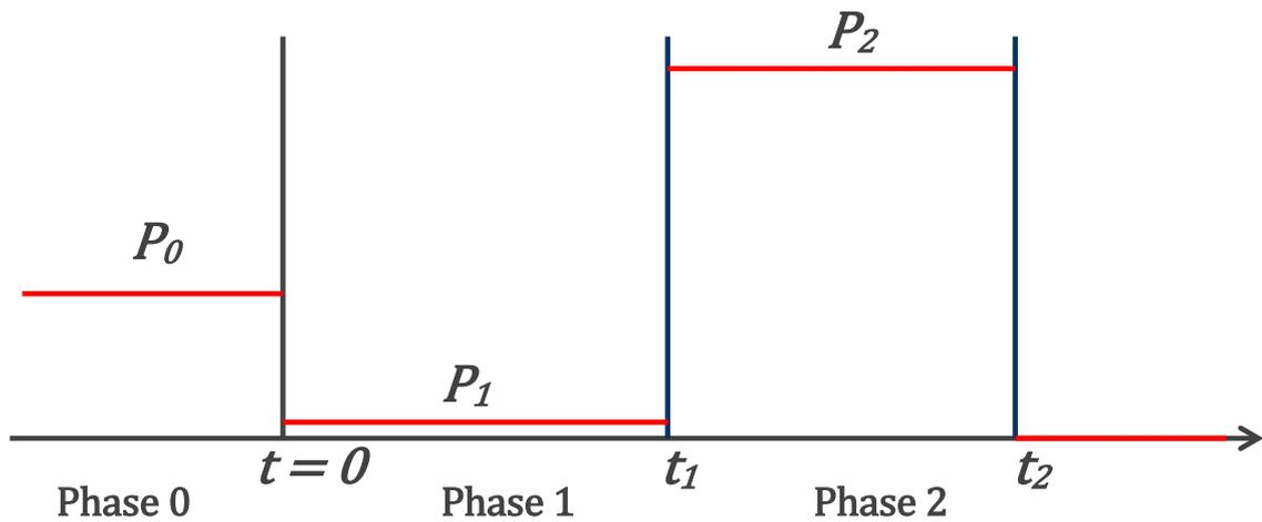
Figure 2.7 - The phases and parameters of the gas turbine ignition model
