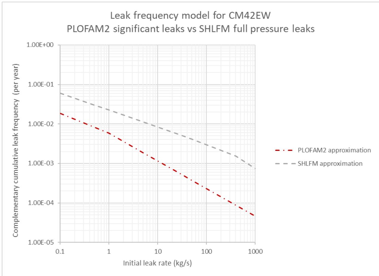
**Figure 3-6: Leak frequency distributions for CM42EW.**
