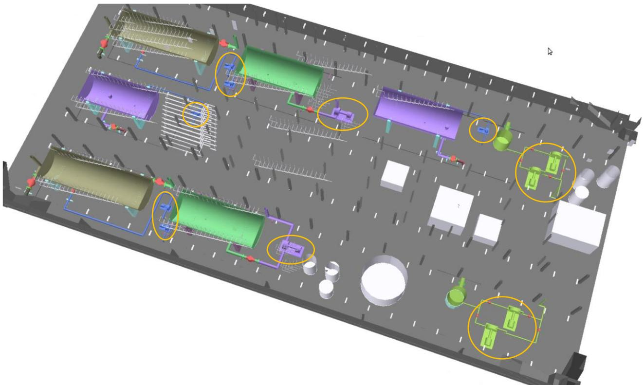
**Figure 4-18: CM132EW: Bird's view displaying location of pumps**
