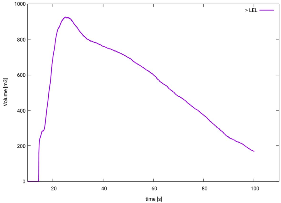
Figure 3.10 - Leak ID 154: Time history for the volume of gas with concentration higher than LFL,  $V_{>LFL,154}(t)$ , estimated by CFD simulation performed with Kamelon FireEx KFX®
