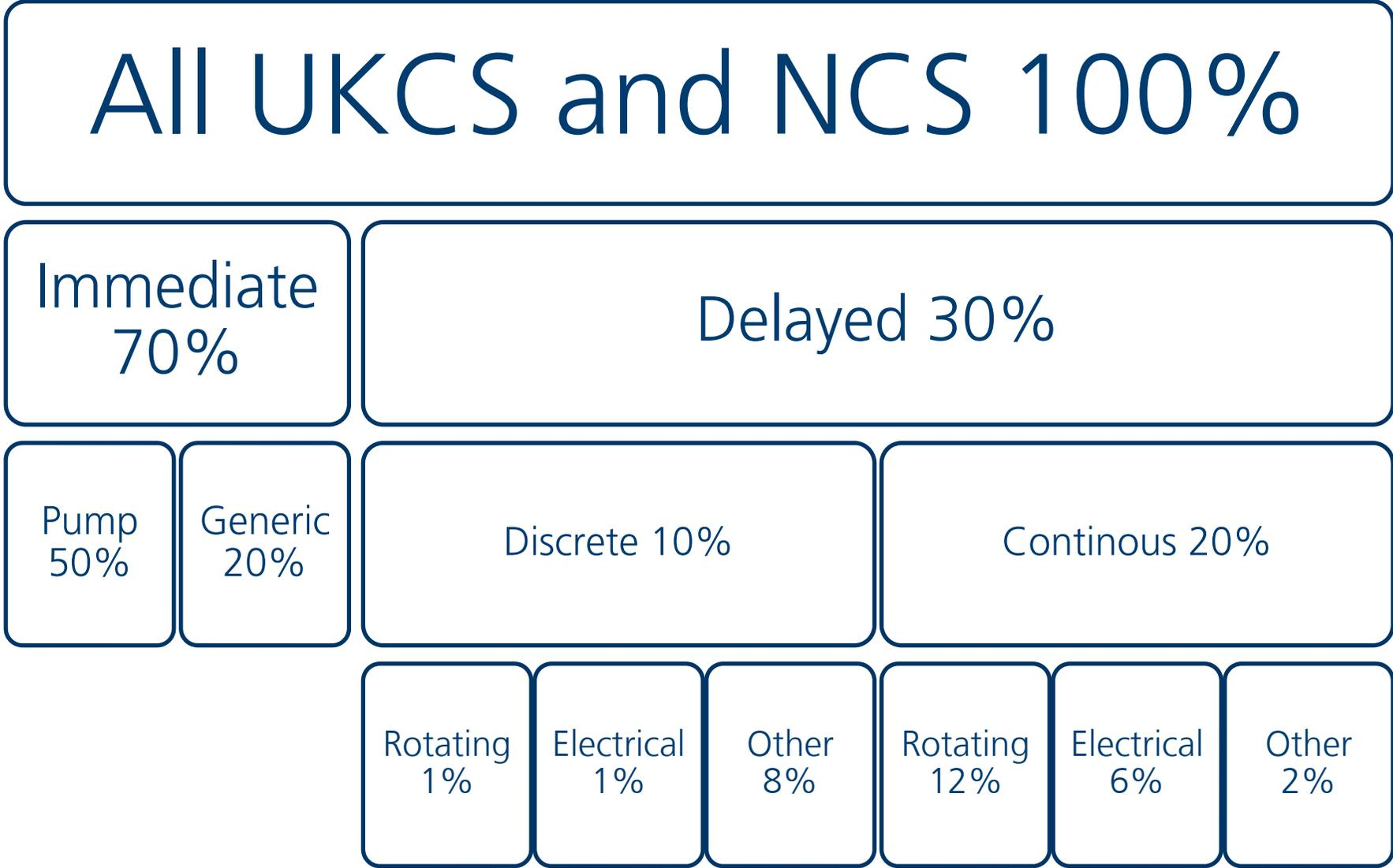
Figure 8.7 - Overview resulting distribution of relevant ignited leaks for MISOF parameters for objects intended for use in potentially explosive atmospheres
