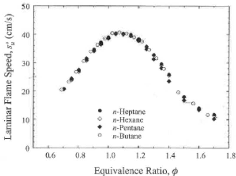
Figure 2.9 - Effect of stoichiometry on laminar burning velocities, from Ref. /6/
