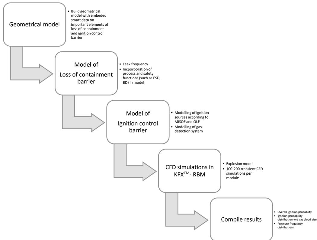
**Figure 3-1: Main steps in methodology for testing of MISOF using the risk analysis software Kameleon FireEx Risk & Barrier Management (KFX-RBM)**
