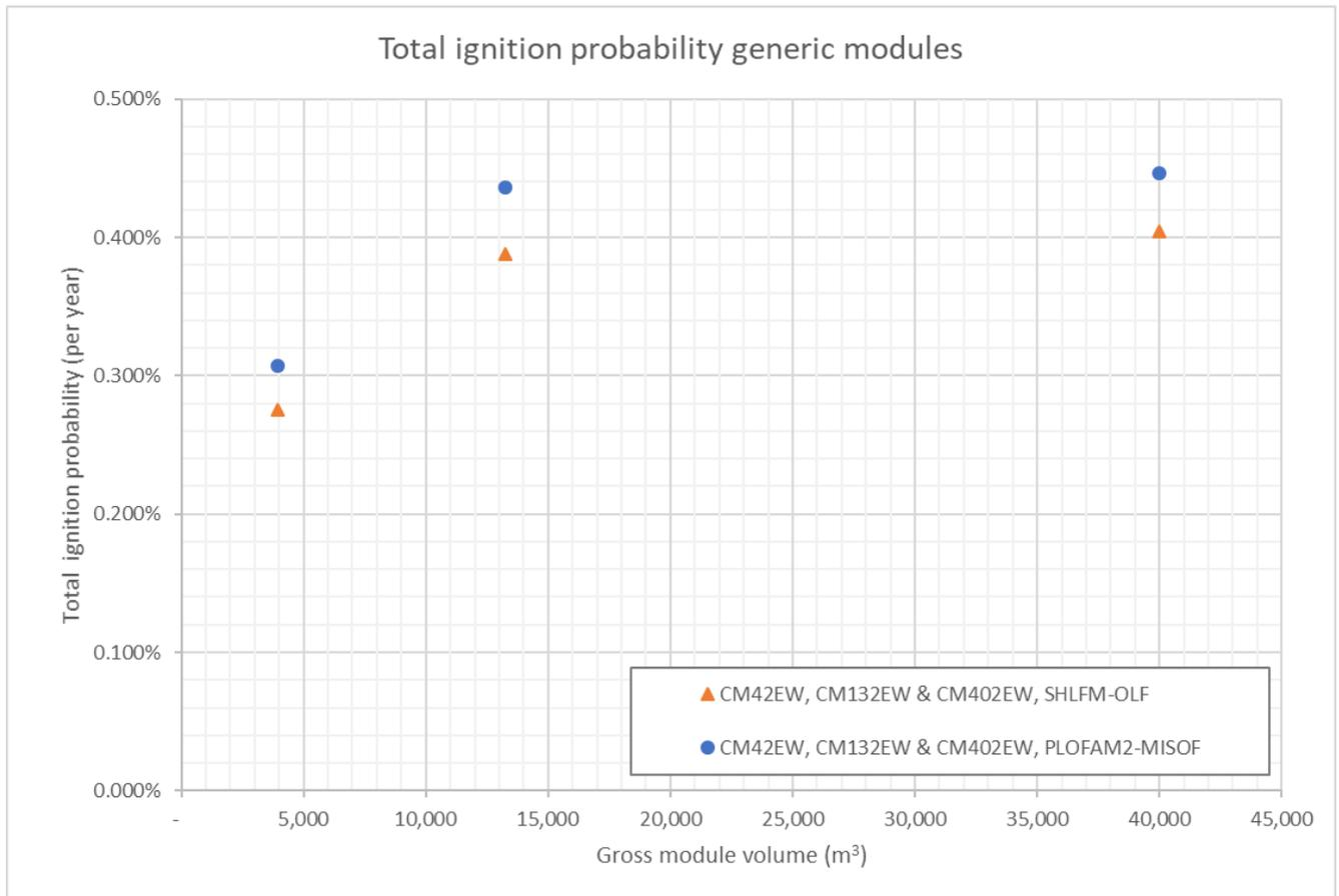
**Figure 4-6: Total ignition probability vs. module volume for the various modules and probabilistic models**
