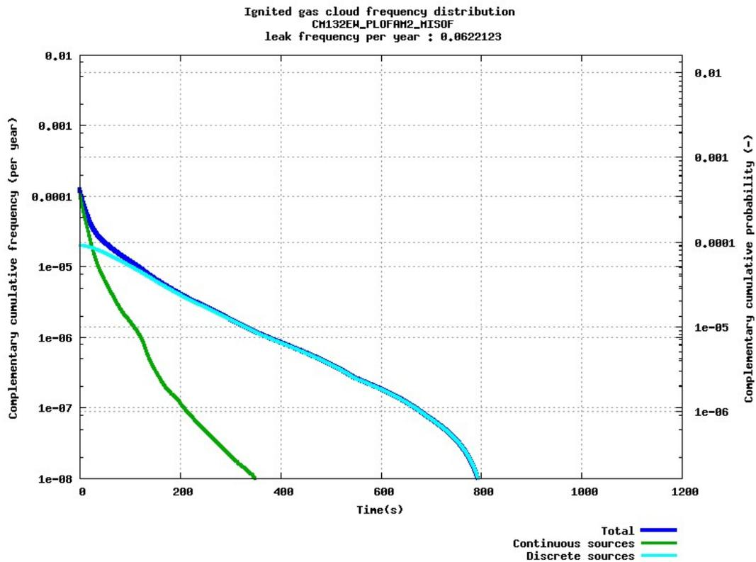
Figure 11.12 – PLOFAM-MISOF: Complementary cumulative frequency distribution for time of ignition of stoichiometric equivalent gas cloud
