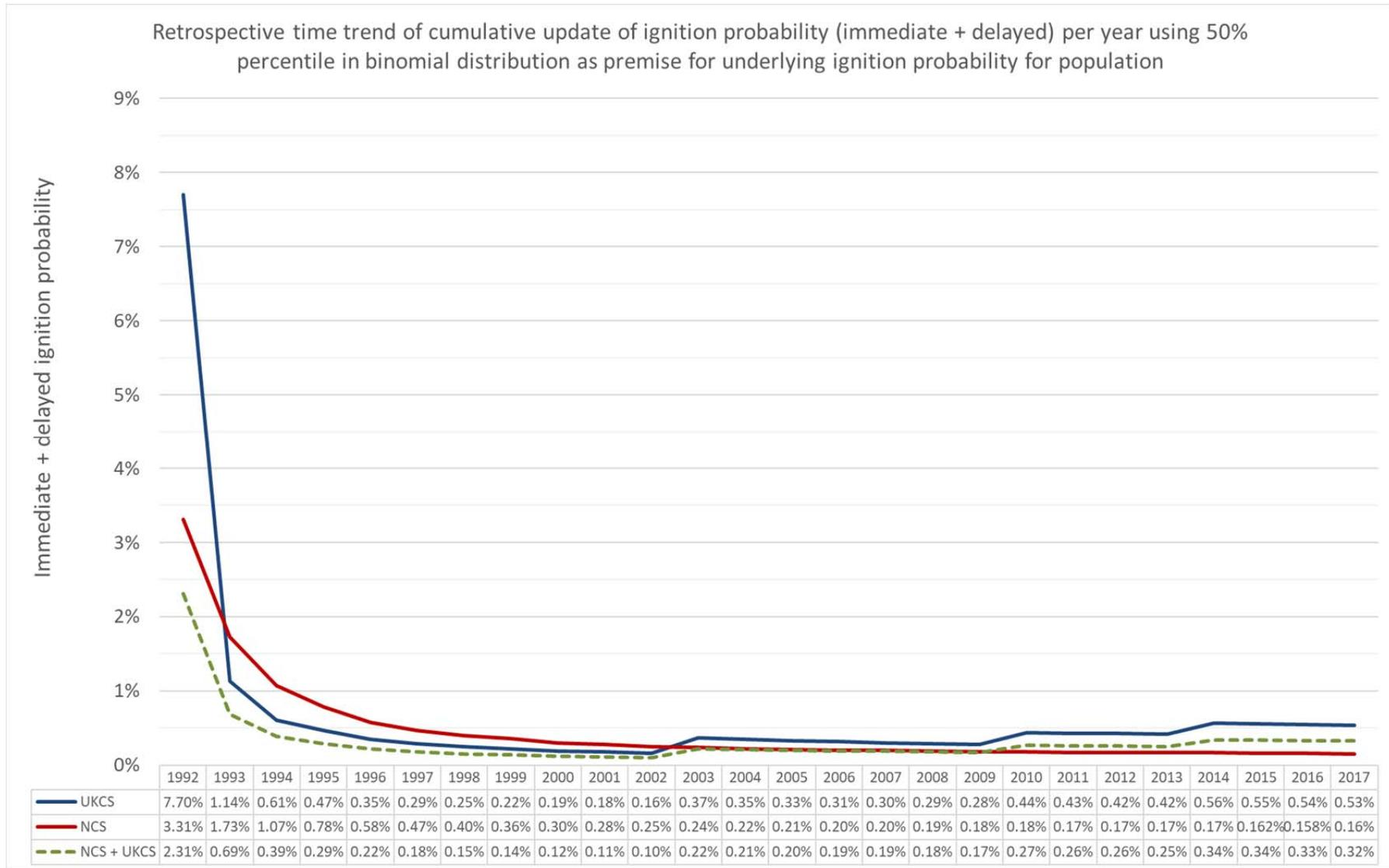
Figure 7.8 – Retrospective time trend of cumulative update for ignition probability per year (immediate plus delayed) using 50% percentile in binomial distribution as premise for estimation of the underlying ignition probability
