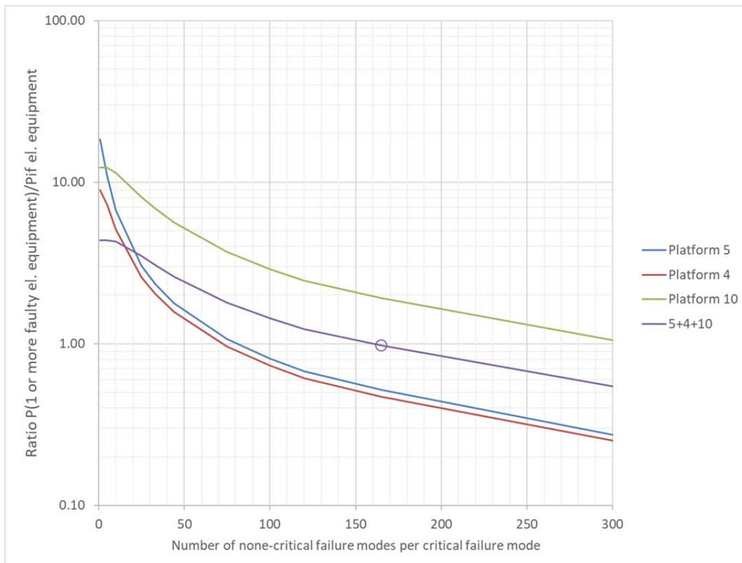
Figure 8.10 - Probability of one or more units of faulty Zone 2 or Zone 1 equipment divided by the conditional ignition probability obtained from  $\lambda_{i,C}$  and  $\lambda_{i,D}$ , for increasing numbers of non-critical failure modes per critical failure mode. The result for all platforms altogether equals 1 for a number of non-critical failure modes per critical failure mode of about 165 (marked with a circle)
