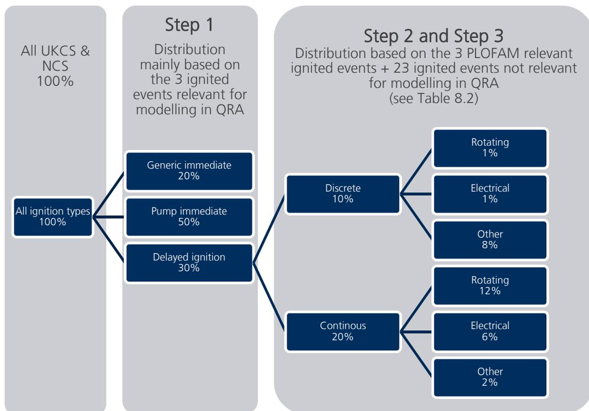
Figure 8.2 - Application of data and resulting distribution of observed ignited events for parameterisation of MISOF parameters
