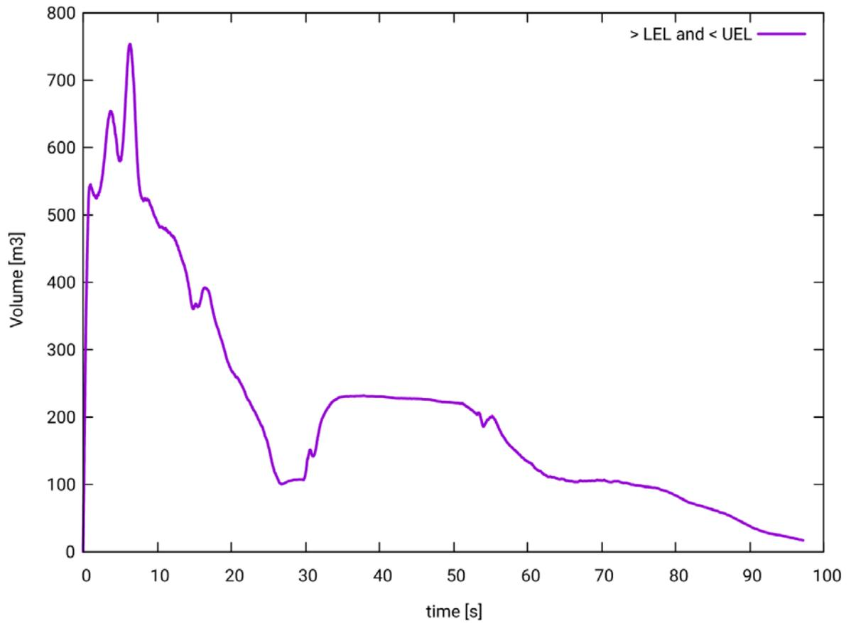
Figure 3.9 - Leak ID 146: Time history for the combustable volume of gas,  $V_{LFL:LEL,146}(t)$ , estimated by CFD simulation performed with Kamelon FireEx KFX®
