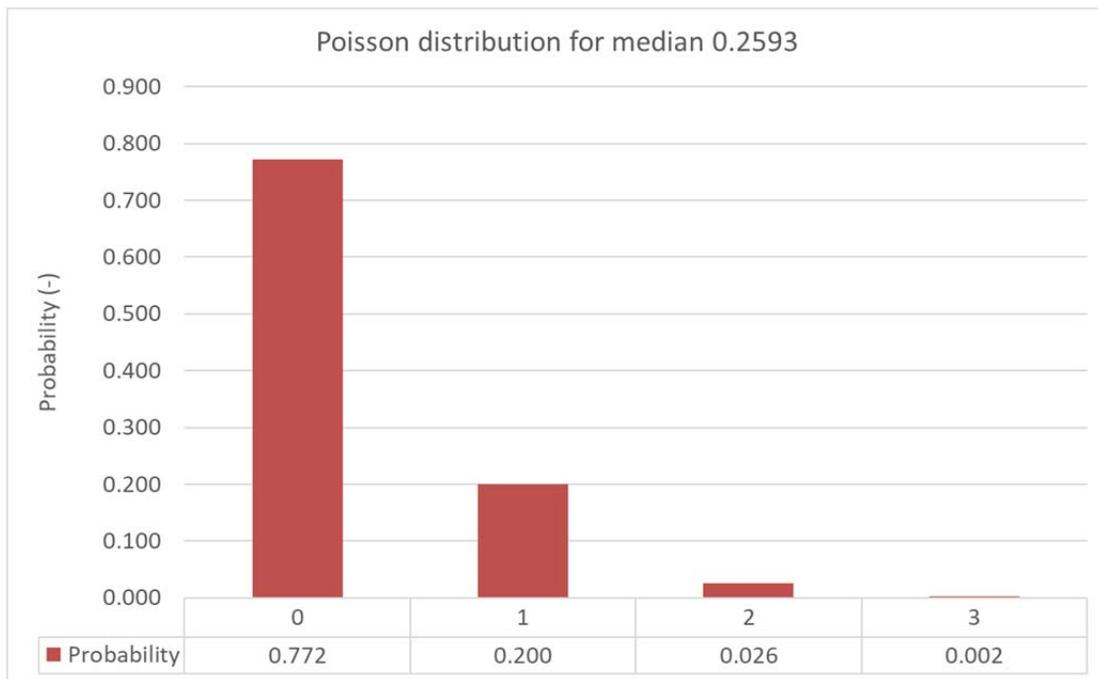
Figure 8.9 – Poisson probability distribution for number of ignitions resulting from an exposed volume of 120,797 m<sup>3</sup> (25,800 m<sup>3</sup>+ 55,553 m<sup>3</sup>+39,444 m<sup>3</sup>) in 201 seconds based on  $\lambda_{i,C}$  and  $\lambda_{i,D}$  presented in Table 8.16.
