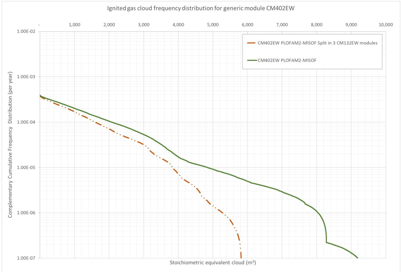
**Figure 5-4: PLOFAM-MISOF: Complementary cumulative frequency distribution for dimensioning explosion load. Sensitivity case representing a design where the CM402EW module is split into three identical CM132EW modules. The aggregated ignited cloud distribution for all three modules is established by multiplying the distribution for CM132EW (see Figure 4-11) with a factor of 3.**
