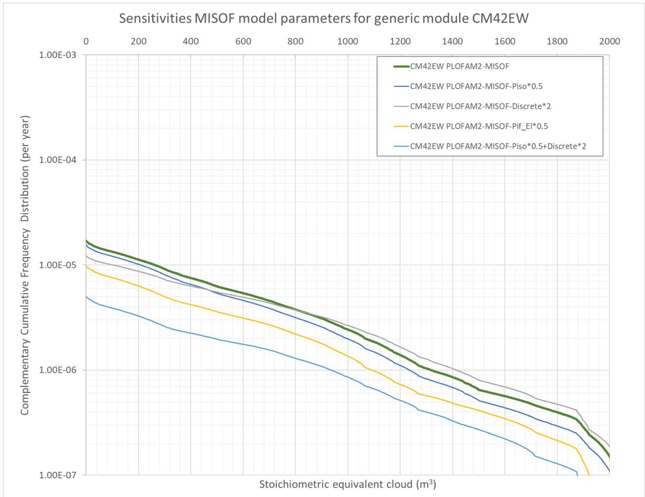
**Figure 4-31: Sensitivities MISOF model parameters: Complementary cumulative frequency distribution for ignited stoichiometric equivalent gas cloud for the generic module CM42EW.**
