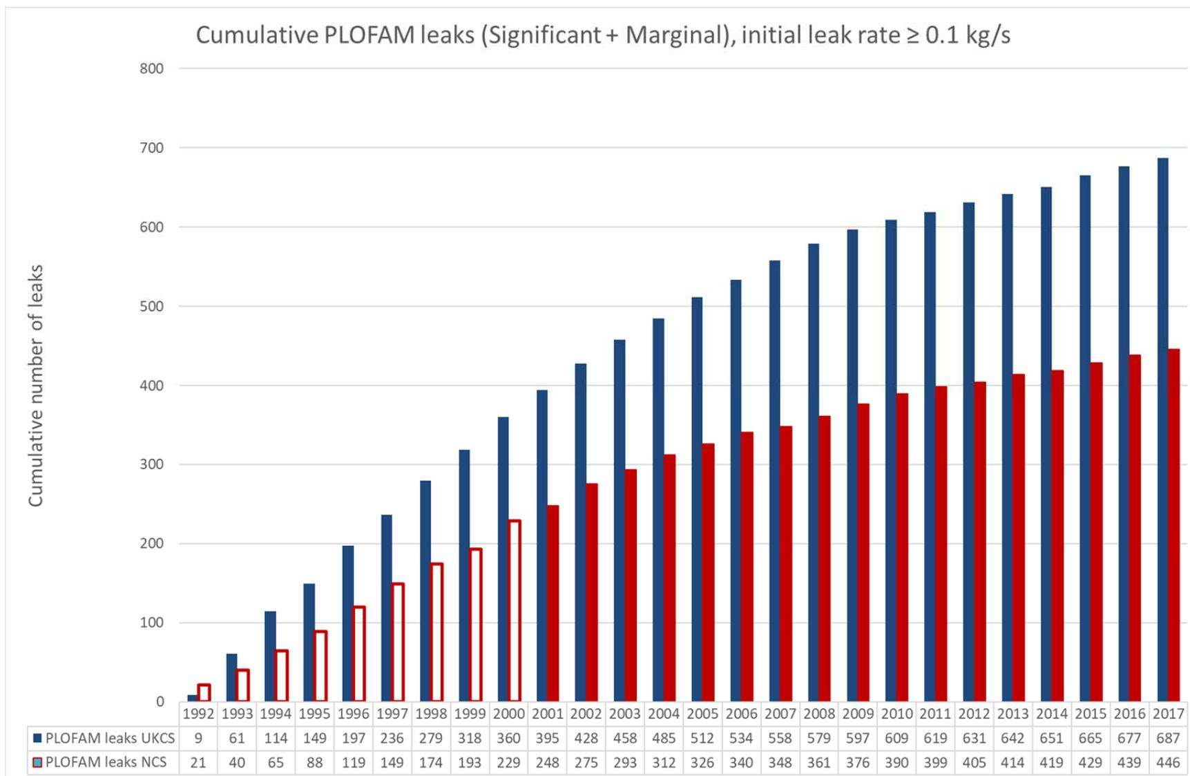
Figure 7.6 – Cumulative number of PLOFAM leaks per year for the period 1992 and onwards. The data for installations on the NCS before 2001 is estimated based on various data sources, and there is some uncertainty associated with this data. The data for this period is therefore marked with unfilled bars
