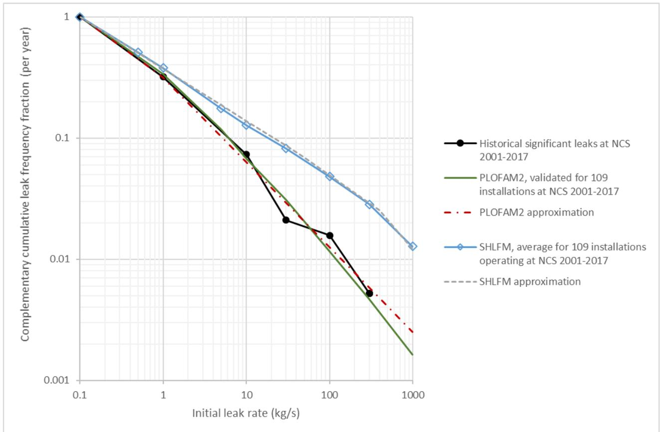
**Figure 3-5: Leak frequency fraction distribution approximations. The PLOFAM approximation applies to significant leaks. The SHLFM approximation applies to both full and limited leaks.**
