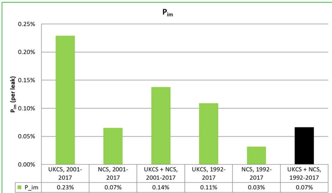
Figure 8.4 - Immediate ignition probability for equipment other than pumps. The concluded parameter to be used in the MISOF model is shown in black colour
