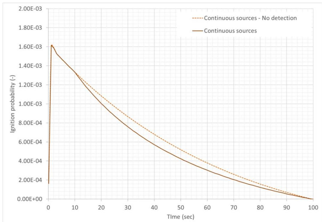
Figure 10.4 – Time dependent ignition probability calculated from equation (10.3) and using the total  $\lambda_{i,C}$  for all equipment categories found in Table 10.2. Gas detection take effect at  $t = 10$  seconds
