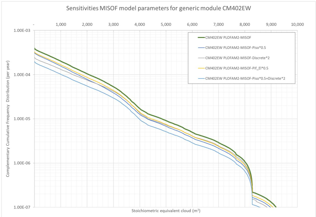
**Figure 4-33: Sensitivities MISOF model parameters: Complementary cumulative frequency distribution for ignited stoichiometric equivalent gas cloud for the generic module CM402EW.**
