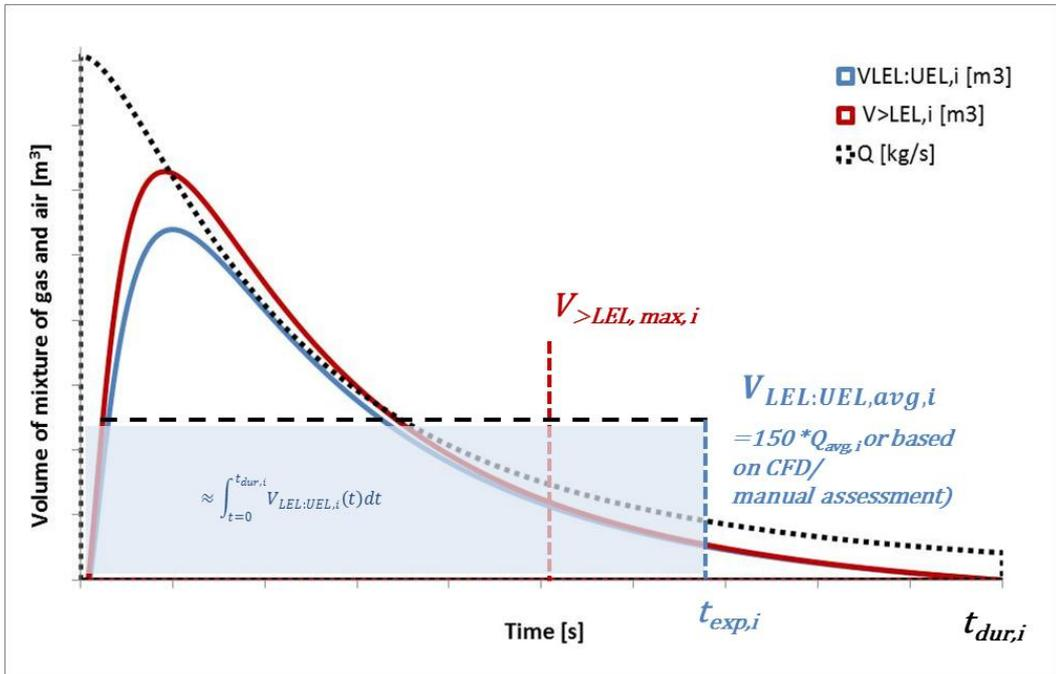
Figure 3.3 - Example a); time dependent gas cloud volume for a transient leak in a typical offshore process module and corresponding graphical representation of the estimation by generic gas exposure model. The example displays a case where the generic model generates quite accurate estimate of the actual gas cloud parameters
