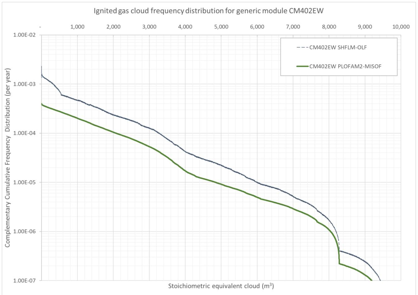
**Figure 4-3: Complementary cumulative frequency distribution for ignited stoichiometric equivalent gas cloud for the generic module CM402EW.**
