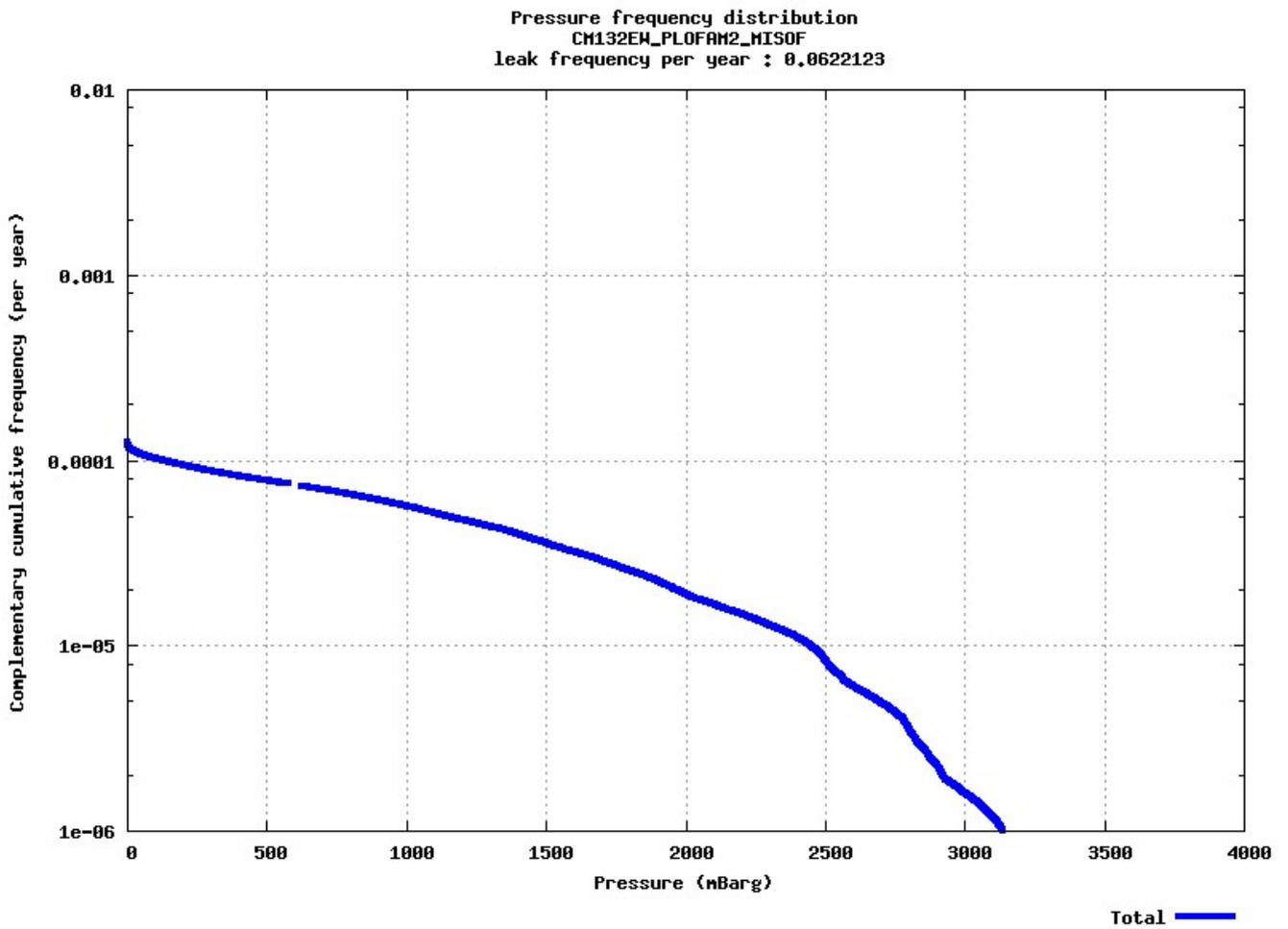
Figure 5-2: CM132EW PLOFAM-MISOF: Complementary cumulative frequency distribution for dimensioning explosion load
