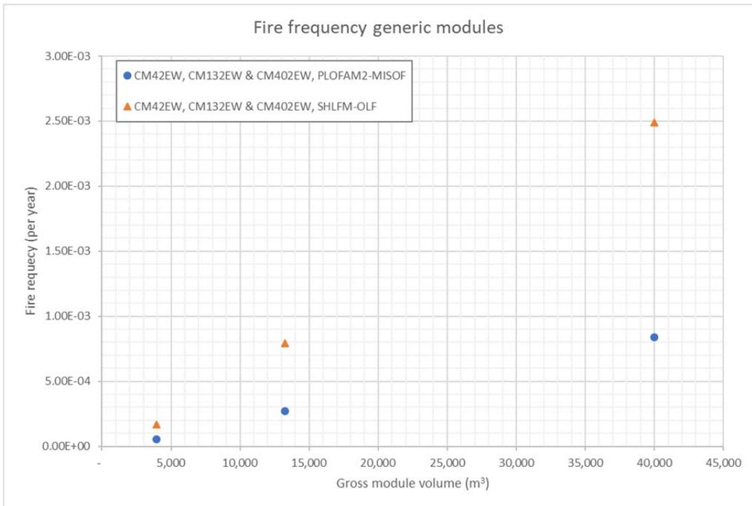
Figure 11.11 – Fire frequency vs. module volume for the various modules and probabilistic models
