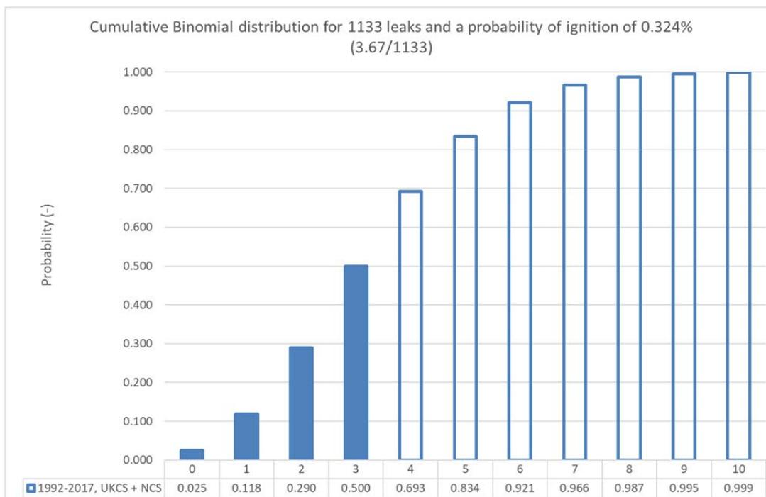
Figure 7.4 – Cumulative binomial distribution for 1133 leaks assuming a probability of ignition of 0.34%, which mathematically corresponds to 3.67 ignited leaks per 1133 leaks
