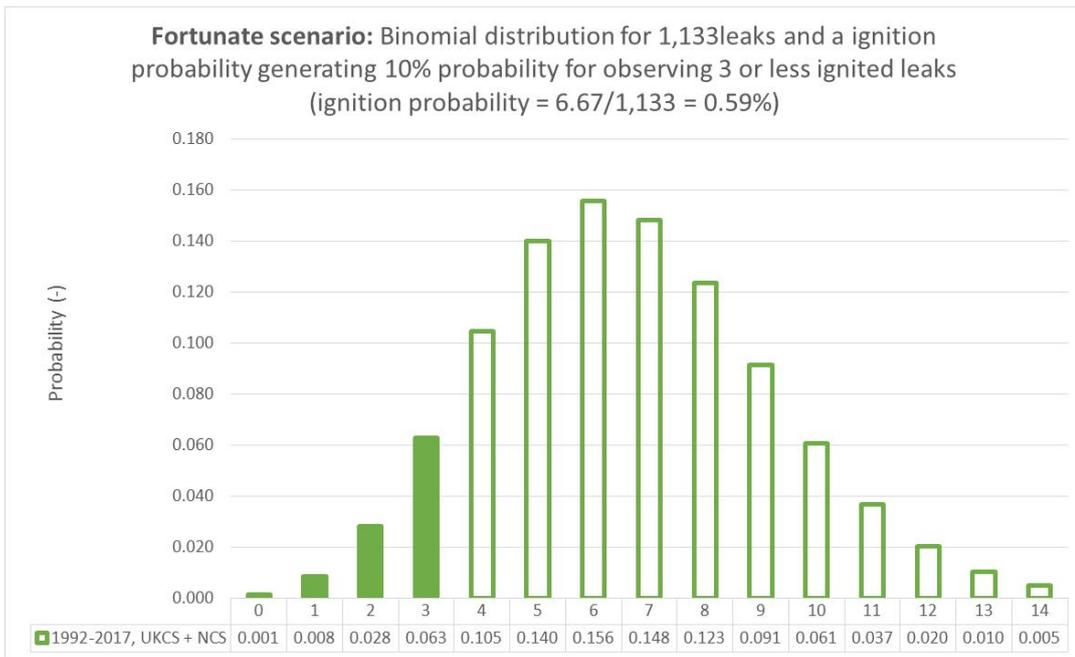
Figure 11.2 – Binomial distribution for the ignition probability (immediate plus delayed) generating 10% probability for observing 3, or fewer, ignited leaks out of 1,133 leaks occurring at installations located on UKCS and NCS in the period 2001-2017 (ignition probability becomes 0.59%)
