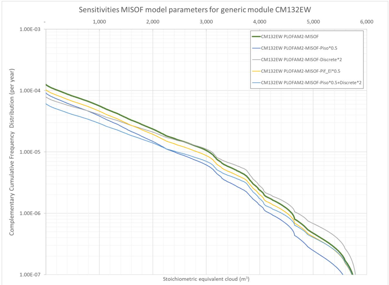
**Figure 4-32: Sensitivities MISOF model parameters: Complementary cumulative frequency distribution for ignited stoichiometric equivalent gas cloud for the generic module CM132EW.**
