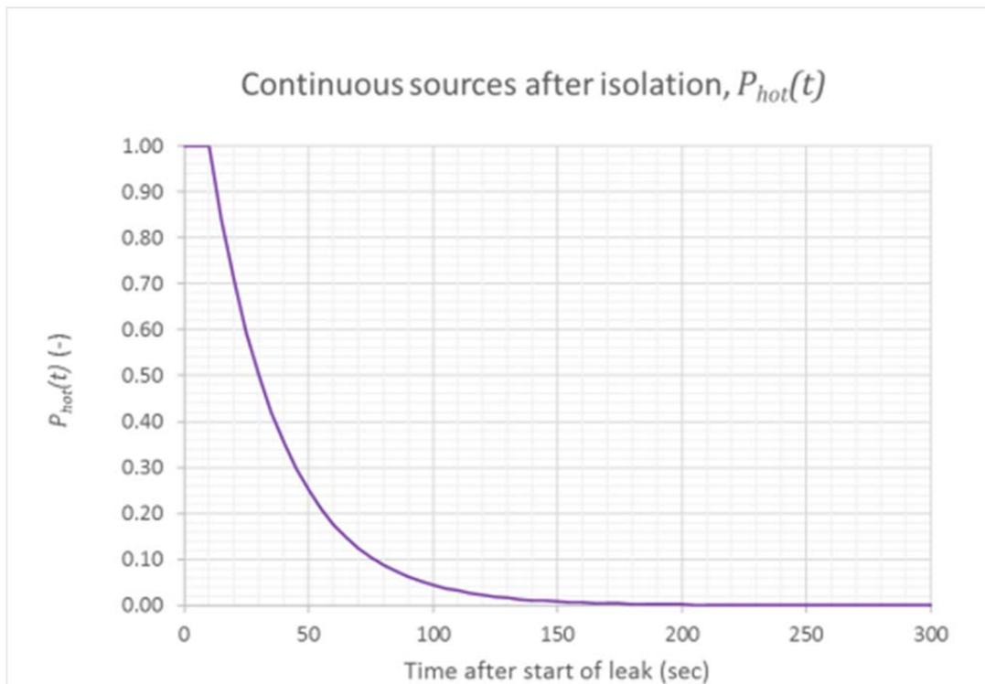
Figure 8.13 – Continuous sources after isolation to account for cooling of hot surfaces for a cooling half time of 20 sec ( $t_{hot} = 20 \text{ sec}$ ) and isolation at 10 seconds after start of leak ( $t_{iso} = 10 \text{ sec}$ )
