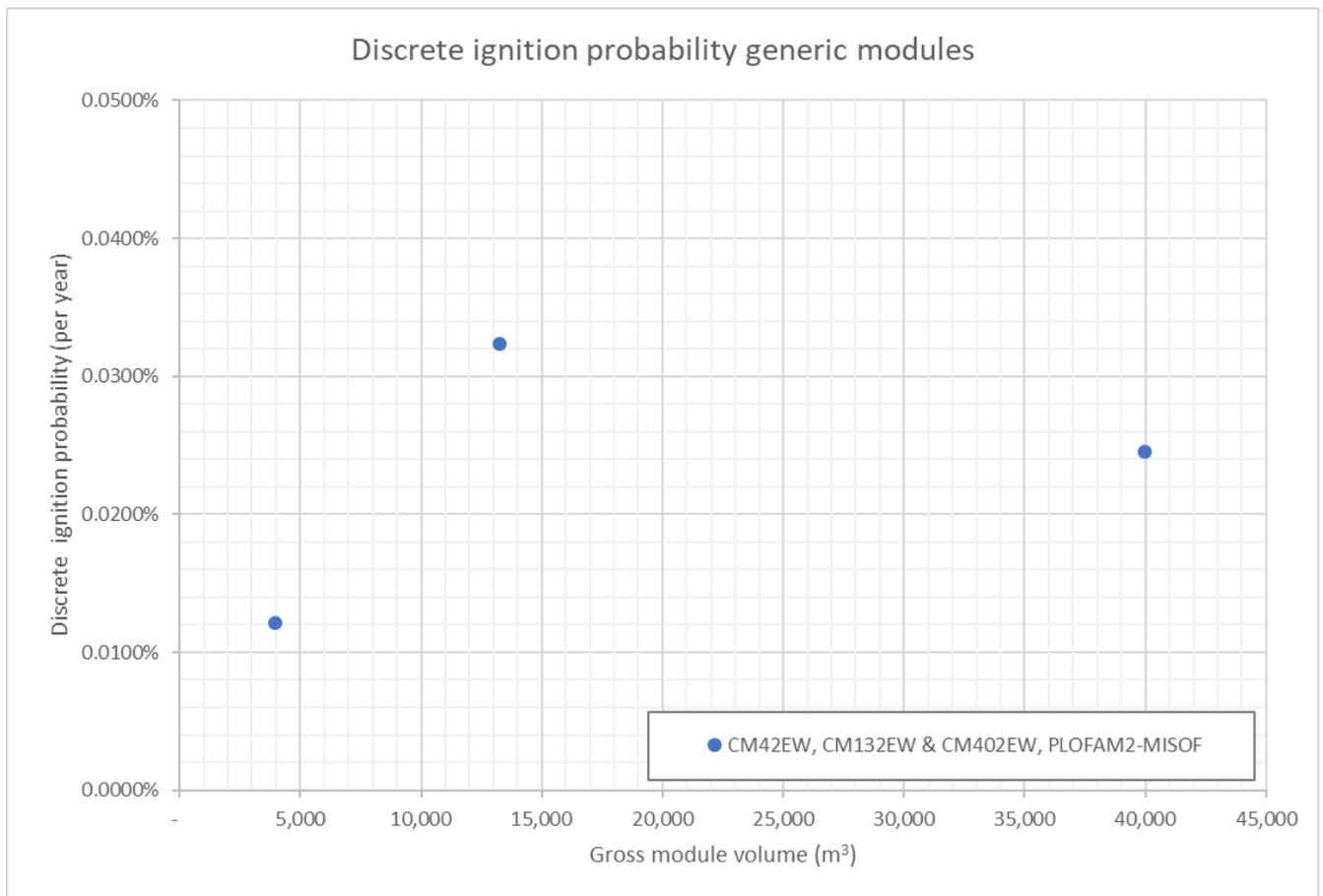
**Figure 6-6: Discrete ignition probability vs. module volume for the various modules**
