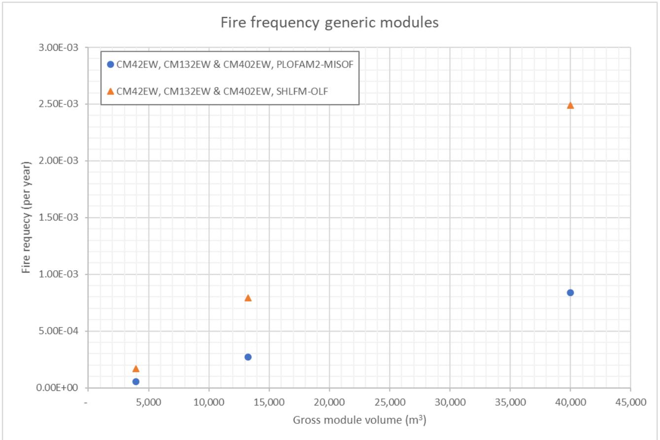
**Figure 4-5: Fire frequency vs. module volume for the various modules and probabilistic models**
