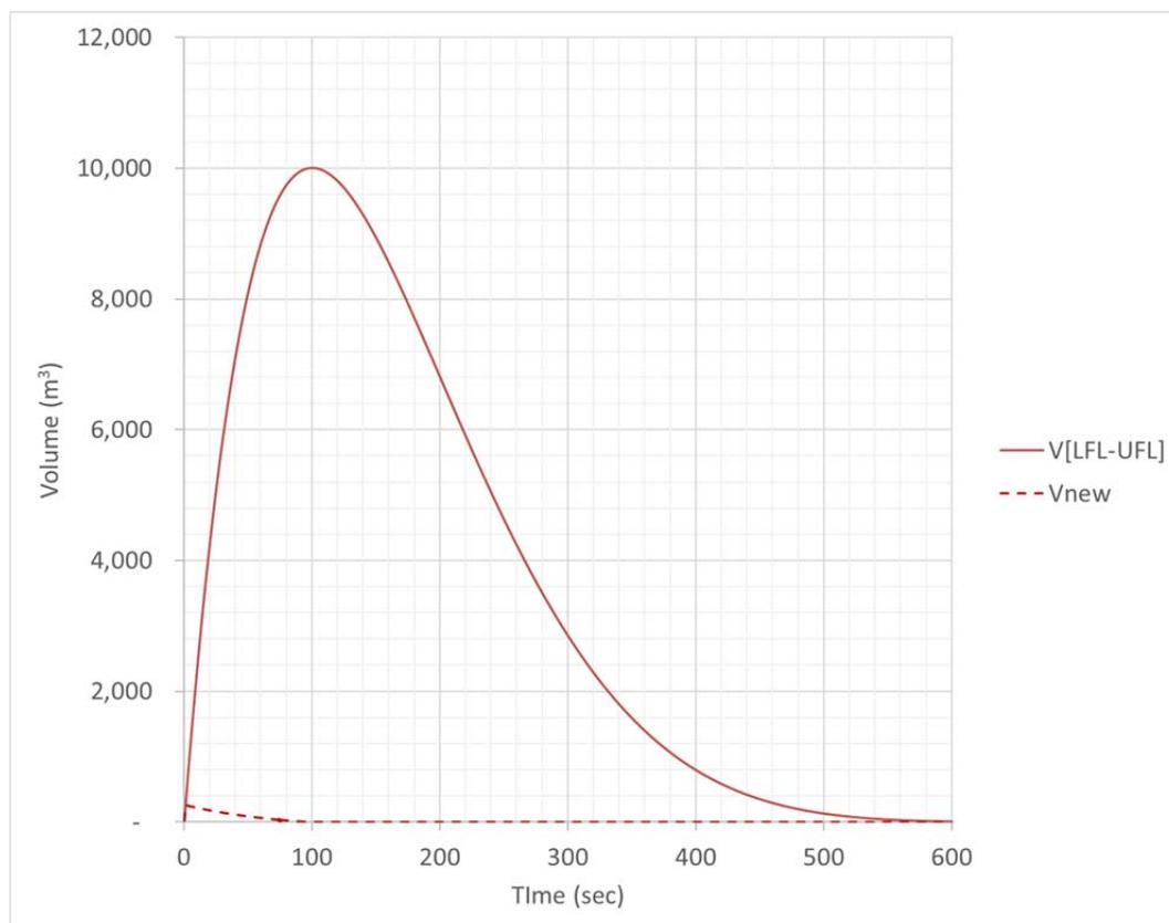
Figure 10.2 - Time dependent gas cloud parameters for a case example required to use an algorithm for uniform distribution of ignition sources in a given area
