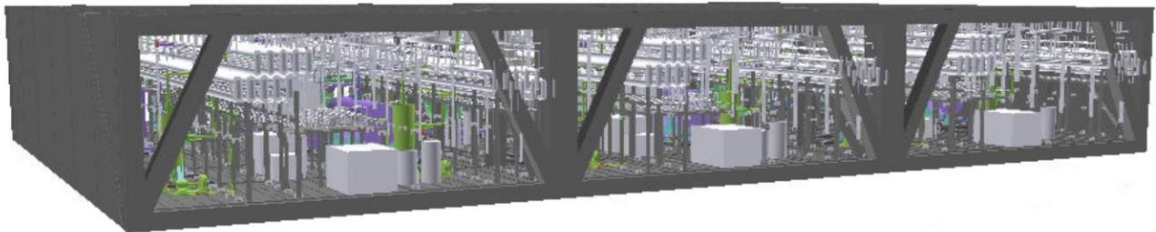
Figure 3-4: CM402EW; about 40 000 gross m<sup>3</sup>, two open walls
