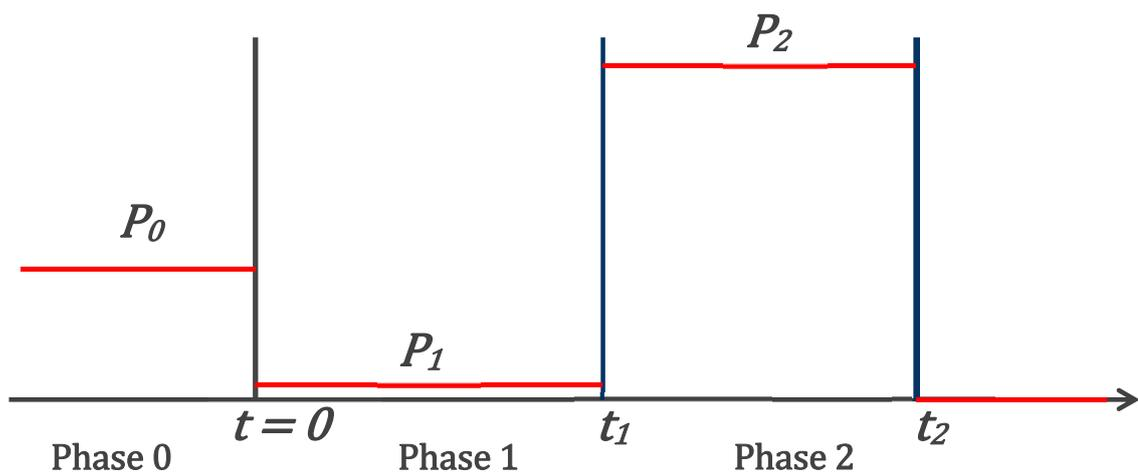
Figure 9.1 - The phases and parameters of the gas turbine ignition model
