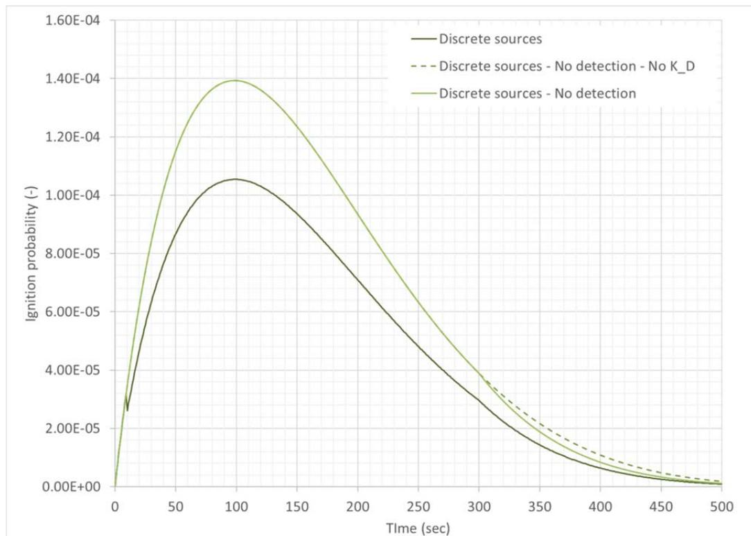
Figure 10.5 – Time dependent ignition probability calculated from equation (10.4) and using the total  $\lambda_{i,D}$  for all equipment categories found in Table 10.2. Note the effect of  $K_{D,300}$  more than 300 seconds after start of the leak. The time step used is 1 second. Note also the effect of detection and immediate isolation of discrete ignition sources at 10 seconds after start of the leak
