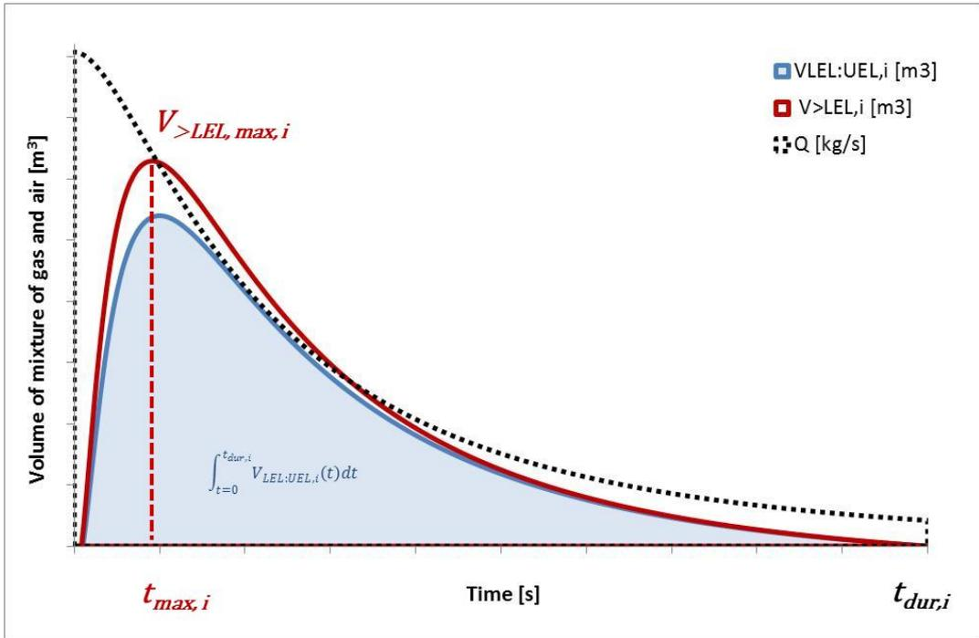
Figure 3.2 - Example time dependent gas cloud volume for a transient leak, denoted  $i$ , in a typical offshore process module
