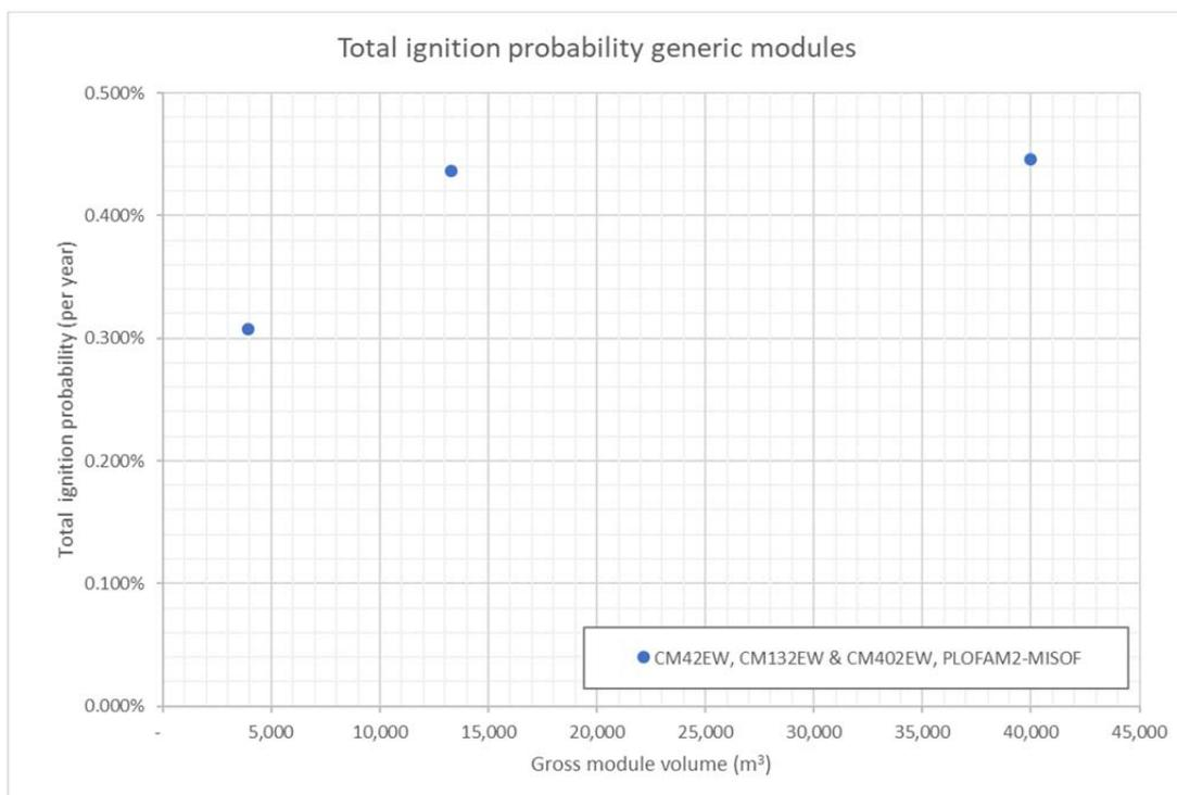
Figure 11.16 – Total ignition probability vs. module volume for the various modules
