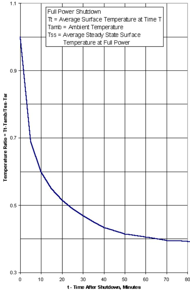
Figure 2.6 - Reduction of surface temperatures in LM2500 after shutdown. The cooling time in the figure is indicative. Probably, the cooling time is shorter for most components, but this has to be verified by vendor data
