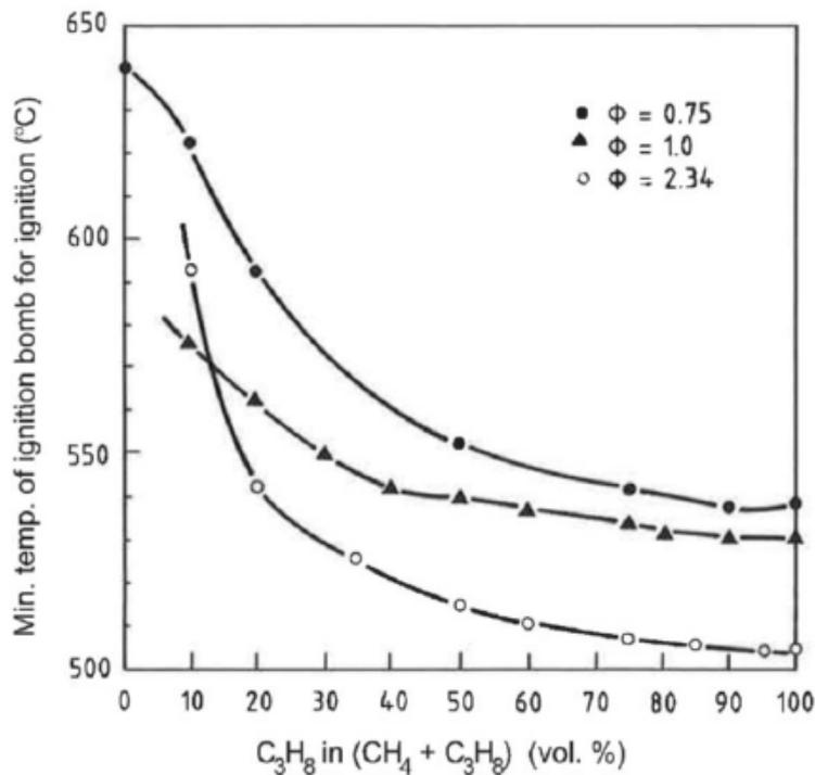
Figure 2.10 - Auto-ignition temperatures for mixtures of methane and propane, from Ref. /3/
