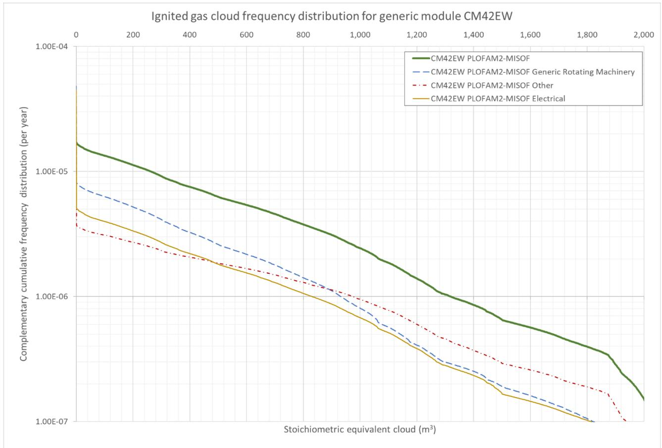
**Figure 4-16: CM42EW PLOFAM2-MISOF: Complementary cumulative frequency distribution for time of ignition of stoichiometric equivalent gas cloud.**
