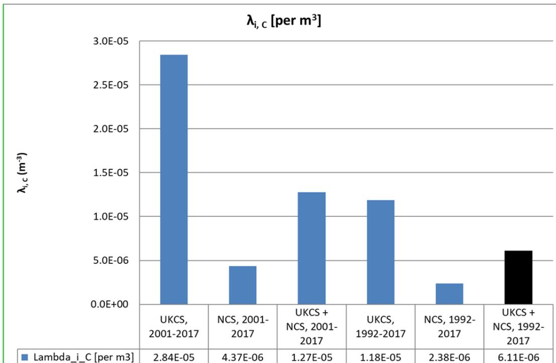
Figure 8.5 - Delayed ignition probabilities for continuous ignition sources. The concluded parameter to be used in the MISOF model is shown in black colour
