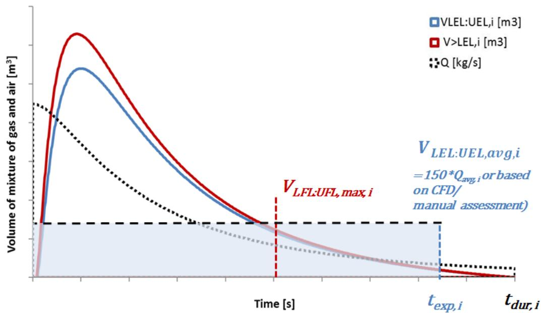
Figure 3.5 - Example c); time dependent gas cloud volume for a transient leak in a typical offshore process module and corresponding graphical representation of the estimation by generic gas exposure model. The example displays a case where the generic model underestimates the actual gas cloud parameters
