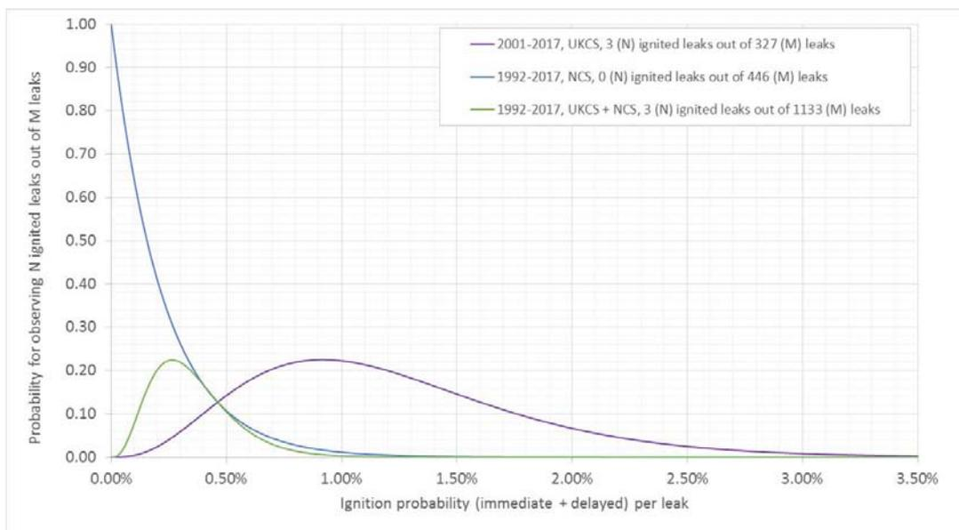
Figure 11.7 – The probability for observing N number of observed ignited leaks out of M total leaks as function of  $p$  (estimate of the underlying ignition probability due to immediate and delayed ignition) based on the binomial distribution. The results are shown for the base dataset (UKCS and NCS for the period 1992-2017) and for two extreme subsets in terms of number of leaks per ignited leak
