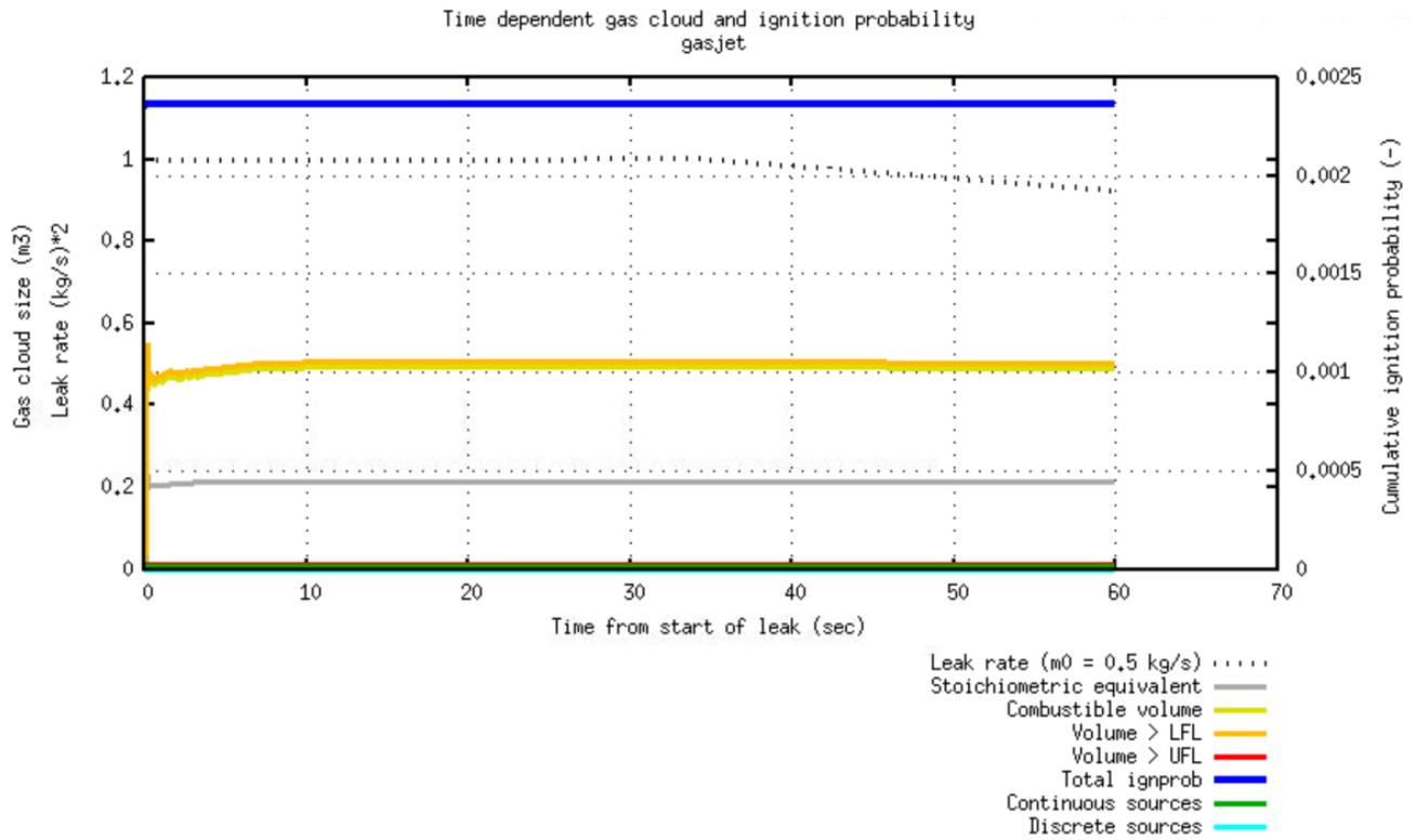
Figure 3-10: Transient result for 0.5 kg/s gas leak in CM42EW.
