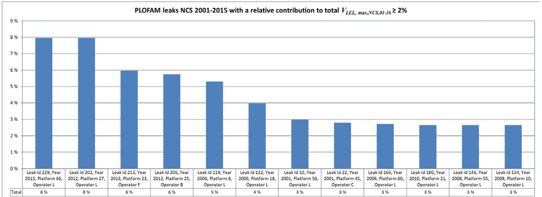
Figure 3.7 - Major contributors to  $V_{LFL:UFL,max,NCS,01-16}$ . In total, these leaks constitute about 60% of  $V_{LFL:UFL,max,NCS,01-16} \cdot t_{exp}$
