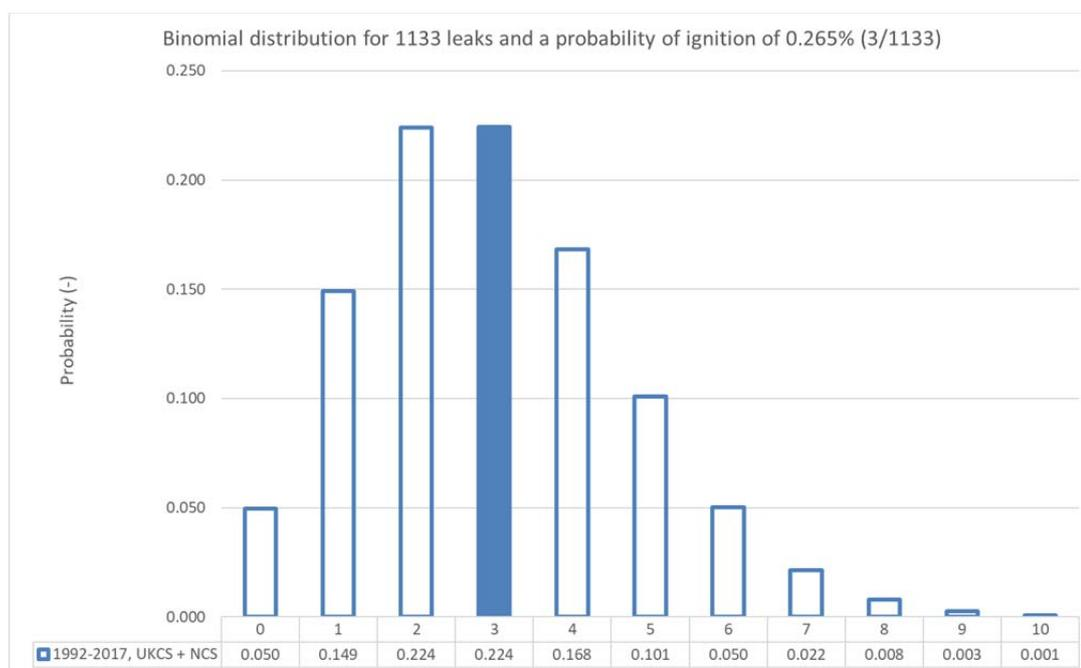
Figure 7.2 – Binomial distribution for 3 ignited leaks in hazardous area out of 1133 leaks occurring at installations located on UKCS and NCS in the period 1992 -2017 (see Table 7.3)
