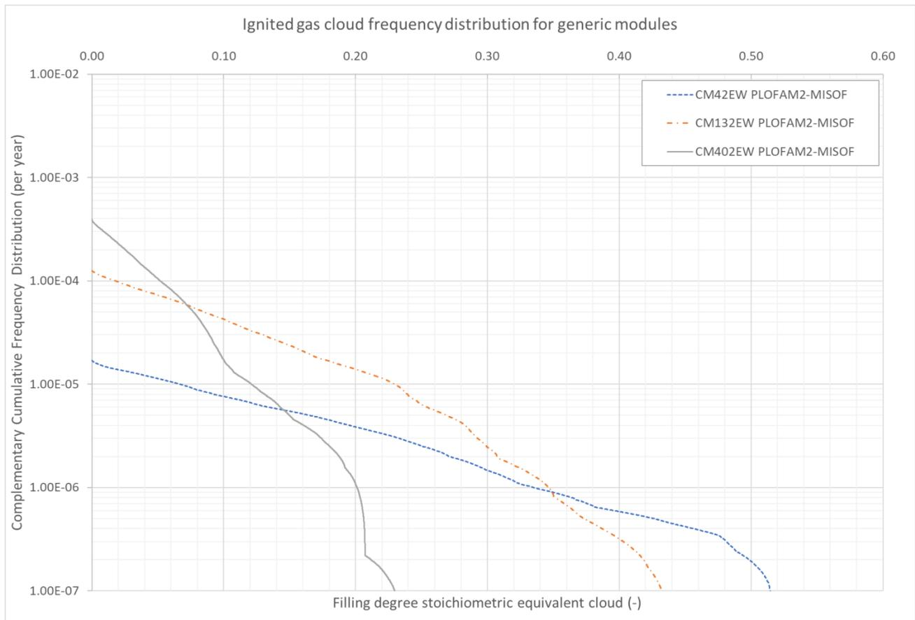
**Figure 4-26: PLOFAM-MISOF: Complementary cumulative frequency distribution for filling degree of ignited stoichiometric equivalent gas cloud for the different generic modules.**
