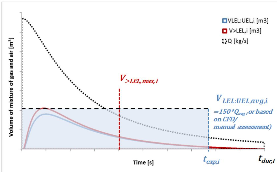
Figure 3.4 - Example b); time dependent gas cloud volume for a transient leak in a typical offshore process module and corresponding graphical representation of the estimation by generic gas exposure model. The example displays a case where the generic model overestimates the actual gas cloud parameters
