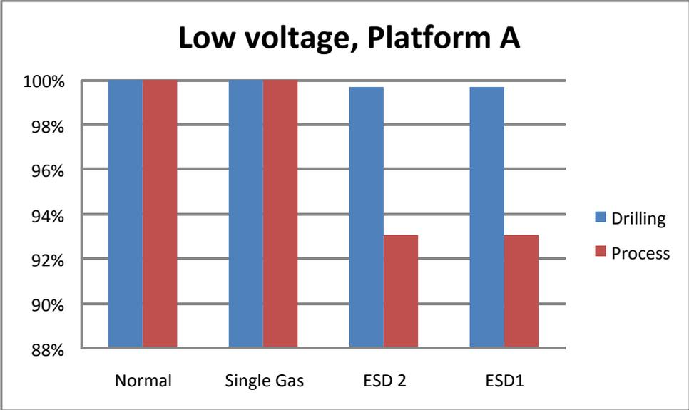
Figure A 3: Illustration of low voltage shutdown at Platform A
