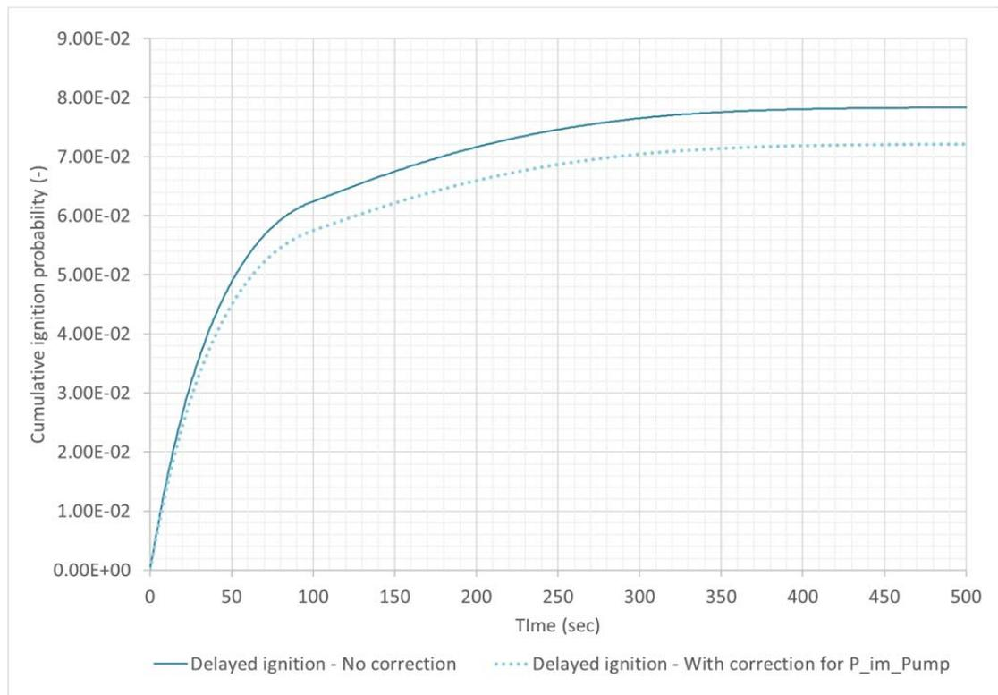
Figure 10.6 – Cumulative time dependent delayed ignition probability assuming that the leak is stemming from a pump (immediate ignition probability is 7.9%). The different curves display the effect of the term  $(1 - \sum_{i=1}^N P_{T,i-1}(I))$  in equation (10.6) assuming that the only contributions are  $\lambda_{i,C}$ ,  $\lambda_{i,D}$  and  $P_{im,pump}$ . The time step,  $\Delta t$ , used was 1 second
