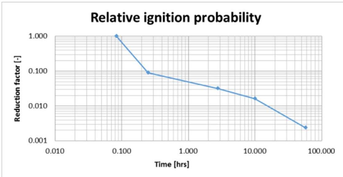
Figure 8.11 - Relative ignition probability per time unit of exposure over time for blowouts
