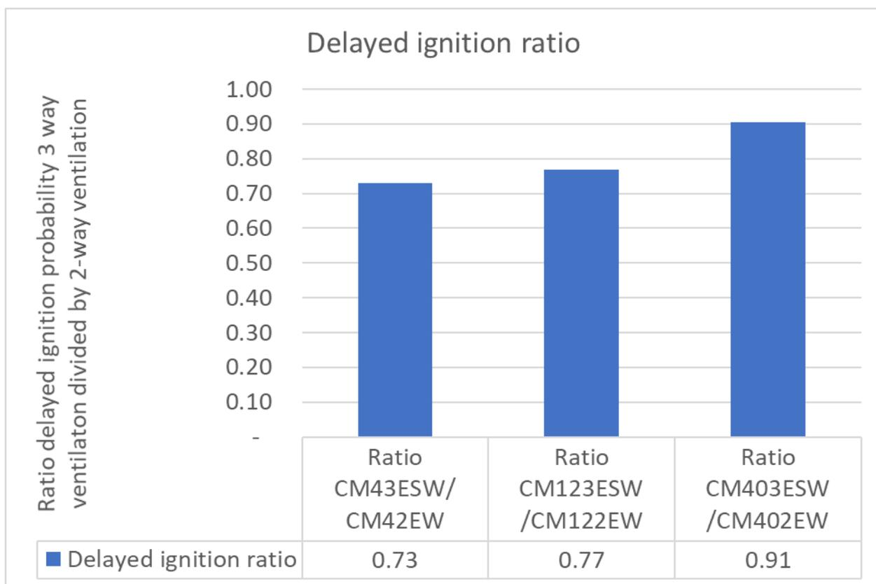
Figure 4-27: Ratio delayed ignition probability for initial sensitivity study of effect of global ventilation conditions.
