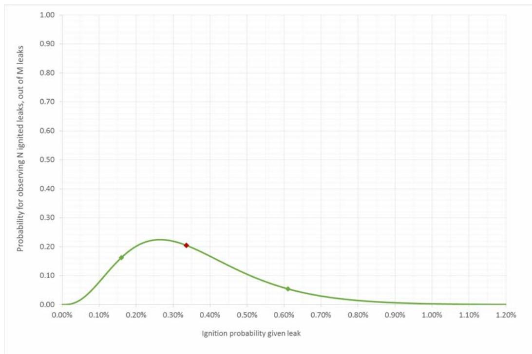
Figure 11.3 – The probability for observing the number of observed ignited leaks (3) out of 1,133 leaks as function of  $p$  (estimate of the underlying ignition probability due to immediate and delayed ignition) based on the binomial distribution. The ignition probabilities corresponding to a probability of 90%, 50% and 10% for observing 3, or fewer, ignited leaks are marked with tile type marker
