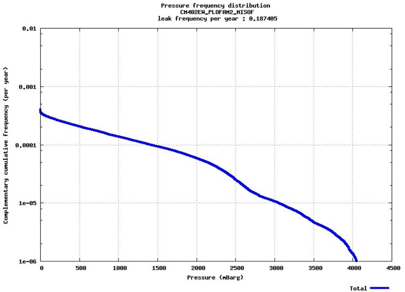
Figure 5-3: CM402EW PLOFAM-MISOF: Complementary cumulative frequency distribution for dimensioning explosion load
