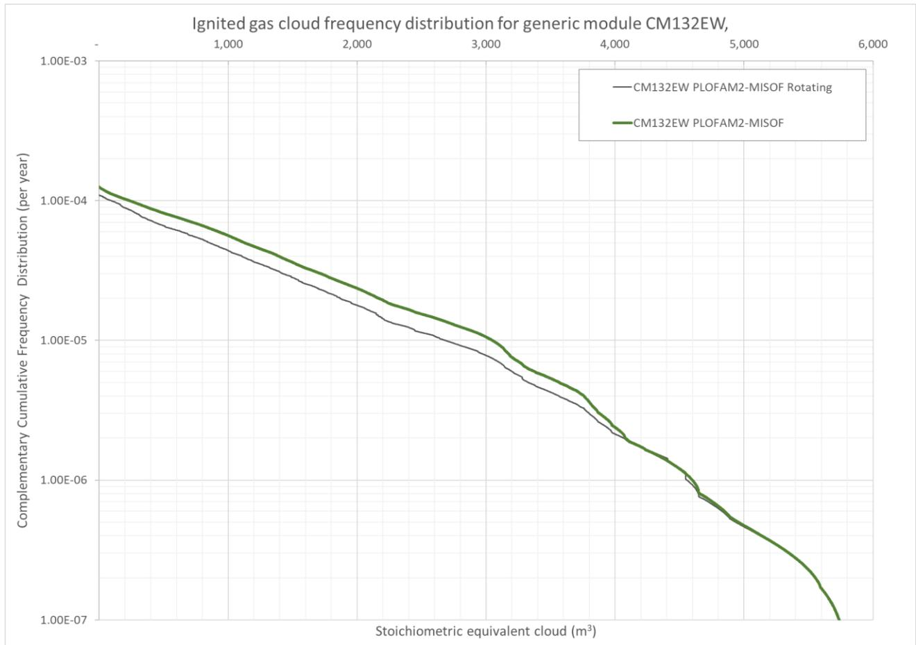
**Figure 4-20: CM132EW PLOFAM2-MISOF with specific modelling of 12 pumps instead of generic volumetric modelling of rotating machinery; complementary cumulative frequency distribution for time of ignition of stoichiometric equivalent gas cloud.**
