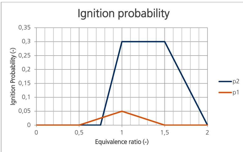
Figure 2.12 – How concentration dependency for the ignition probabilities  $p_i$  and  $p_j$  could be taken into account
