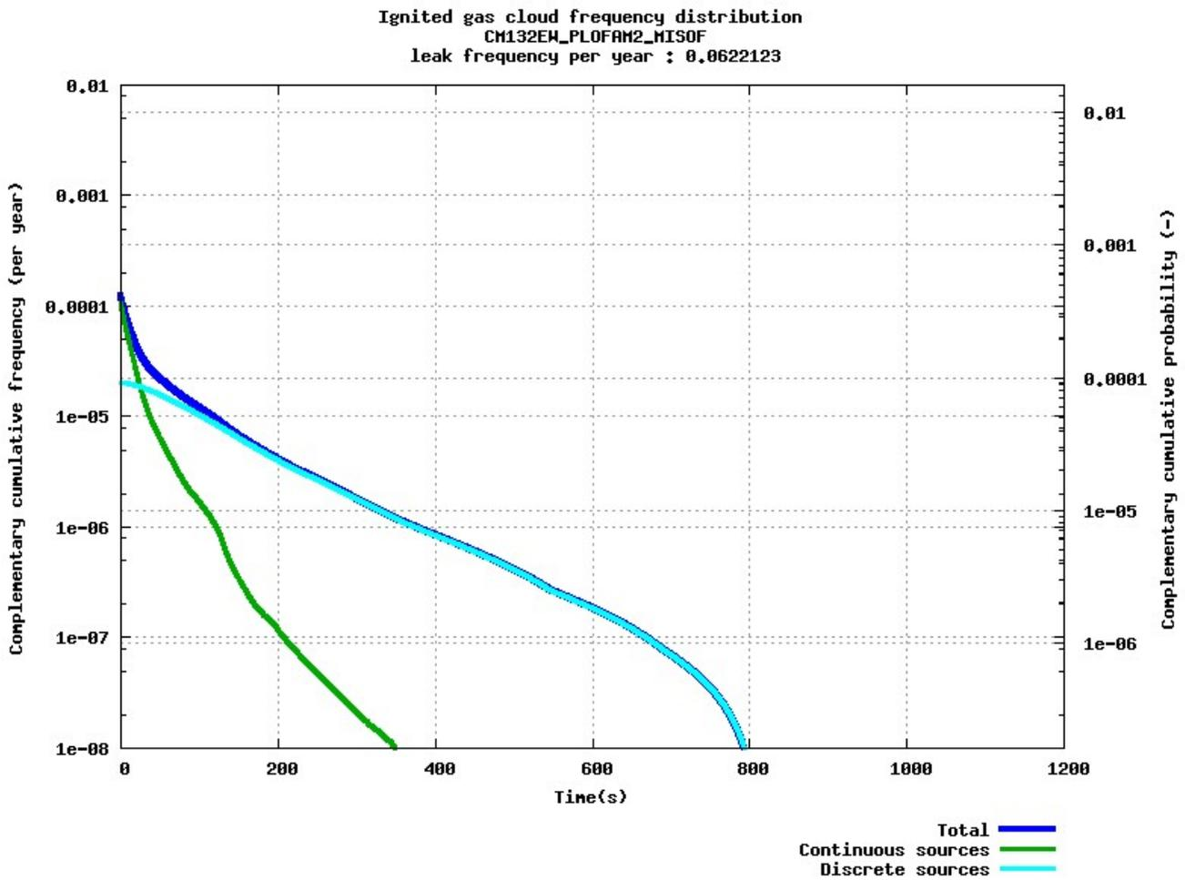
Figure 4-14: CM132EW PLOFAM-MISOF: Complementary cumulative frequency distribution for time of ignition of stoichiometric equivalent gas cloud.
