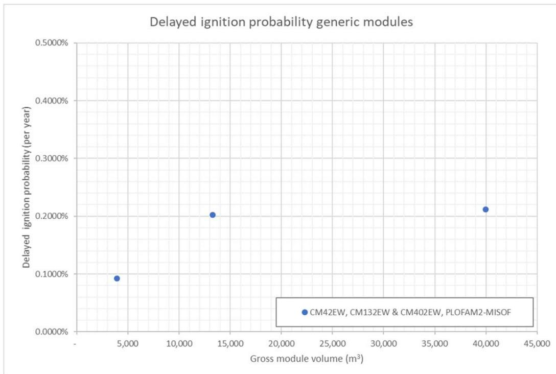
Figure 11.17 – Delayed ignition probability vs. module volume for the various modules
