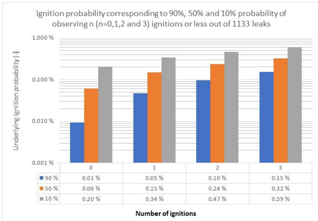
Figure 11.5 – Underlying ignition probability corresponding to 90%, 50% and 10% probability of observing  $n$  ( $n=0, 1, 2$  and  $3$ ) ignitions or less out of 1133 leaks
