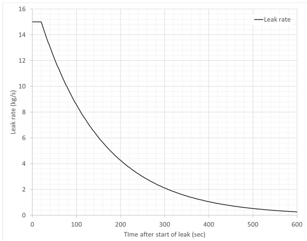
Figure 10.1 - Time dependent leak rate used as basis for an example to illustrate use of algorithm for uniform distribution of ignition sources in area
