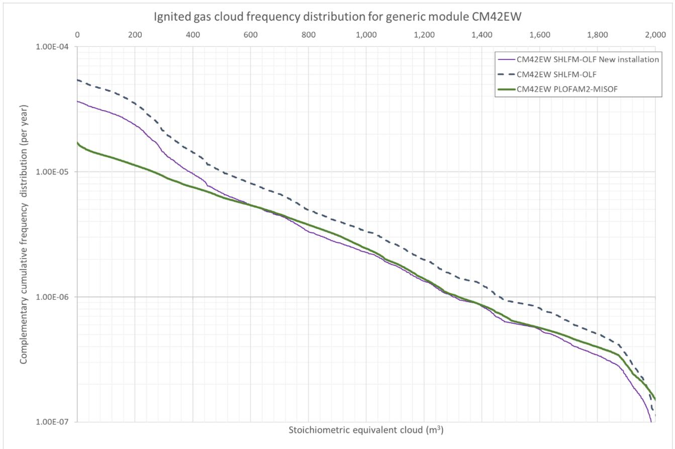
**Figure 4-7: Complementary cumulative frequency distribution for ignited stoichiometric equivalent gas cloud for the generic module CM42EW including sensitivity with OLF model assuming new installation. A correction factor of 0.675 has been used to reflect a new installation (see Table 3-6).**
