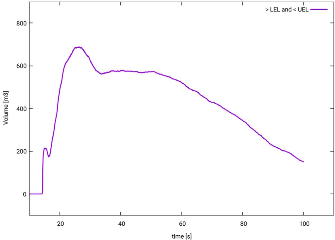
Figure 3.11 - Leak ID 154: Time history for the combustible volume of gas,  $V_{LFL:UFL,154}(t)$ , estimated by CFD simulation performed with Kamelon FireEx KFX®
