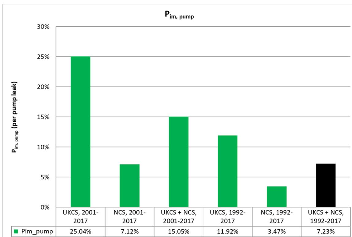
Figure 8.3 - Immediate ignition probability for pump leaks. The concluded parameter to be used in the MISOF model is shown in black colour
