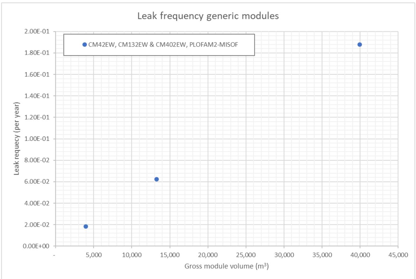
Figure 6-1: Total leak frequency vs. module volume for the various modules
