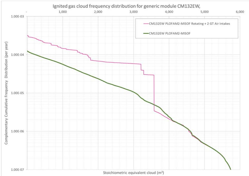
Figure 11.14 – CM132EW PLOFAM-MISOF with specific modelling of 12 pumps instead of generic volumetric modelling of rotating machinery + two gas turbine air intakes located directly above the module (see Figure 11.15); complementary cumulative frequency distribution for time of ignition of stoichiometric equivalent gas cloud
