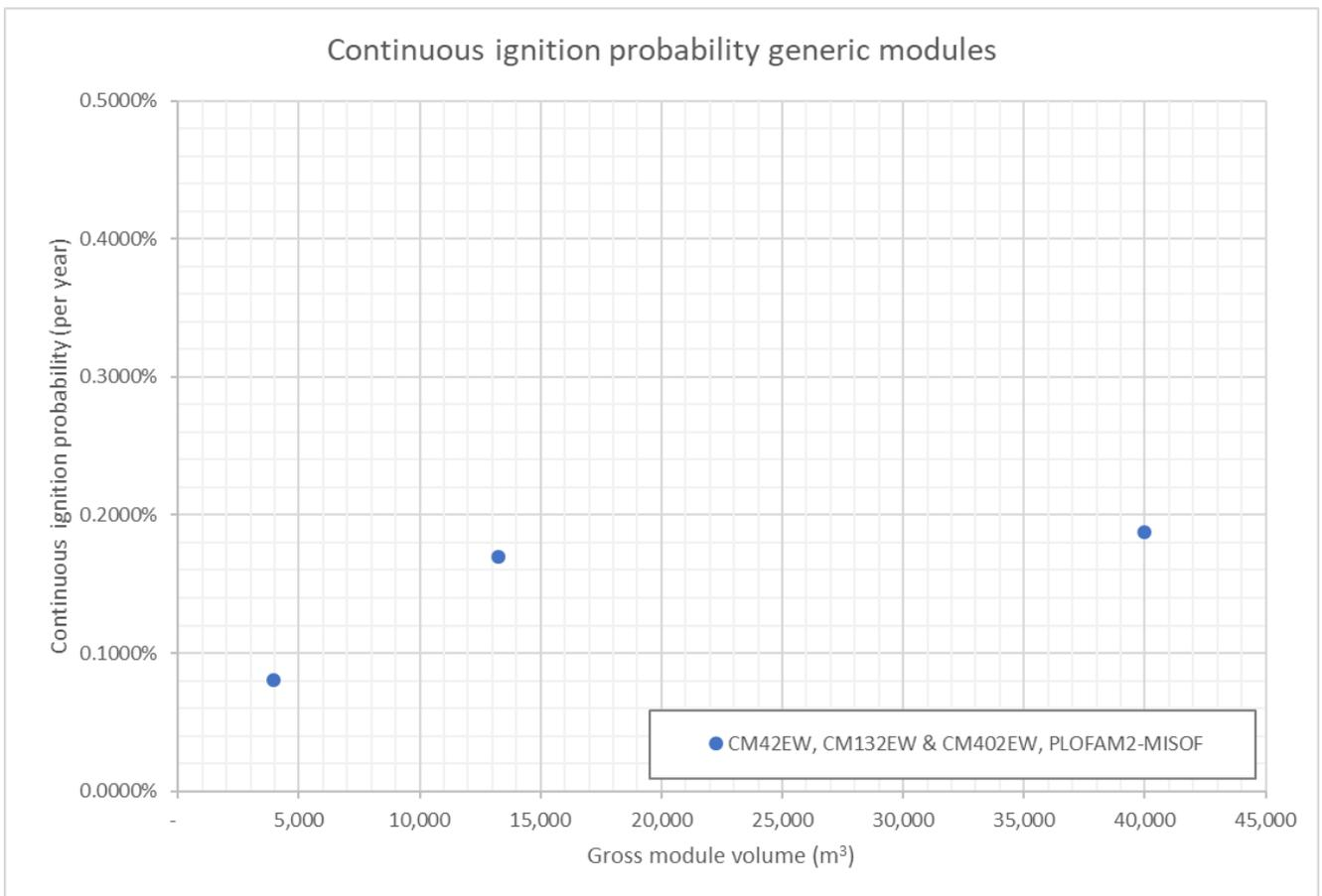
**Figure 6-5: Continuous ignition probability vs. module volume for the various modules**
