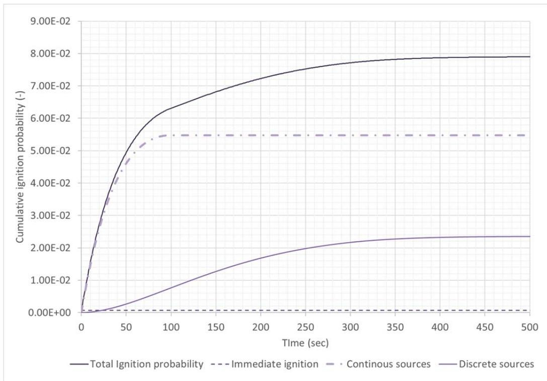
Figure 10.7 – Total cumulative time dependent ignition probability for all equipment categories and for all ignition mechanisms (using the generic probability for immediate ignition; i.e. 0.07%)
