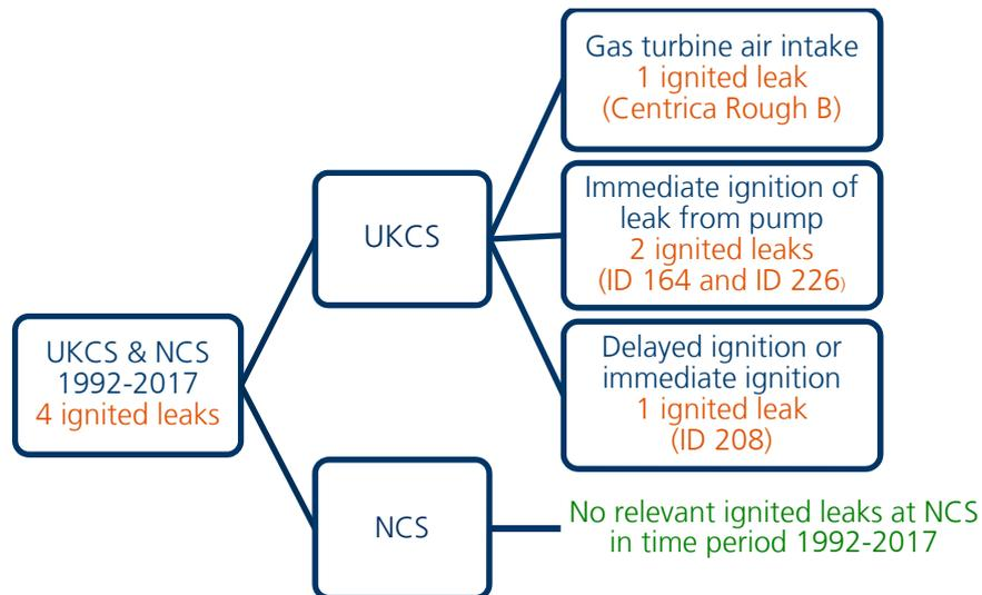
Figure 8.1 - Overview observed ignited leaks in the period 1992-2017 at UKCS& NCS relevant for modelling of ignition probability in QRA (*i.e.* corresponding to PLOFAM leaks)
