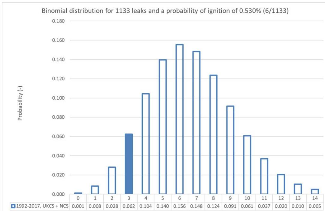
Figure 7.3 – Binomial distribution for 1133 leaks assuming ignition probability of 0.55% (6/1133)
