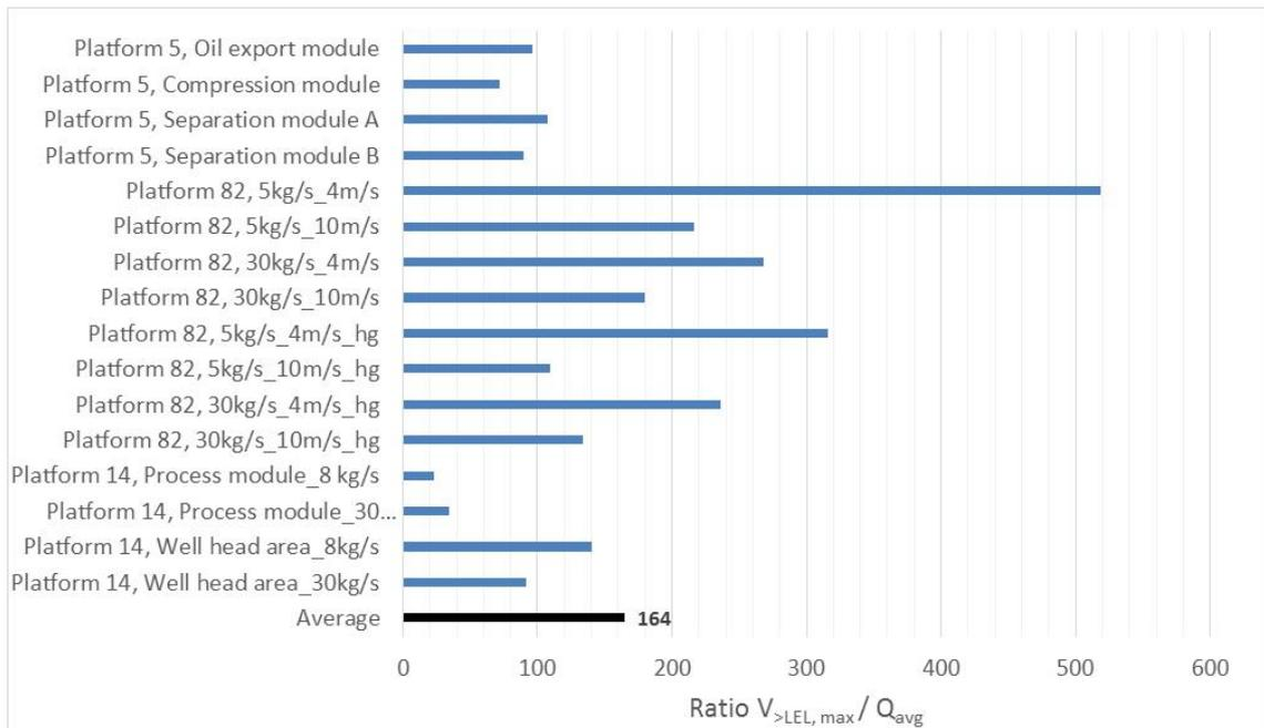
Figure 3.1 - Average ratio  $V_{>LEL,max,i}/Q_{avg}$  for all CFD simulations performed in 4 different typical offshore modules (anonymization in accordance with nomenclature in PLOFAM, see Ref. /1/ in main report)
