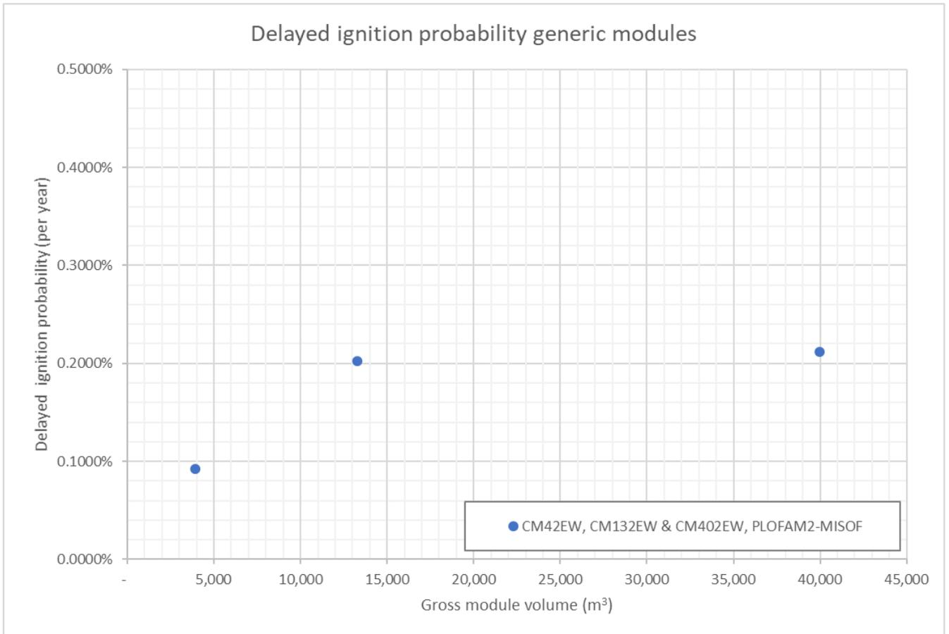
**Figure 6-4: Delayed ignition probability vs. module volume for the various modules**
