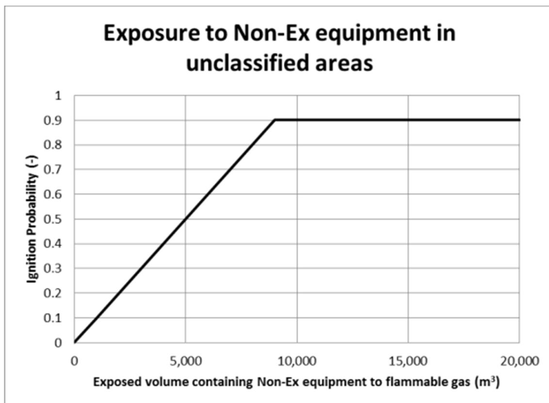
Figure 9.2 - Exposure to non-Ex equipment in unclassified areas. This is applicable to areas where non-Ex equipment is generally used. For specific non-Ex equipment, (believed to be the regular case in the North Sea) a special study defining the conditional ignition probability associated with the equipment is recommended
