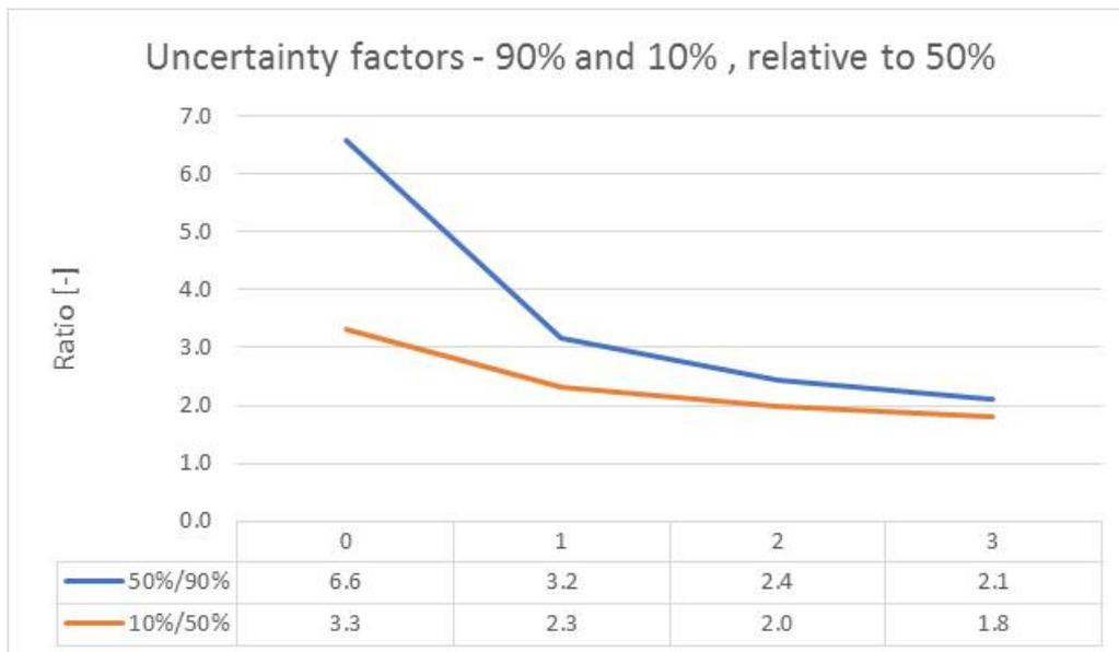
Figure 11.6 – Underlying ignition probability corresponding to 50% relative to 90% probability of observing n or fewer ignitions out of 1133 leaks, and the underlying ignition probability corresponding to 10% relative to 50% probability of observing n or fewer ignitions out of 1133 leaks
