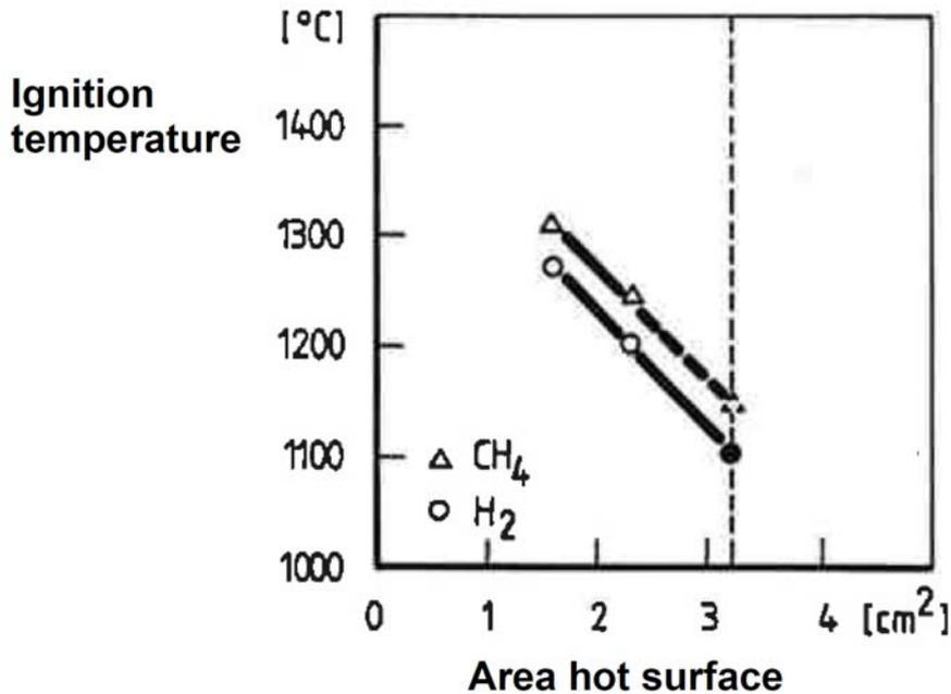
**Figure 1** Ignition temperature of methane- and hydrogen-air mixtures depending on the surface area of the hot surface [19].
