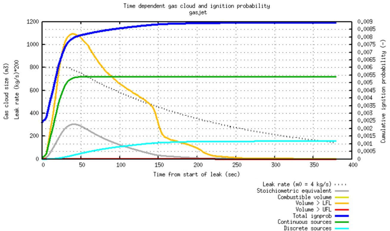
Figure 3-11: Transient result for 4 kg/s gas leak in M43OSV
