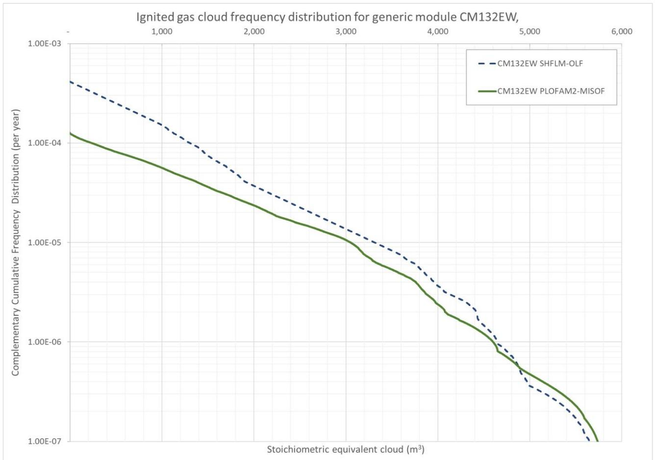
**Figure 4-2: Complementary cumulative frequency distribution for ignited stoichiometric equivalent gas cloud for the generic module CM132EW.**
