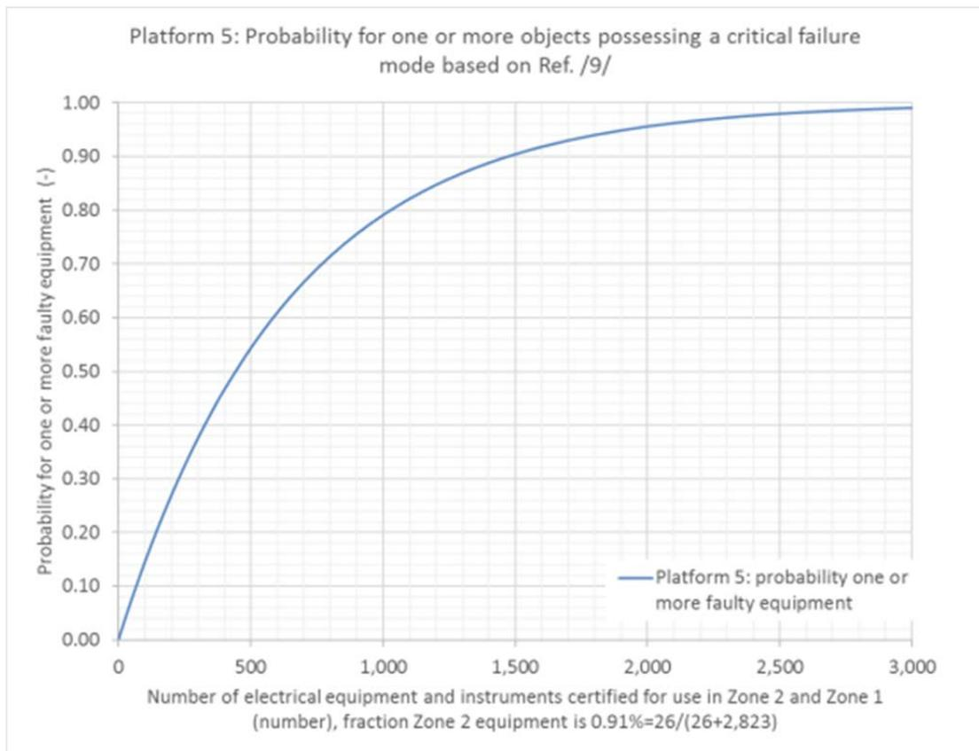
Figure 8.8 - Probability of one or more faulty Zone 2 or Zone 1 equipment for increasing number of electrical equipment for Platform 5. The fraction of Zone 2 equipment is  $26/(26 + 2823)$  in accordance with Table 8.13
