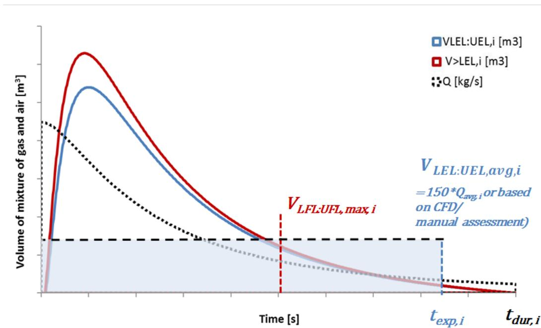
Figure 3.5 - Example c); time dependent gas cloud volume for a transient leak in a typical offshore process module and corresponding graphical representation of the estimation by generic gas exposure model. The example displays a case where the generic model underestimates the actual gas cloud parameters
