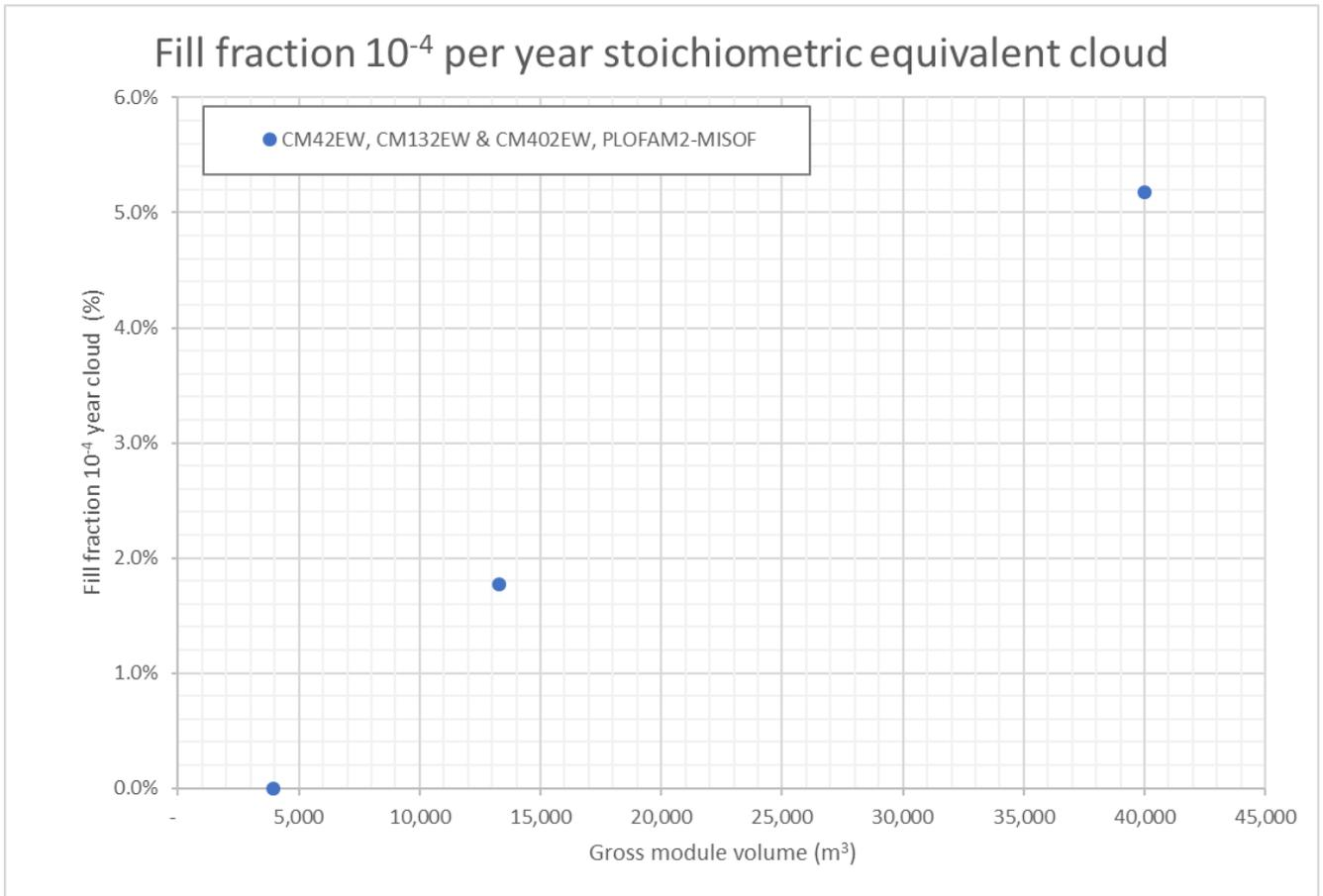
**Figure 6-7: Fill fraction 10<sup>-4</sup> per year stoichiometric equivalent volume vs. module volume for the three modules**
