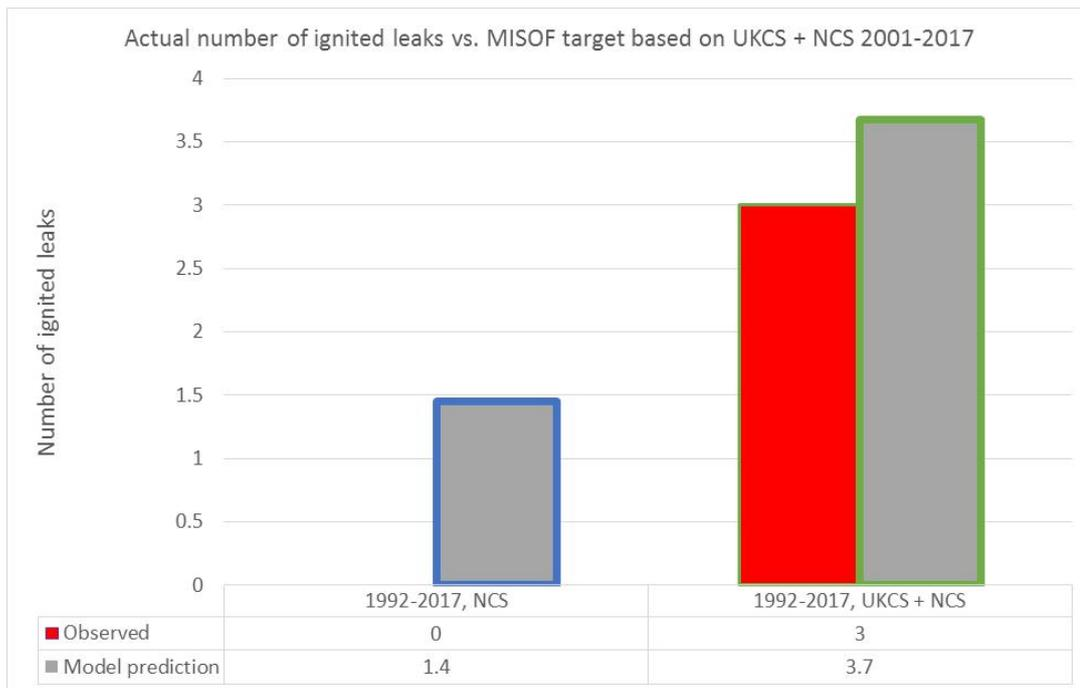
Figure 11.9 – Ignition in hazardous areas: comparison of observed number of ignited leaks vs. MISOF model prediction for the various data subsets
