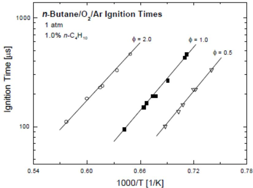
Figure 2.8 - Effect of stoichiometry on ignition delay time for butane, from Ref. /5/
