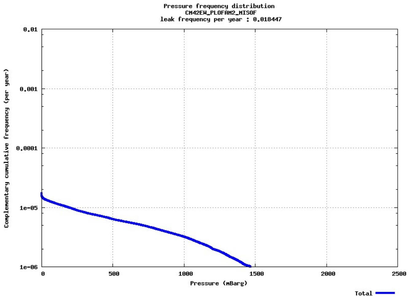
Figure 5-1: CM42EW PLOFAM-MISOF: Complementary cumulative frequency distribution for dimensioning explosion load
