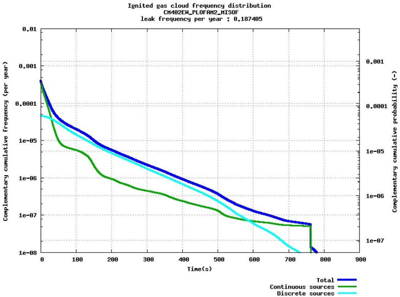
Figure 4-15: CM402EW PLOFAM-MISOF: Complementary cumulative frequency distribution for time of ignition of stoichiometric equivalent gas cloud.
