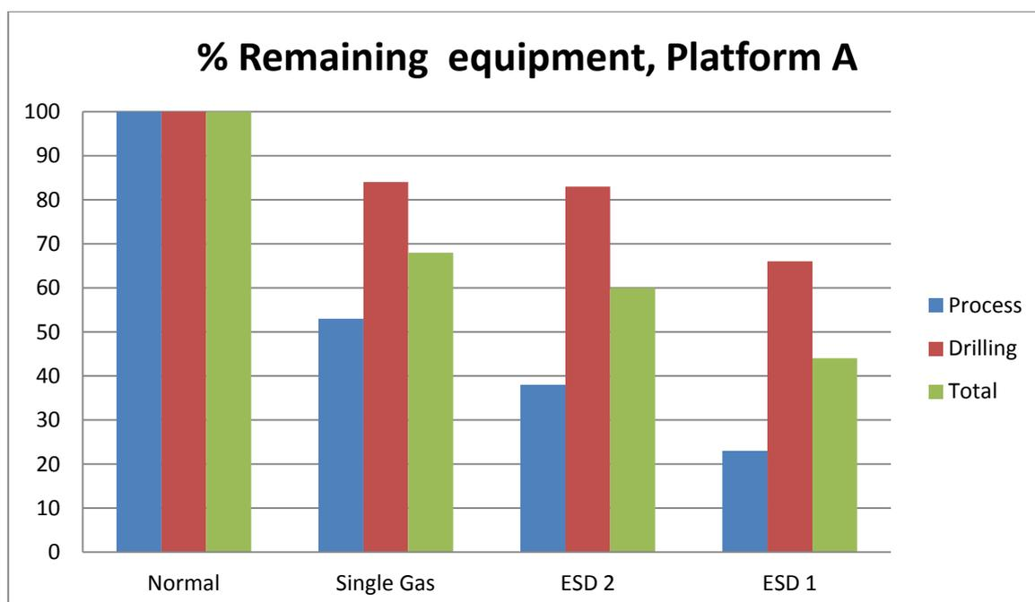
Figure 5.1: Isolation factor F for equipment on Platform A, scaled for Ex protection.
