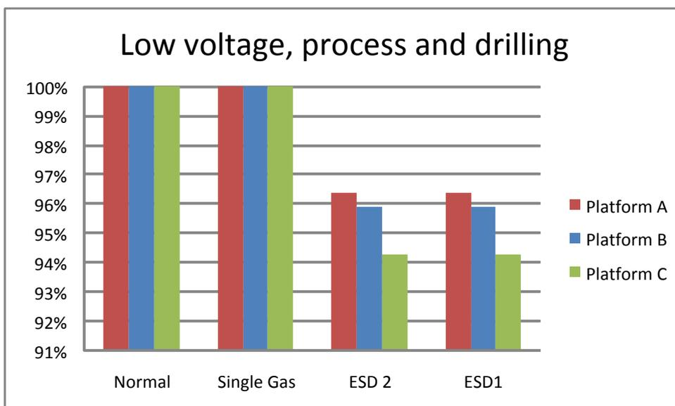
Figure A 12: Illustration of shutdown of low voltage ignition sources without scale factor for all three installations
