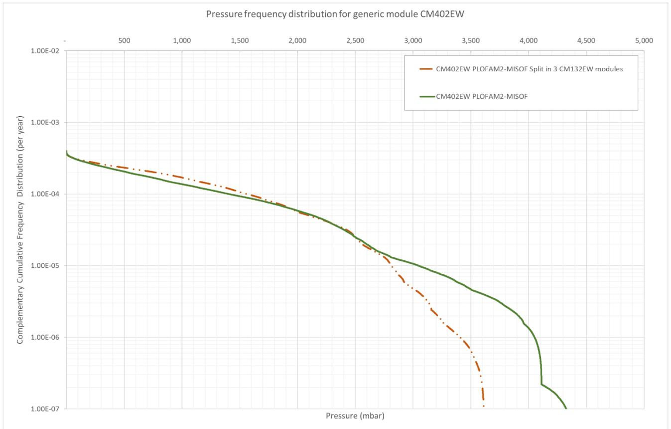
**Figure 5-5: CM402EW PLOFAM2-MISOF: Complementary cumulative frequency distribution for dimensioning explosion load. Sensitivity case representing a design where the CM402EW module is split into three identical CM132EW modules. The aggregated pressure frequency distribution for all three modules established by combining the estimated cloud distribution shown in Figure 5-4 with the explosion model for CM402EW (see Figure 3-9).**
