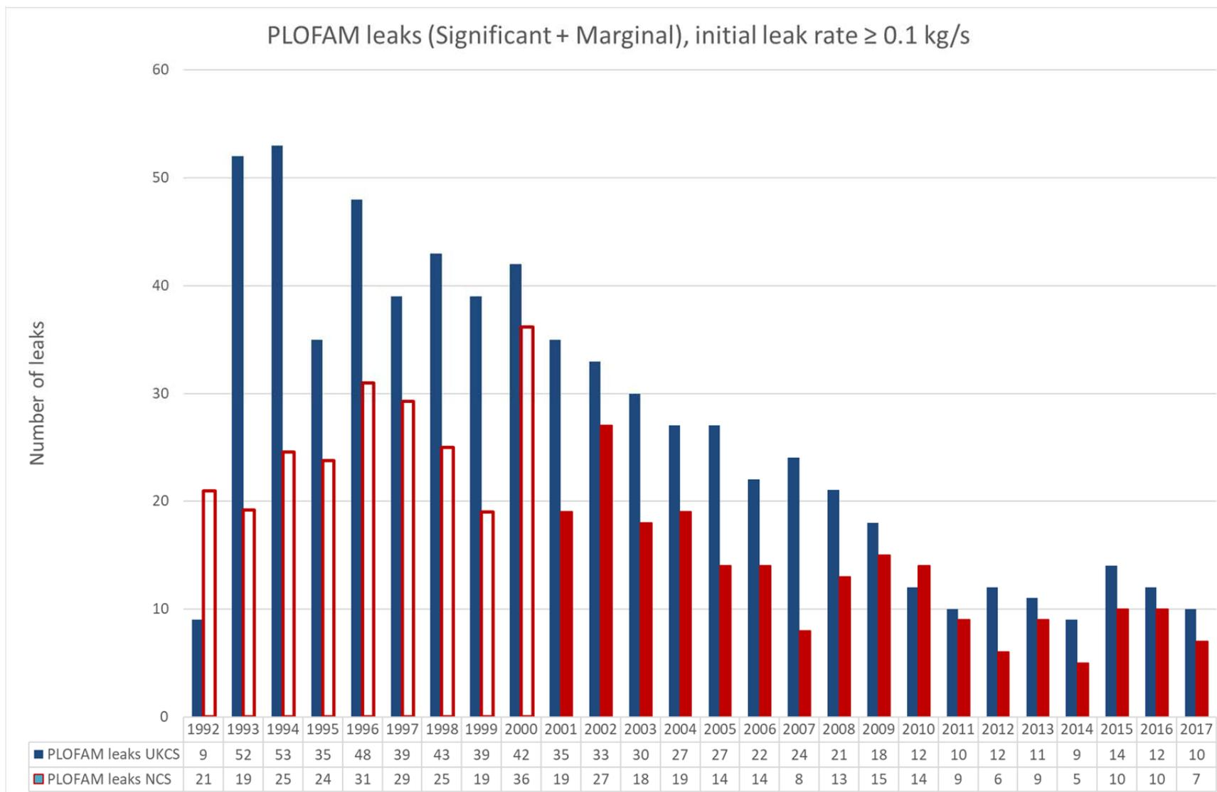
Figure 7.5 – Number of PLOFAM leaks per year for the period 1992 and onwards. The data for installations on the NCS before 2001 is estimated based on various data sources, and there is some uncertainty associated with these data. The data for this period is therefore marked with unfilled bars
